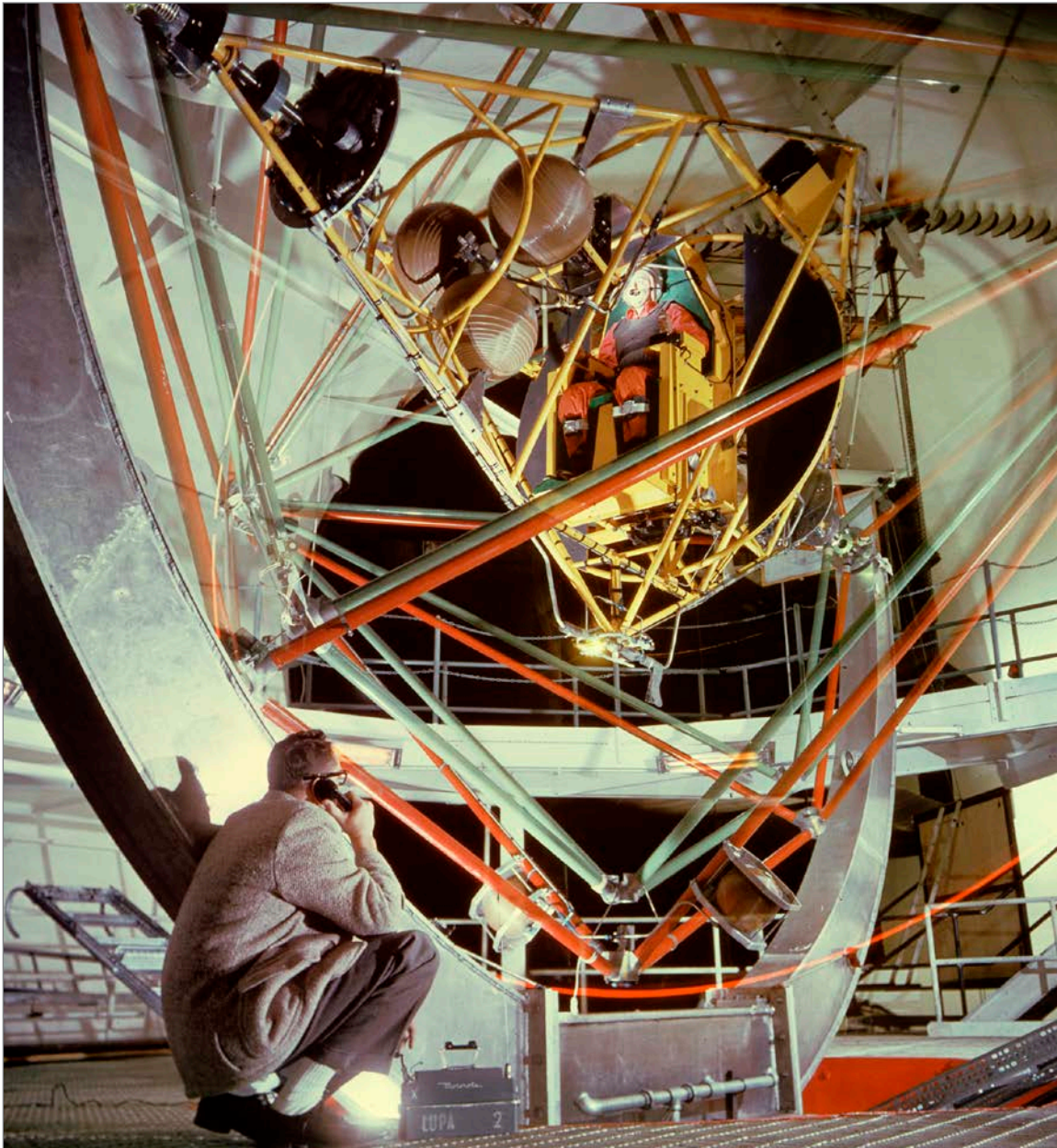
The Multiple Axis Space Test Inertia Facility (MASTIF), also known as the Gimbal Rig, is shown here in the Altitude Wind Tunnel (AWT) at Lewis Research Center, now John H. Glenn Research Center at Lewis Field.
