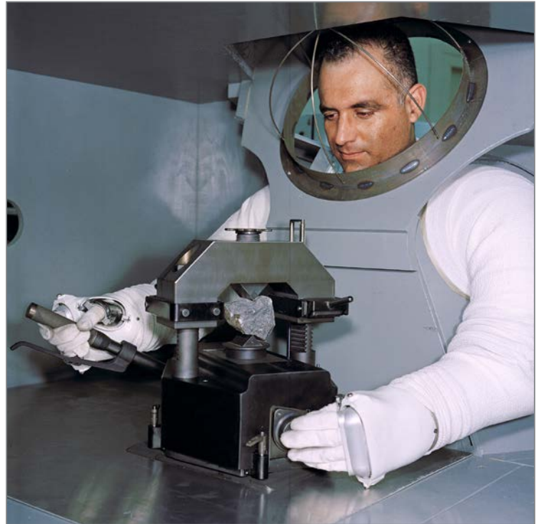
JPL developed a prototype rock-breaker/can-sealer to handle lunar rocks.
