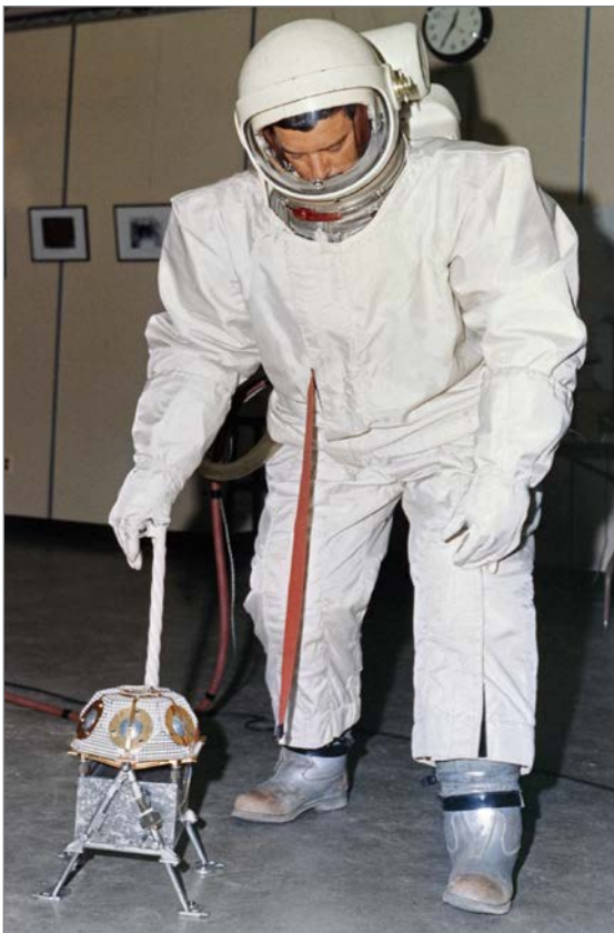
In this 1967 photo, an astronaut practiced removing the Solar Wind Spectrometer from its container and deploying it.
