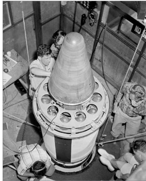
Shown here is the Missile 34 high-speed stages and experimental reentry vehicle, 24 May 1957. (Copyright California Institute of Technology)
