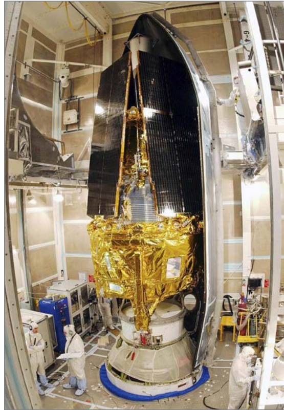
Shown here is the installation of the Gravity Probe B (GP-B) payload atop the Delta II launch vehicle. (Photo credit: Russ Underwood/Lockheed Martin Corporation)
