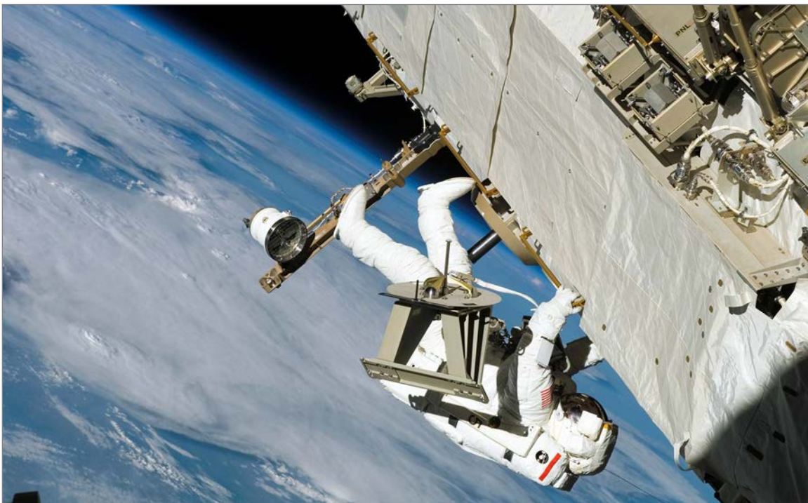
Piers J. Sellers, STS-112 mission specialist, works on the Starboard One (S1) Truss, newly installed on the ISS.
