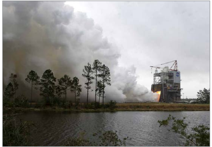
NASA engineers conduct a successful test firing of RS-25 rocket engine No. 2059 on the A-1 Test Stand at Stennis. The hot fire marks the first test of an RS-25 flight engine for NASA's new Space Launch System (SLS) vehicle. Four RS-25 engines, in conjunction with a pair of solid rocket boosters, will power the SLS at launch. The March 10 test was conducted for a full-duration 500 seconds, the same amount of time the engines must fire during an actual launch.
