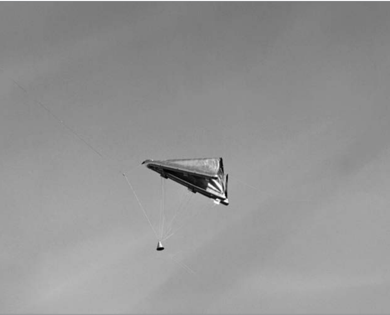
A Gemini model with a flexible wing attached is shown during a drop model test at Plum Tree Island, Virginia. (Photo credit: NASA)
