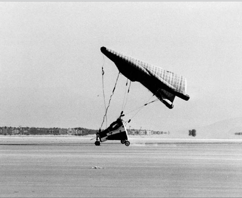
If the Rogallo inflatable wing had been used for Gemini landings, it would have looked like this test except with skids instead of wheels. (Photograph credit: North American Aviation and NASA)
