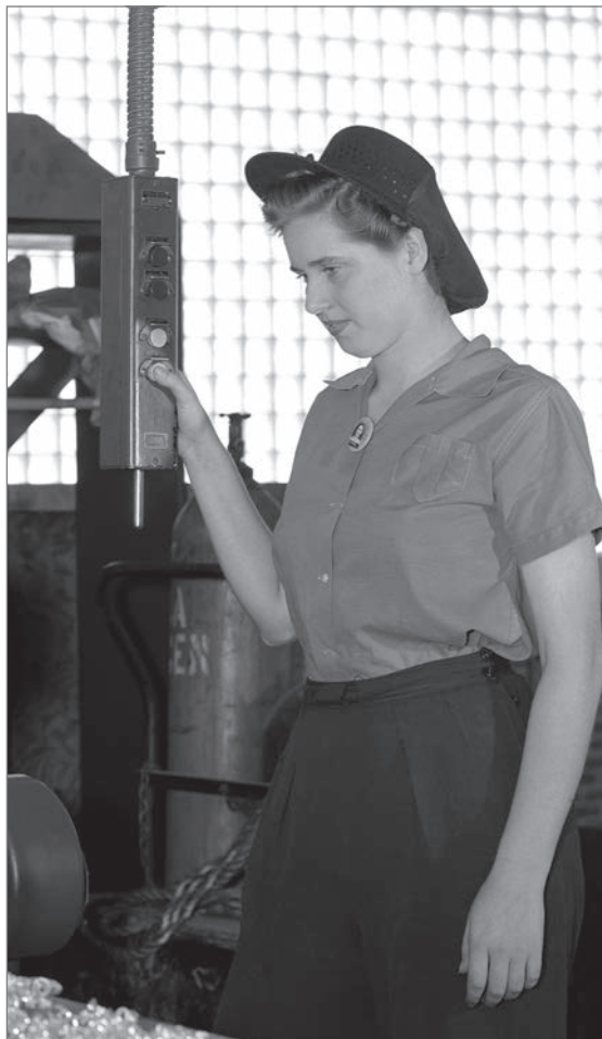
This woman is wearing a safety cap with snood. Note that the cap is pushed back on her head and not worn as prescribed. (L-33962)
