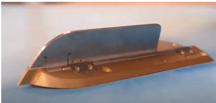
Image 3: A close-up image of a vortex generator
