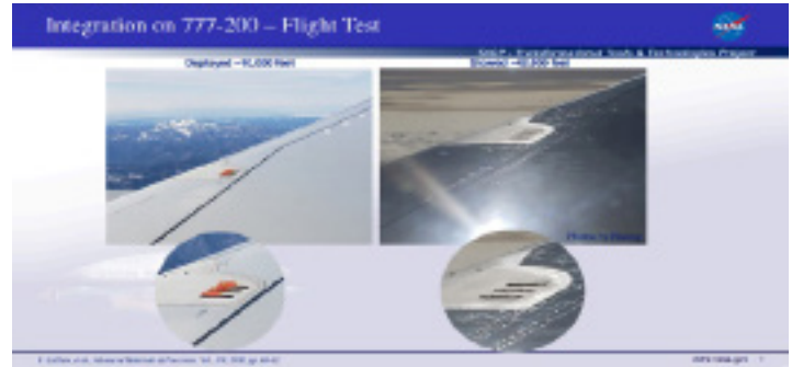
Image 4: Vortex generators on the ecoDemonstrator in the extended and collapsed positions
