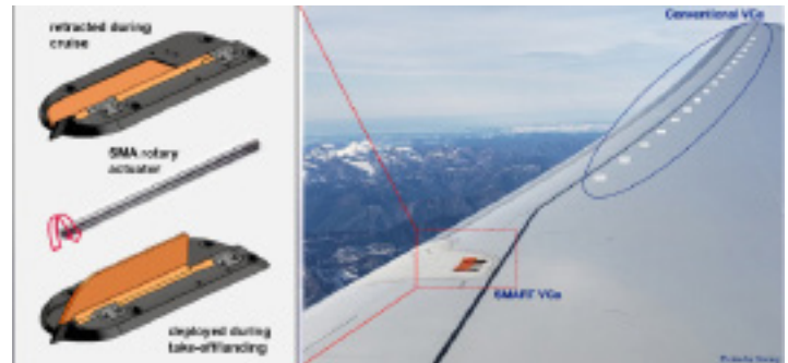
Image 5: explanation of how the smart memory alloy will work on a vortex generator
