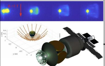
Rendering of pulsed fusion propulsion vehicle with PGMN, model of plasma expansion in PGMN, and experimental data of plasma retardation and expansion in strong magnetic field.
