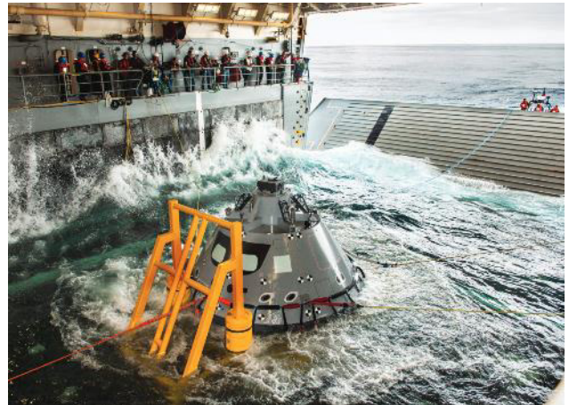
A test version of the Orion capsule is pulled into the flooded well deck of the USS John P. Murtha. (NASA/Tony Gray)
