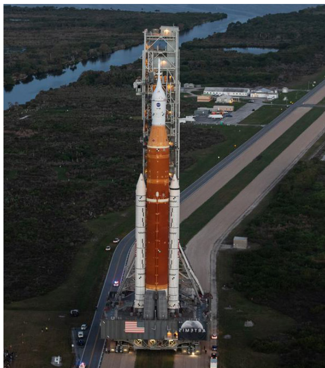
NASA's crawler-transporter carries the Space Launch System rocket with the Orion spacecraft to the launch pad. (NASA/Joel Kowsky)
