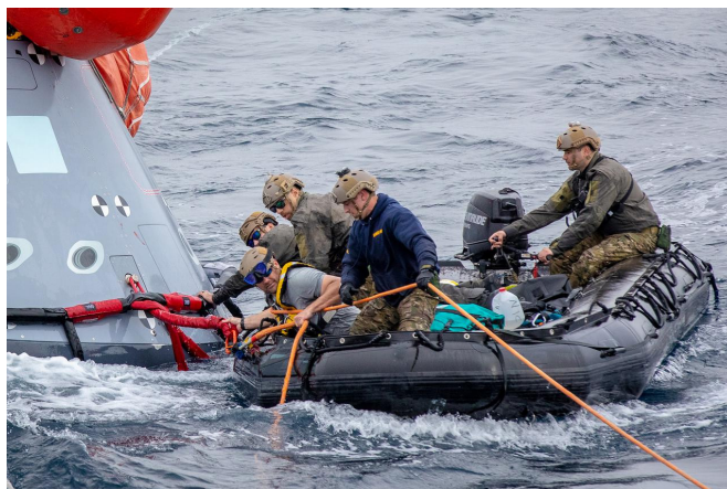
Navy divers attach lines to a mock Orion capsule during a recovery test. (NASA/Frank Michaux)
