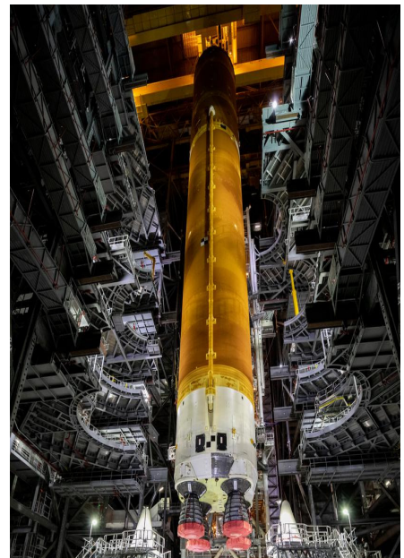
NASA teams prepare to lower the Space Launch System core stage inside the Vehicle Assembly Building at NASA's Kennedy Space Center. (NASA/Cory Huston)
