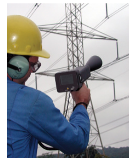
UE Systems Inc. detectors use licensed NASA technology to safely scan for electrical and compressed air leaks.
