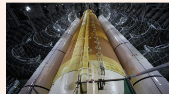
Closeup view of the SLS rocket inside the Vehicle Assembly Building with platforms retracted. (NASA/Frank Michaux)
