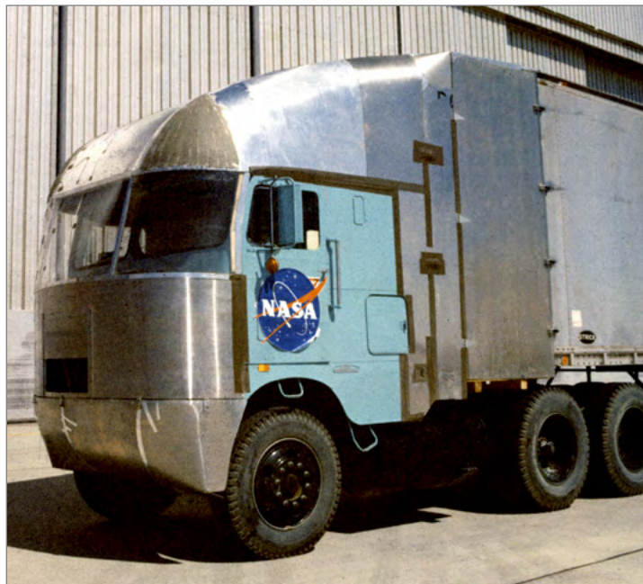
The final configuration of the tractor-trailer with the center modified to reduce its aerodynamic drag. (Photo credit: NASA)
