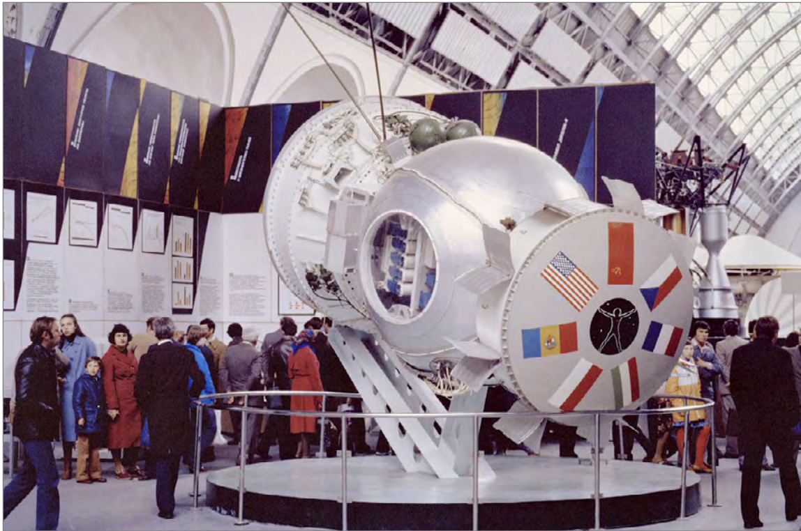
A mock-up of a Bion spacecraft on display at the Space Pavilion in Moscow. The central spherical module (similar to the Zenit bus) was adapted from the Vostok spacecraft, a smaller version compared to the Soyuz. (Photo credit: NASA)
