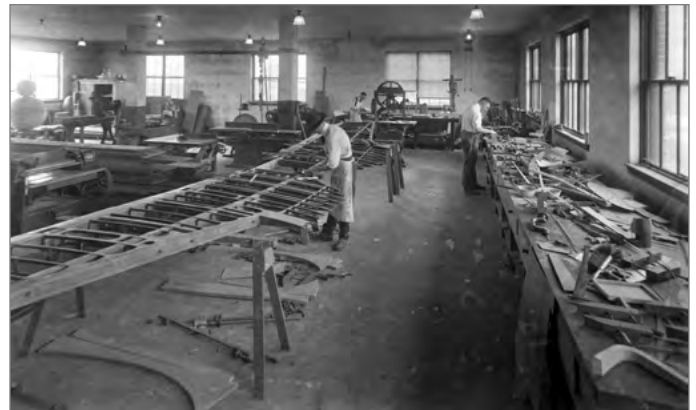
Top: Percy Keffer at Sphere Making Apparatus. Bottom: Workers in the pattern makers' shop manufacture a wing skeleton for a Thomas-Morse MB-3 airplane for pressure distribution studies in flight, June 1922. (Photo credits: NASA)
