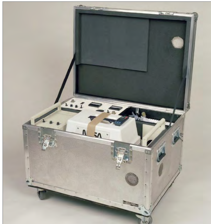
Rapid payload recovery during Bion missions was crucial for many of the experiments on board, including the many experiments that had nothing to do with primates. This bio-transporter case had environmental controls to keep bio-specimens stable for transport and distribution to NASA's space biologists and their international collaborators once the specimens had been retrieved from the spacecraft shortly after landing. (Photo credit: NASA/Tom Trower)
