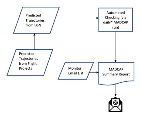
\*Frequency of execution used for current Lunar orbiters. Frequency can be increased/decreased if conditions render it necessary or desirable. Red event threshold values are based on each Project's three-sigma trajectory uncertainty estimates and are provided by the Project to the MADCAP Team.
