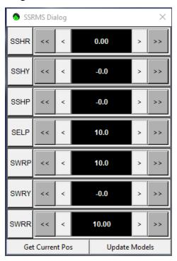
Use the SSRMS Dialog to modify the joint angles of the SSRMS by inputting values into the text boxes or clicking the arrow buttons. Click Update Models button to apply changes.
