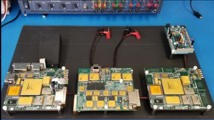
Quad-core flight computer, 100-300 krad TiD, redundant, low power (<10W)
