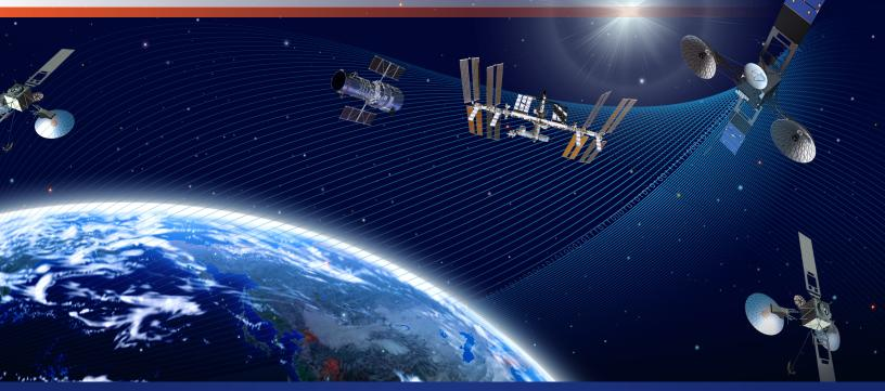
NASA's Tracking and Data Relay Satellites (TDRS) provide communications services to NASA's most storied missions. Through this constellation of satellites, NASA has the ability to transmit valuable spacecraft data via a bent-pipe relay system from anywhere in low-Earth-orbit.
