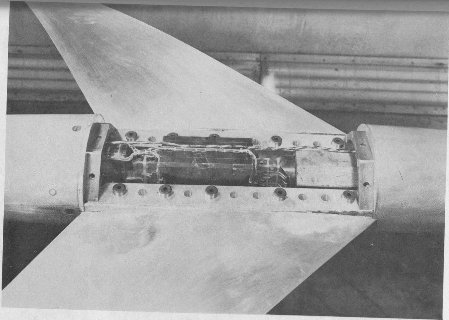
Figure 9.- An internal strain-gage balance installation. Top cover of model fuselage is removed.
