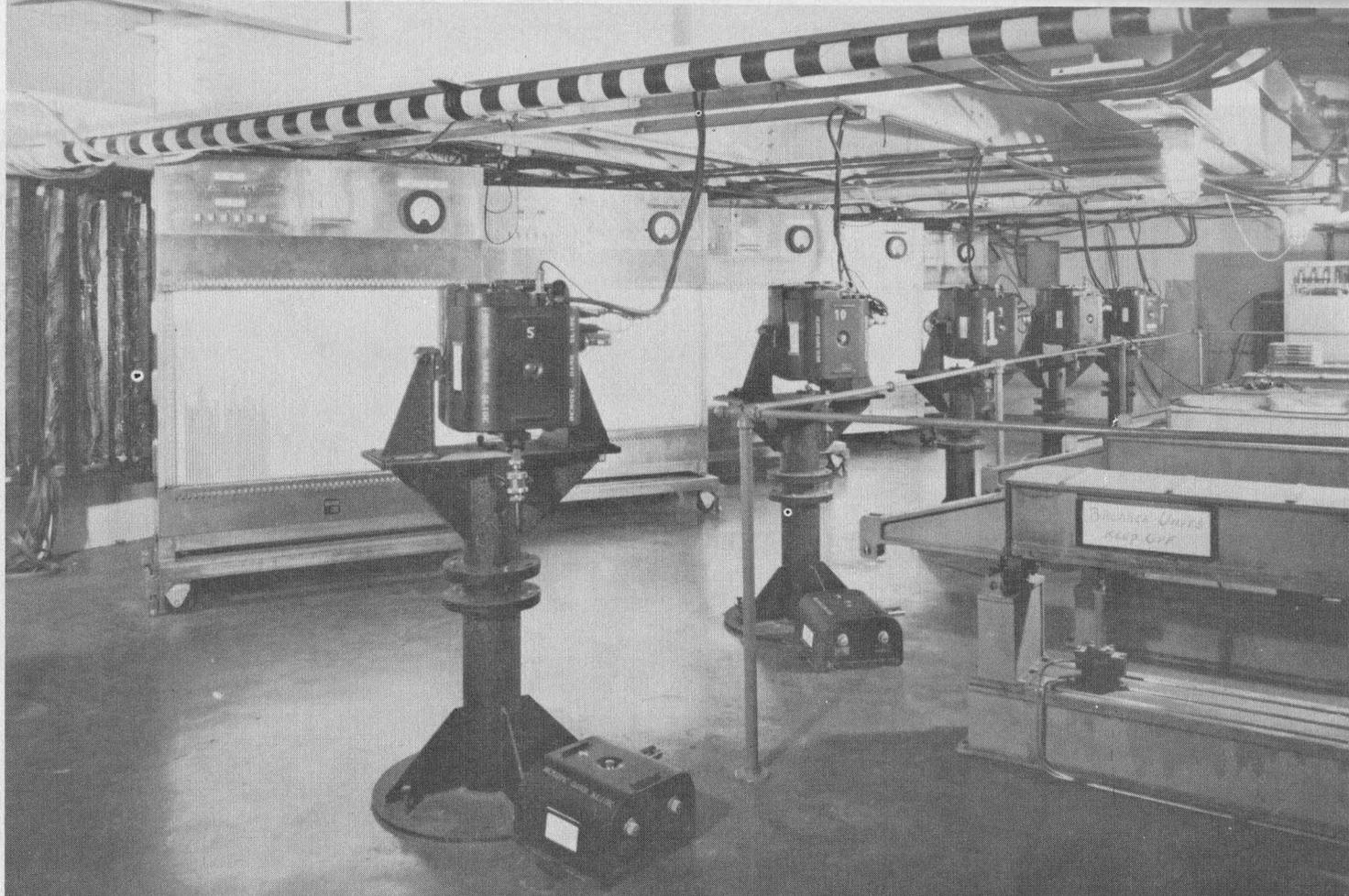
Figure 7.- Mercury manometers and cameras used for steady pressure measurements at the Langley
