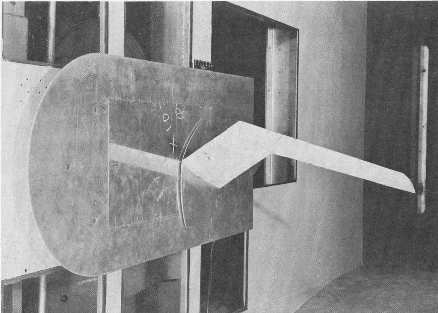
Figure 4.- Reflection-plane semispan-model installation in the Langley 300-MPH 7- by 10-foot tunnel. L-68735
