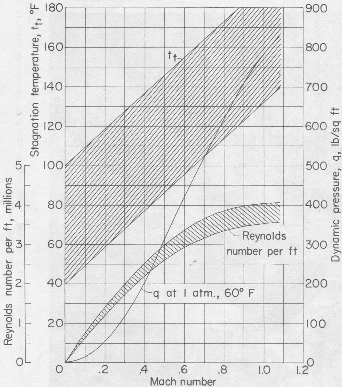
Figure 4.- Variation of stagnation temperature, Reynolds number per foot, and dynamic pressure with Mach number. Langley 16-foot transonic tunnel.
