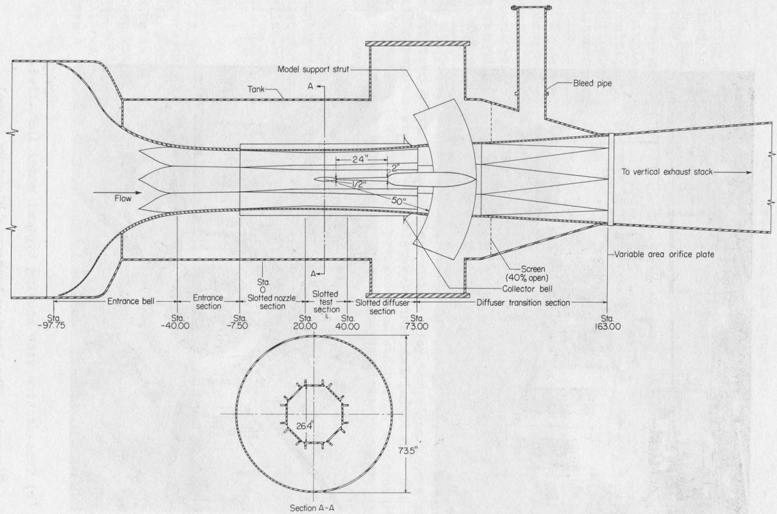
Figure 2.- Sketch of the test section in Langley transonic blowdown tunnel.
