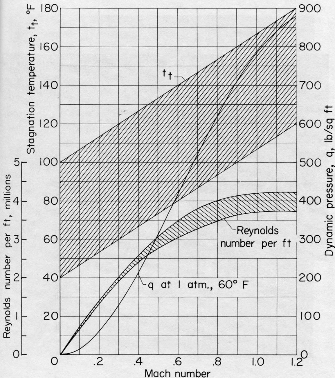
Figure 4.- Variation of stagnation temperature, Reynolds number per foot, and dynamic pressure with Mach number. Langley 8-foot transonic tunnel.
