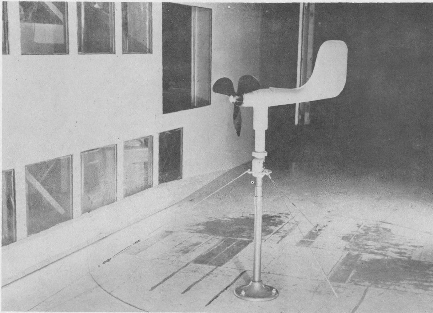
Figure 9.- Wind-velocity and direction indicator investigated in the Langley 300-MPH 7- by 10-foot tunnel.
