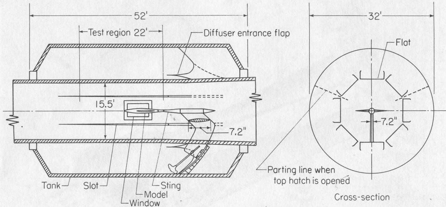
Figure 2.- Schematic sketch of the test section of the Langley 16-foot transonic tunnel.
