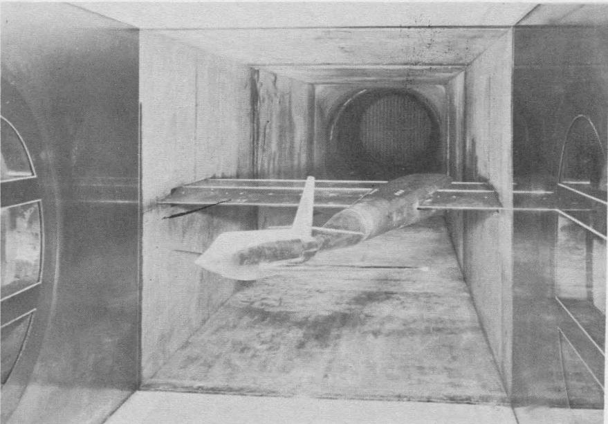
(b) Model set for sideslip tests. L-62227
