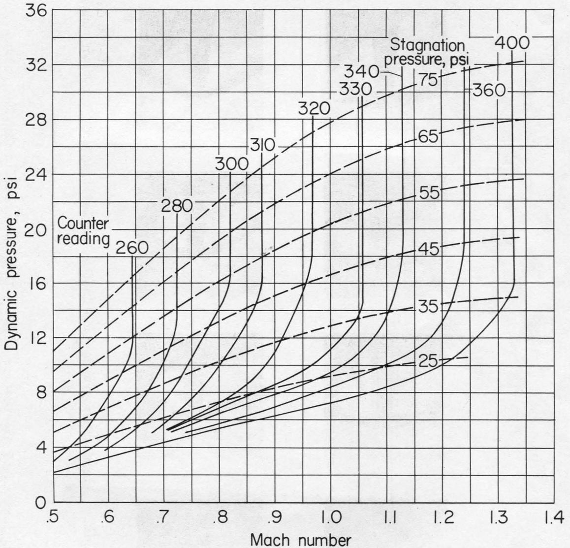
Figure 3.- Operating ranges of stagnation and dynamic pressures and Mach number with bleed duct closed. Langley transonic blowdown tunnel.
