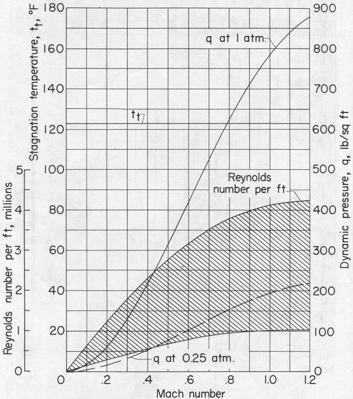
Figure 3.- Variation of stagnation temperature, Reynolds number per foot, and dynamic pressure with Mach number. Langley 8-foot transonic pressure tunnel.
