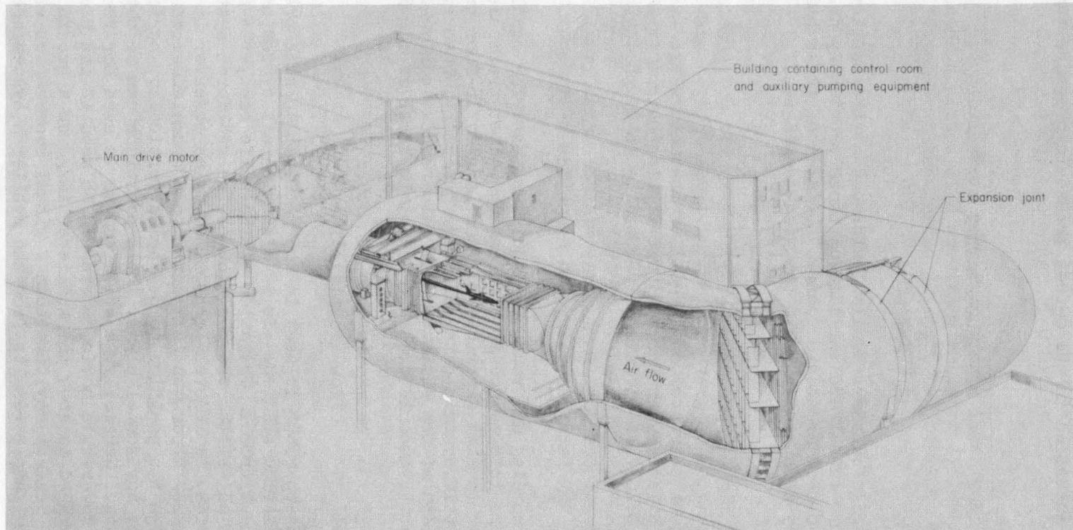
Figure 1.- Perspective drawing of Langley 8-foot transonic pressure tunnel. L-57-2529
