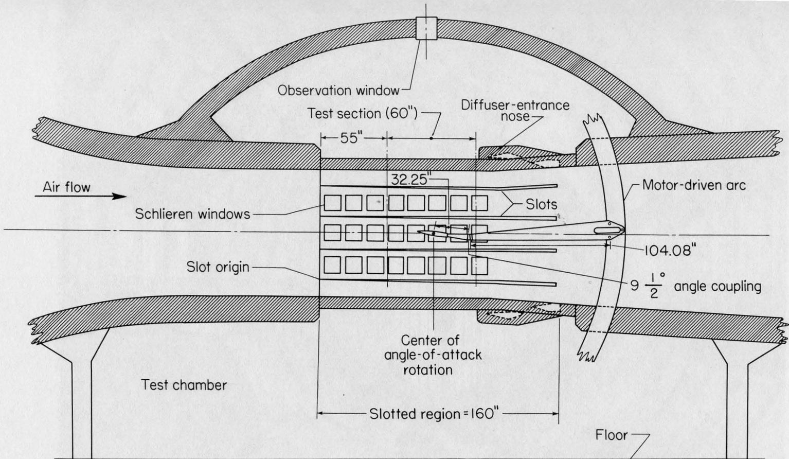
Figure 2.- Details of test section in the Langley 8-foot transonic tunnel.
