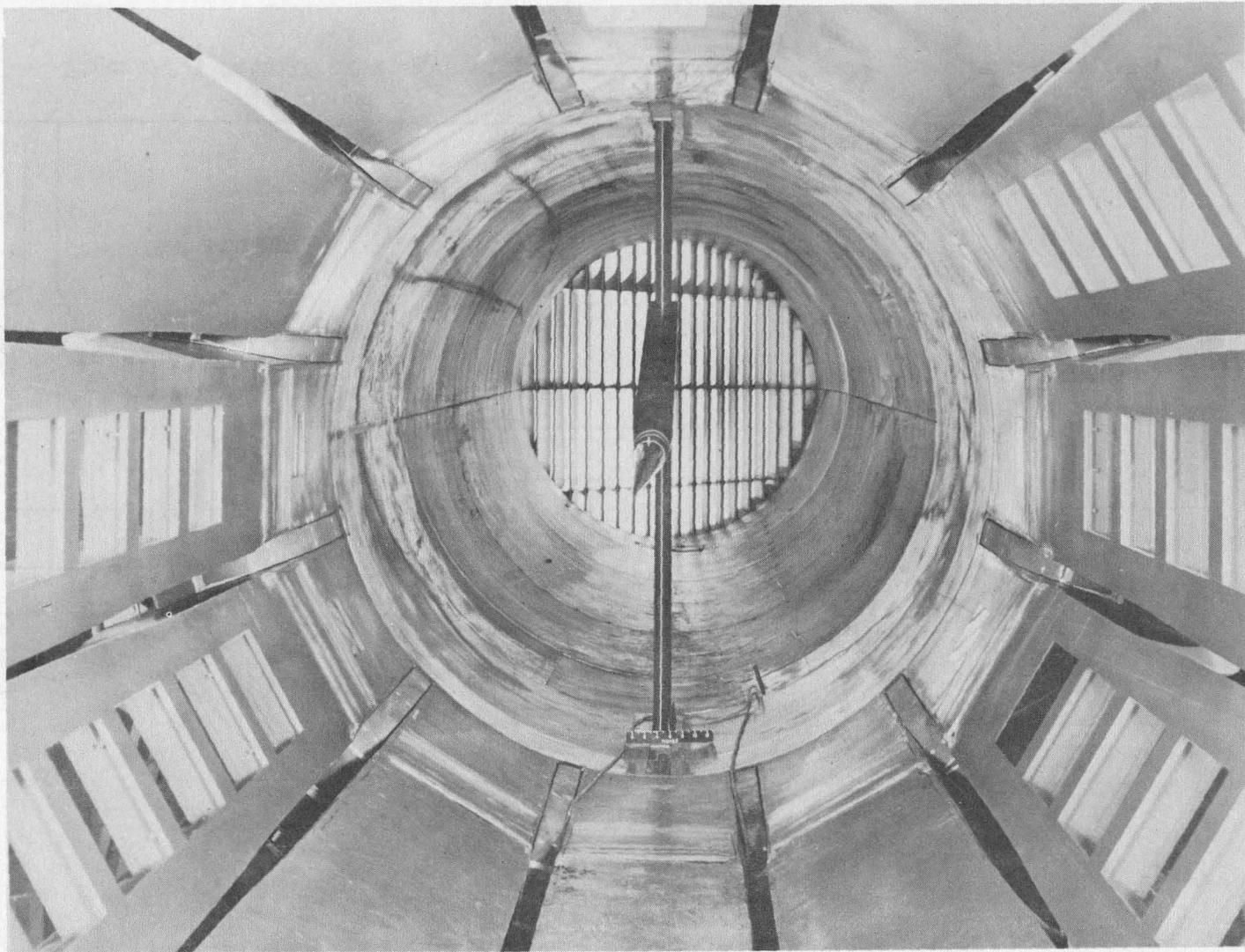
Figure 3.- Interior view of the test region in the Langley 8-foot transonic tunnel. L-57-959
