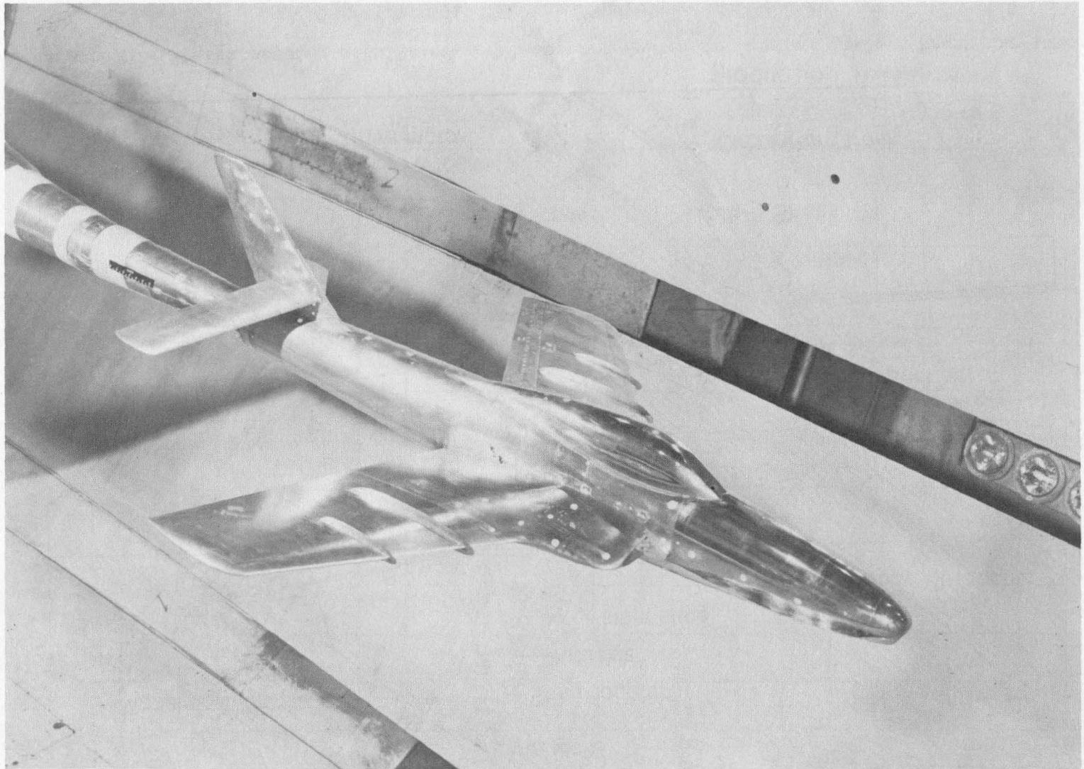
Figure 6.- A typical model installation in Langley 16-foot transonic tunnel.
