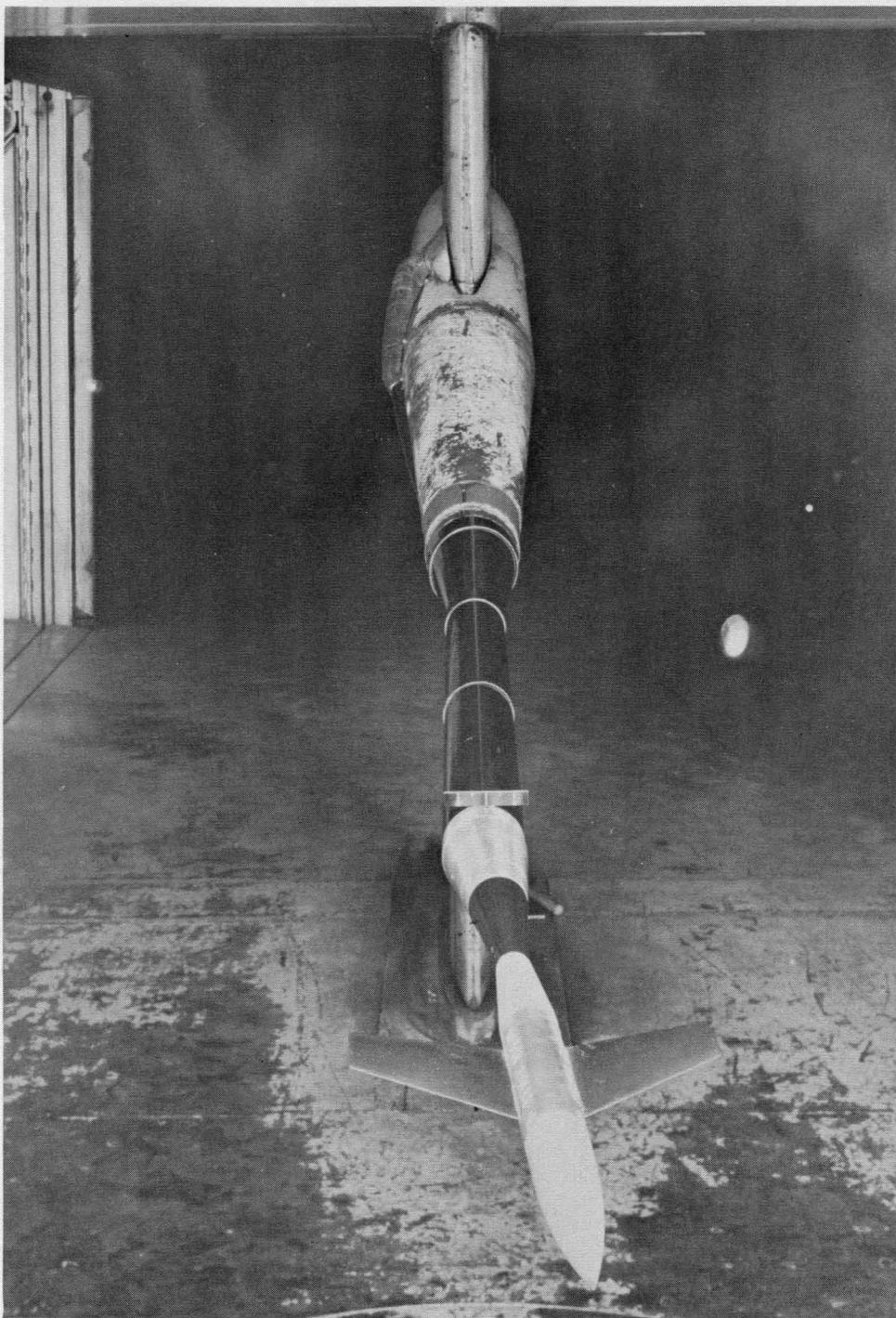
Figure 6.- A model installation on the variable-sideslip sting in the Langley high-speed 7- by 10-foot tunnel. L-89040
