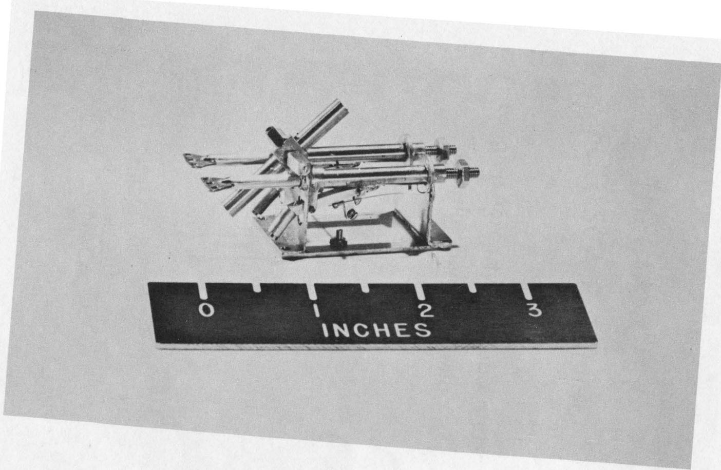
Figure 6.- Remote-control mechanism used in spin models for Langley
