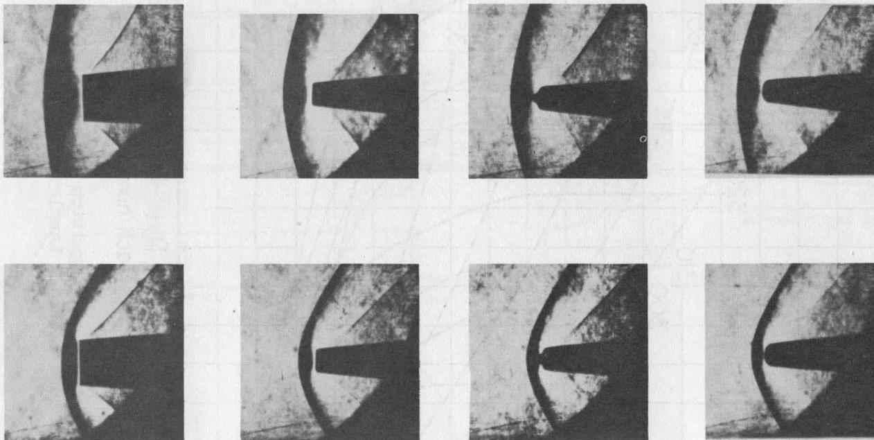
Figure 4.- Sample schlieren photographs made in the Langley transonic blowdown tunnel. L-85651.1
