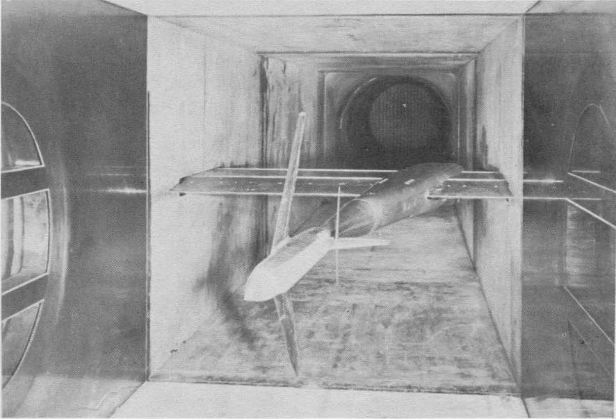
(a) Model set for angle-of-attack tests. L-62225
