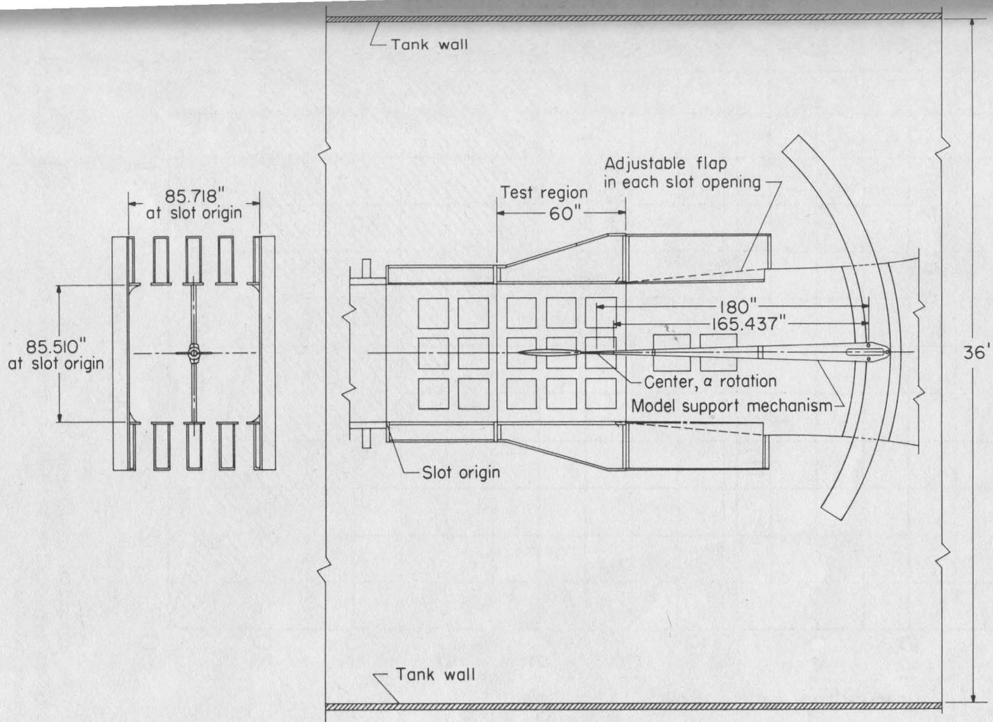
Figure 2.- Details of test section and location of model in the Langley 8-foot transonic pressure tunnel.
