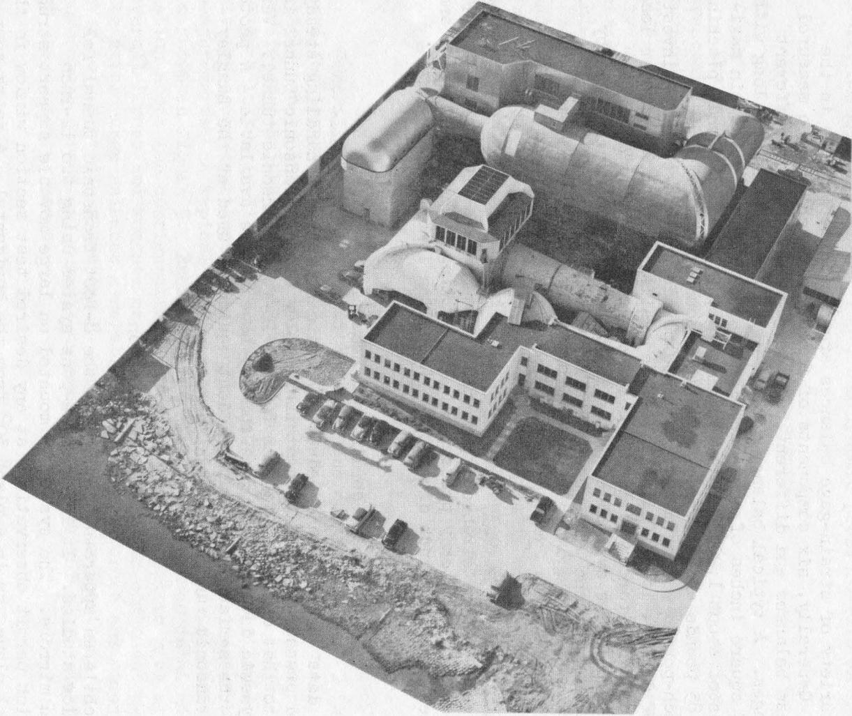
Figure 1.- Aerial photograph of 8-foot tunnels. The 8-foot transonic tunnel is in the foreground; the 8-foot transonic pressure tunnel in the background.
