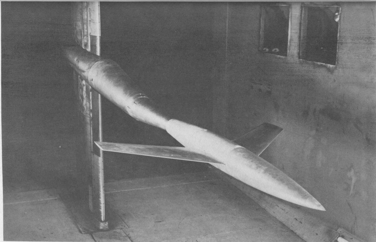
Figure 5.- A typical sting-supported-model installation in the Langley high-speed 7- by 10-foot tunnel.
