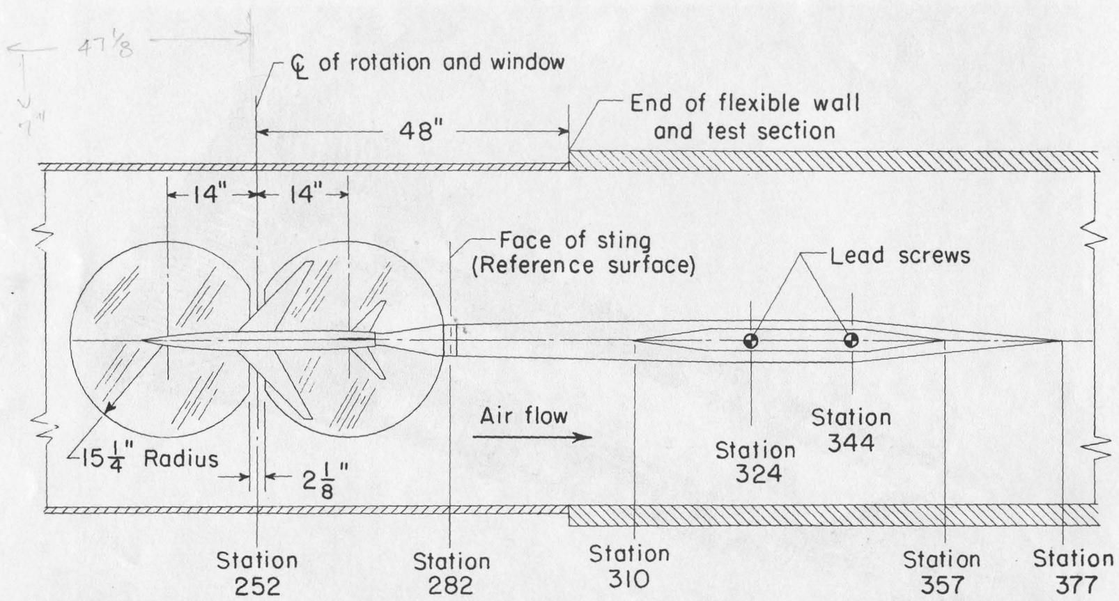
Figure 2.- Sketch showing the position of a model relative to the sting support and to the schlieren window in the Langley 4- by 4-foot supersonic pressure tunnel. (Tunnel stations in inches; reference station 0 taken at the start of the flexible nozzle.)
