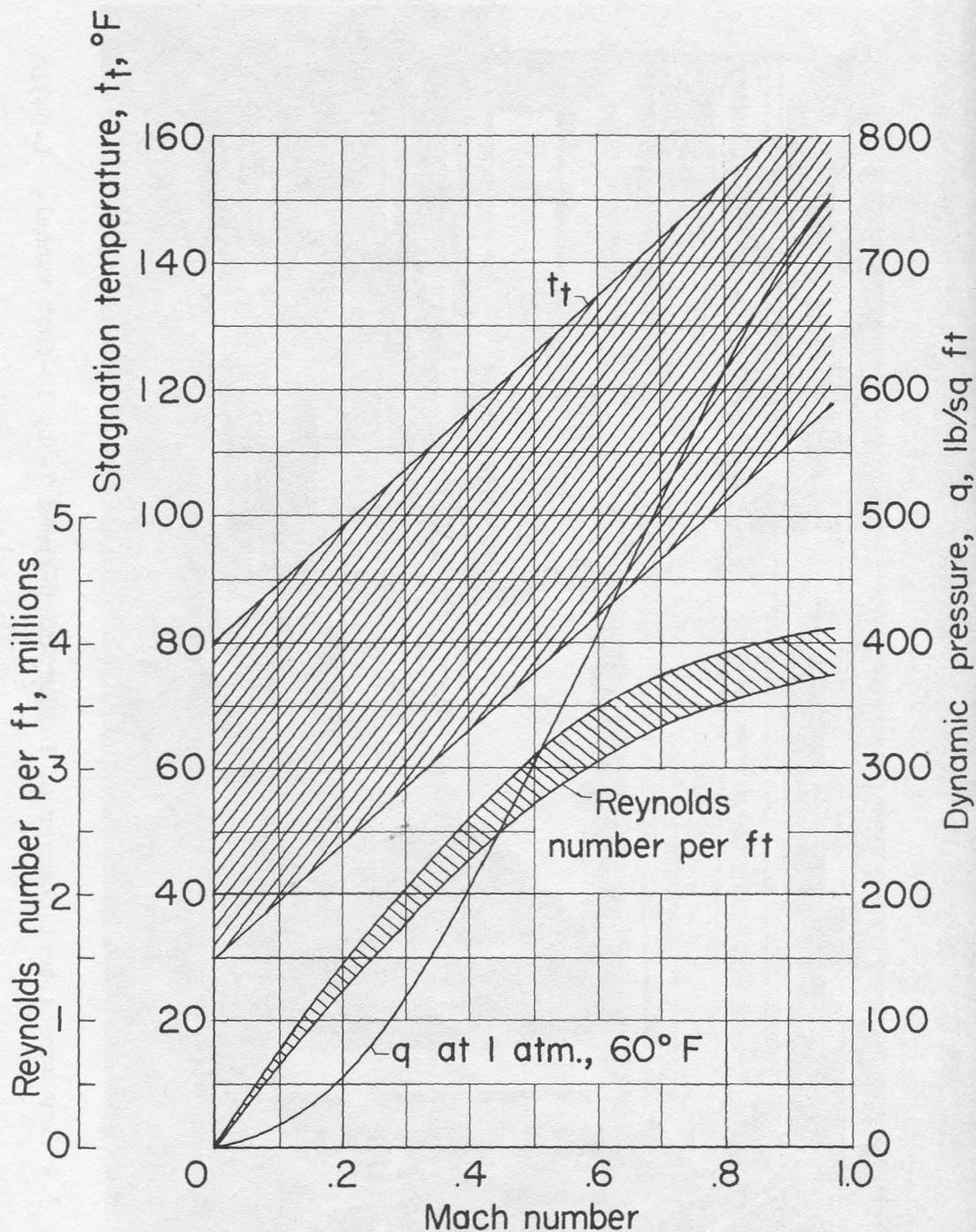
Figure 4.- Variation of stagnation temperature, Reynolds number per foot, and dynamic pressure with Mach number. Langley high-speed 7- by 10-foot tunnel.
