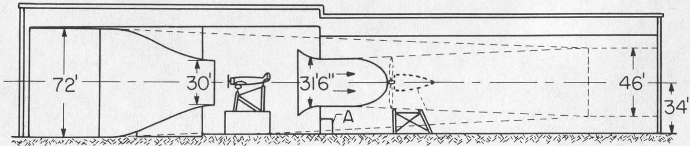
Figure 1.- Plan and elevation sketch of the Langley full-scale tunnel.
