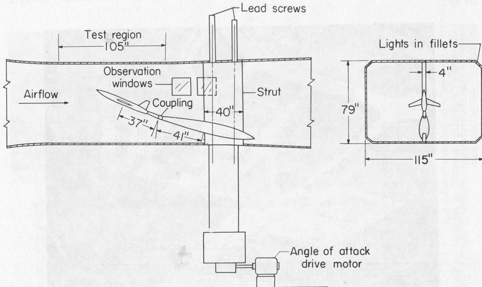
Figure 2.- Sketch of test section and sting support system of the Langley high-speed 7- by 10-foot tunnel. All dimensions in inches.
