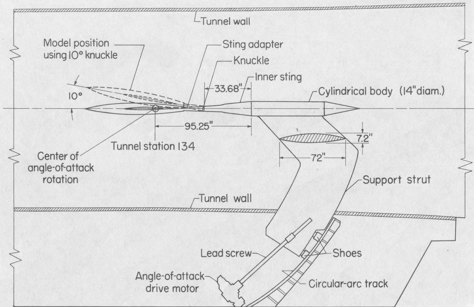
Figure 5.- Sketch showing details of model-support system in Langley 16-foot transonic tunnel.
