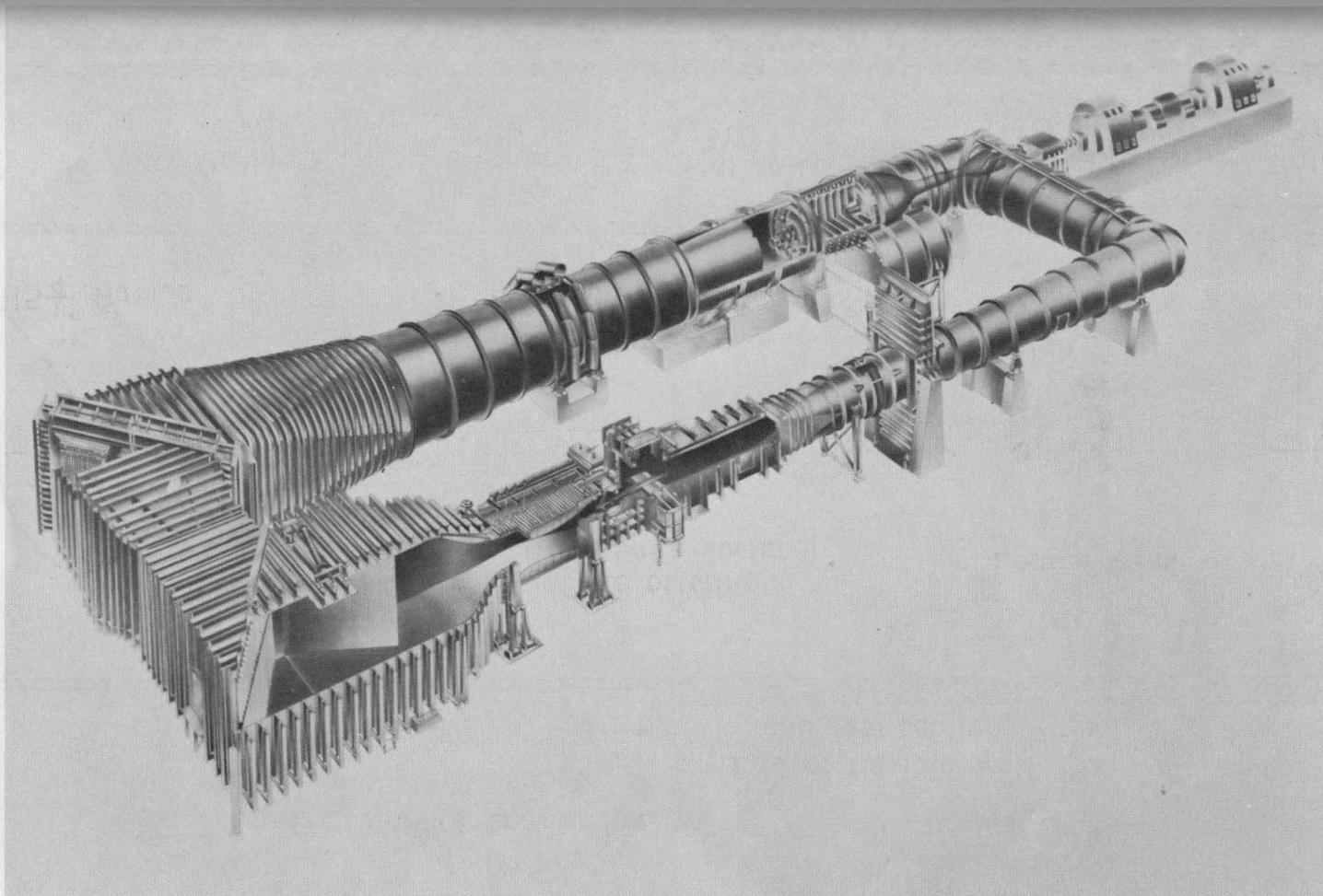
Figure 1.- Pictorial drawing of the Langley 4- by 4-foot supersonic pressure tunnel.
