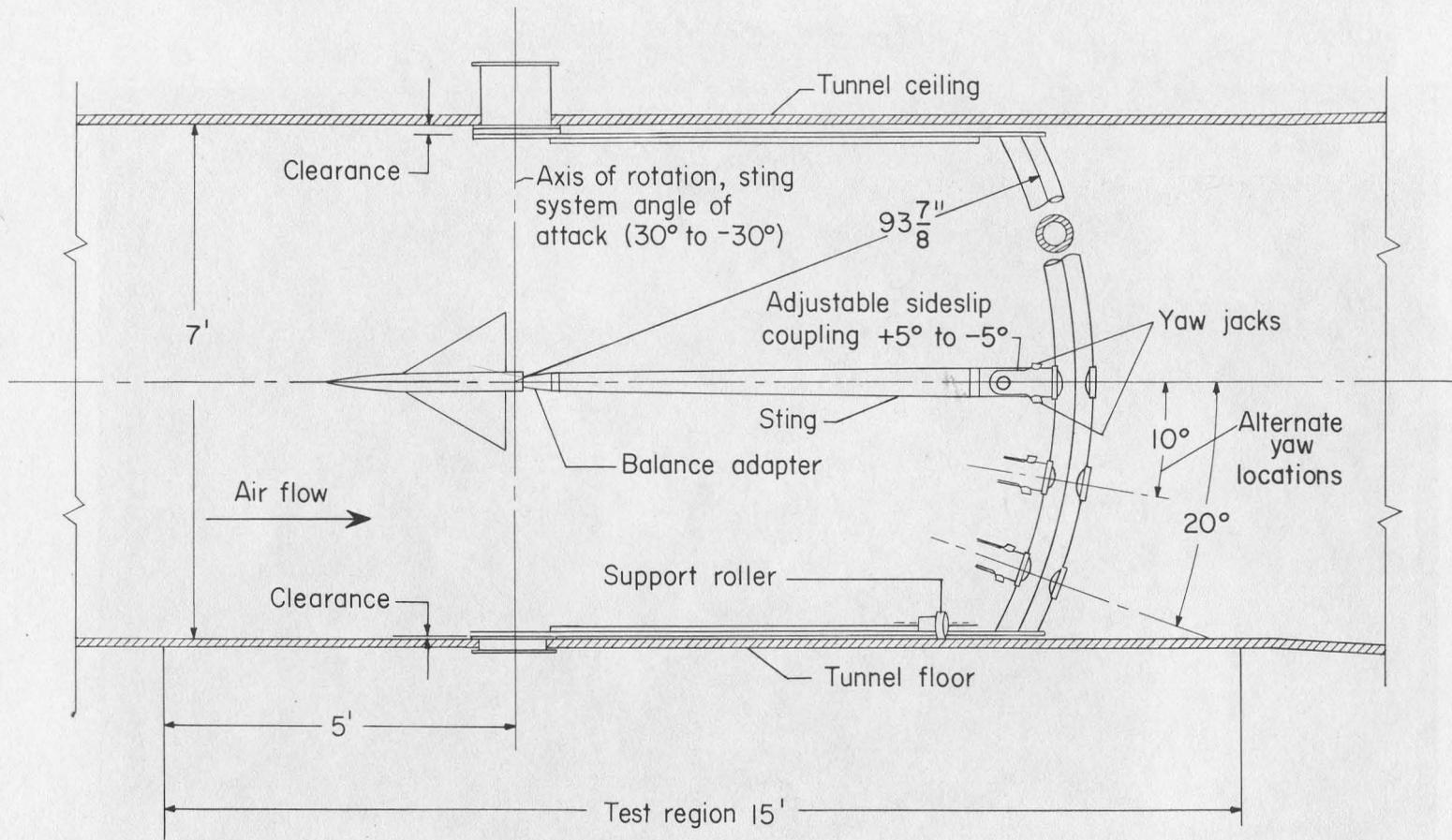
Figure 7.- Diagram of the sting-support system in the Langley 300-MPH 7- by 10-foot tunnel.
