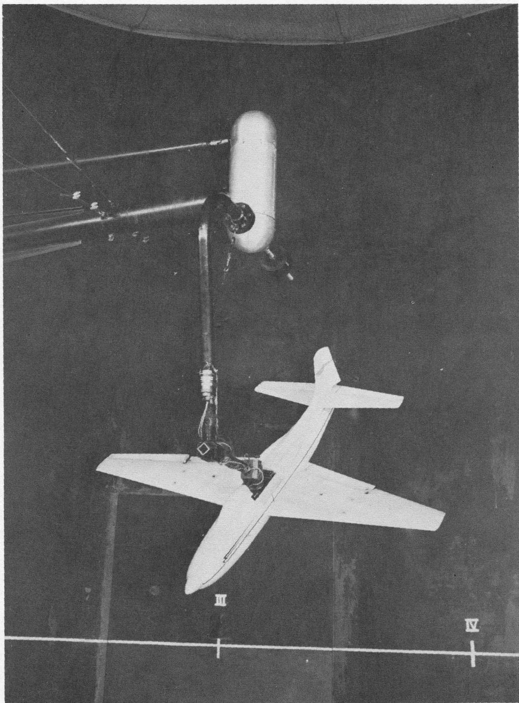
Figure 4.- Gooseneck rotary arm support for models or, used in Langley
