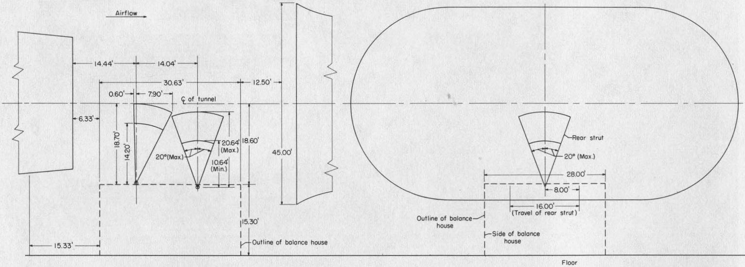
Figure 4.- Diagram of the relative positions of the support struts and their ranges of travel. Langley full-scale tunnel.
