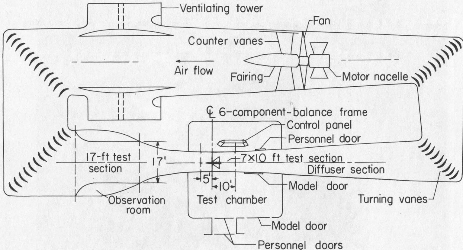
Figure 1.- Plan view of the Langley 300-MPH 7- by 10-foot tunnel.
