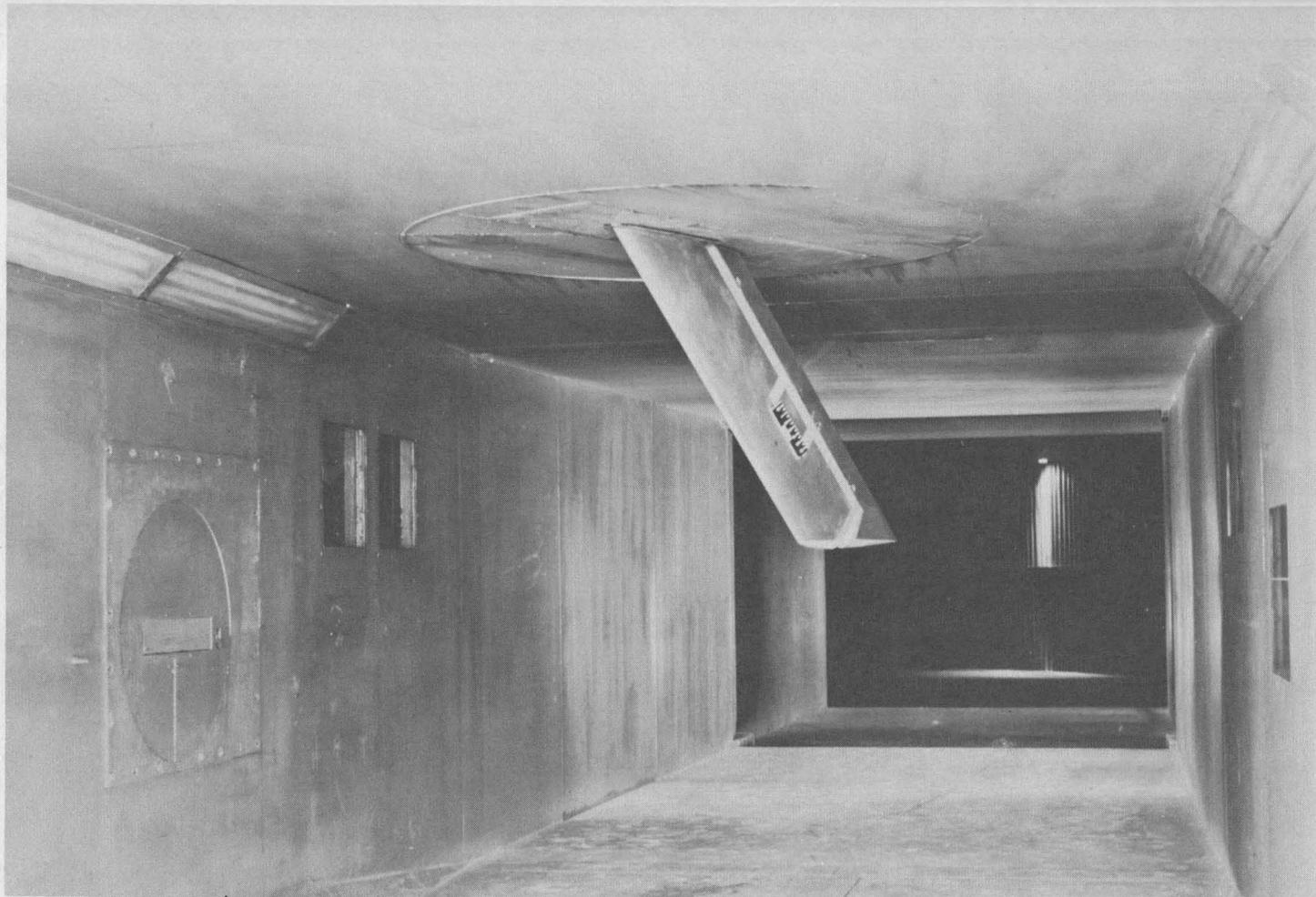
Figure 7.- A ceiling-mounted semispan model installation in the Langley high-speed 7- by 10-foot tunnel.
