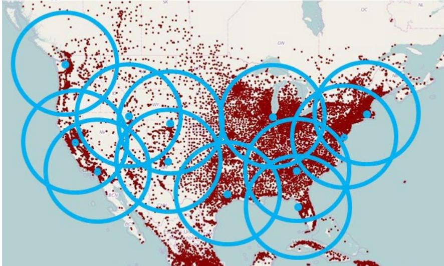
Figure 11: An example of deploying ground stations so that major population centers and federal research centers are connected through qEDISON. The circle radii correspond to roughly 1100 km, less than the reach of both the Stage 1 LEO and Stage 2 MEO satellites; for this ground station separation the Stage 1 performance is considerably higher.
