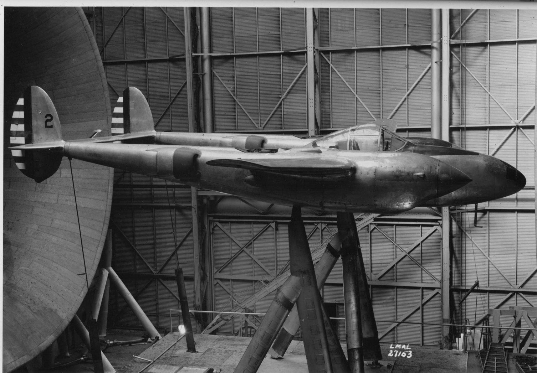
Figure 3. - Prestone duct entrances modified to those of the P-38E airplane.
