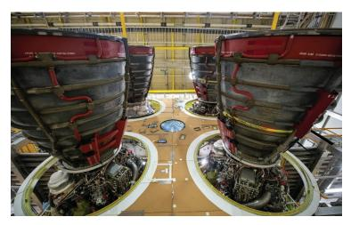
The Artemis I RS-25 engines installed in the core stage during assembly at NASA's Michoud Assembly Facility in New Orleans.
