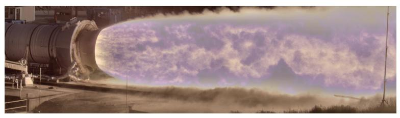
Boosters lead contractor Northrop Grumman and NASA hot-fired several full-scale solid rocket motors to help qualify them for the SLS Program.
