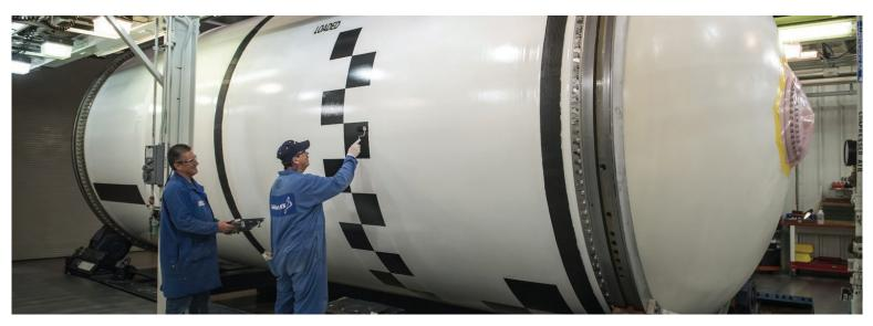
Technicians with lead solid rocket boosters contractor Northrop Grumman paint photogrammetric markings on one segment of an SLS solid rocket motor. The black-and-white targets painted on each element of the rocket provide targets for cameras, which then use those positions compared with fixed positions on the ground and on the mobile launcher to precisely locate SLS in space.
