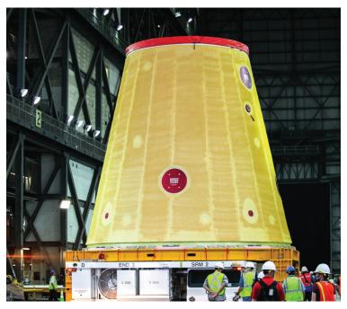
The Artemis I launch vehicle stage adapter arrives at the Vehicle Assembly Building for stacking on the Artemis I rocket.
