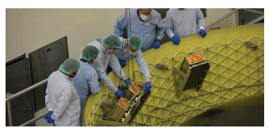
The Artemis I Orion stage adapter with mounting brackets for secondary payloads.
