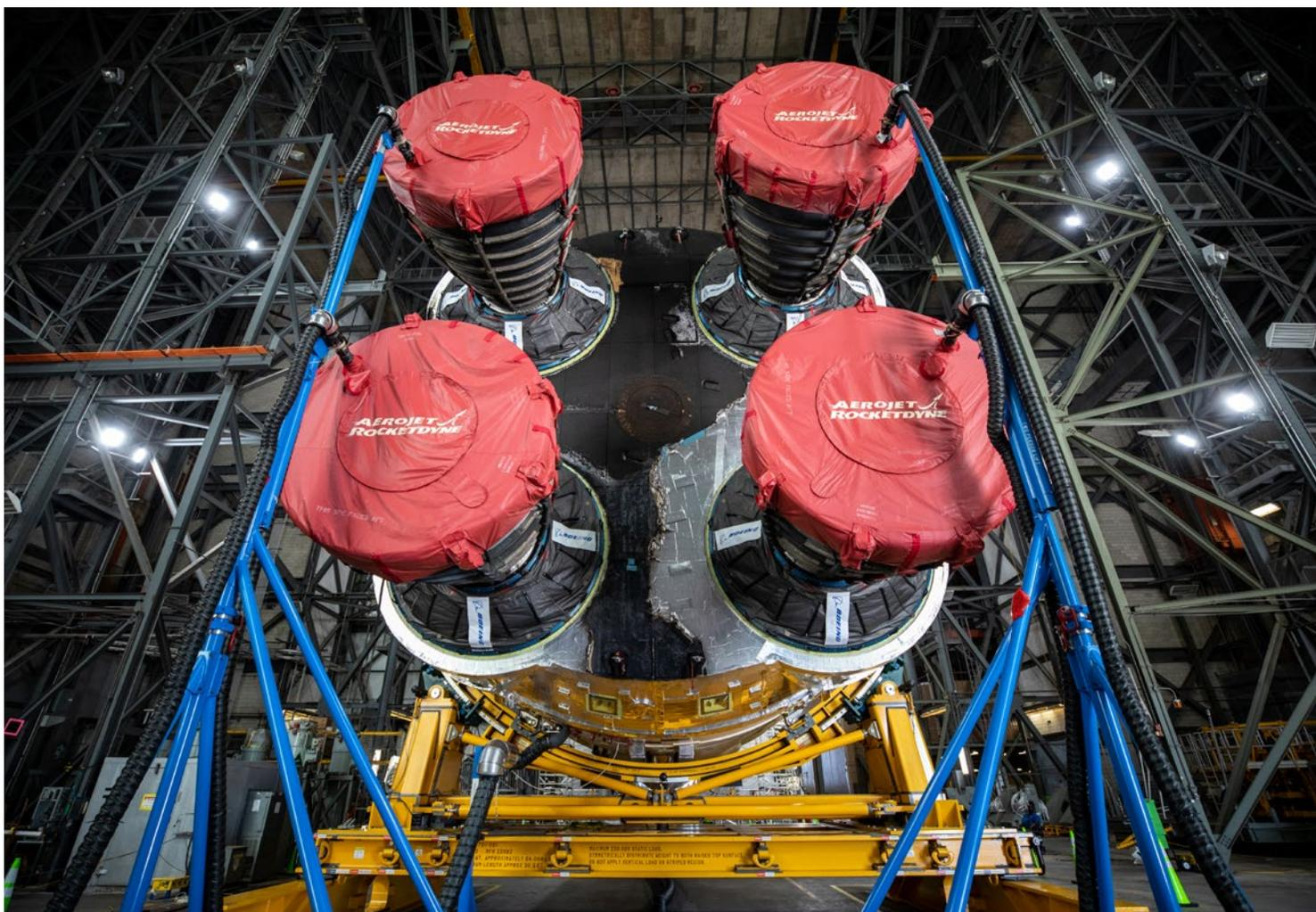
Industry partner Aerojet Rocketdyne, headquartered in Sacramento, California, supplies RS-25 engines for the SLS core stage and RL10 engines for the ICPS.
