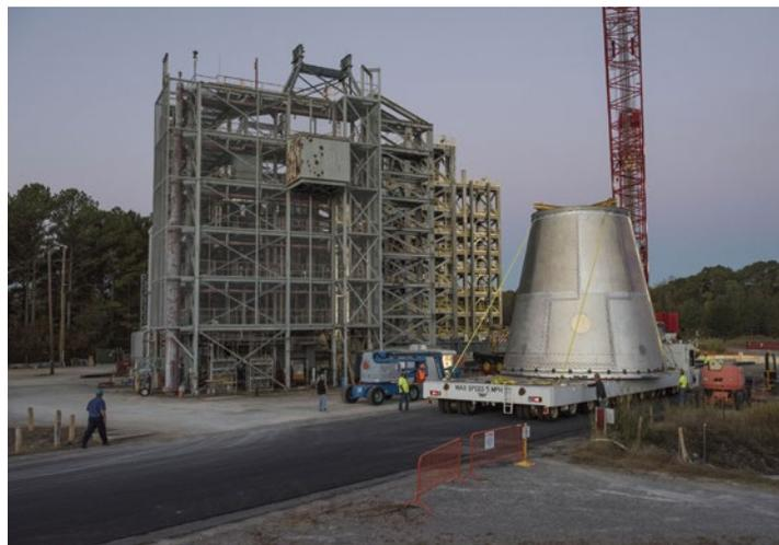
*The launch vehicle stage adapter structural test article for the Integrated Structural Test was manufactured and tested at Marshall.*
