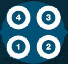
Shown here from the bottom, looking up at the rocket from below, four liquid hydrogen (**LH2**) and liquid oxygen (**LOX**)-fueled **RS-25 ENGINES** are arranged in a square pattern, like legs on a table, providing stability and even distribution of propulsion forces to the rocket. At launch, they will produce
