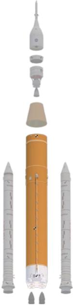
The SLS **core stage** is the tallest rocket stage NASA has ever built. It measures approximately 212 ft. (64.6 m) tall and 27.6 ft. (8.4 m) in diameter (excluding thermal protection system foam and flanges). Its fully fueled weight, excluding engines, is 2.4 million lbs. (1,088 t).
