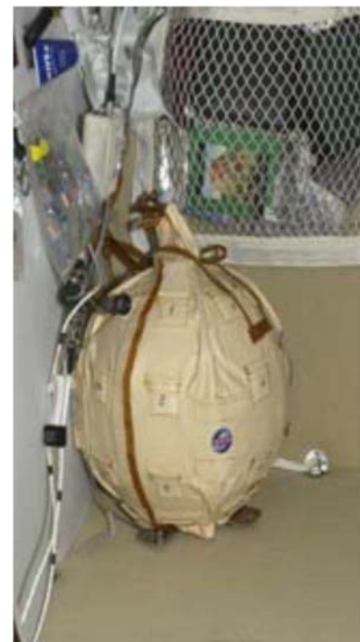
Spherical phantom in the ISS SM crew quarter (Image provided by RSC Energia)
