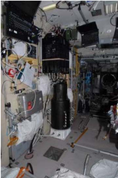
Torso phantom in the interior of the ISS RS on the left wall. (Image provided by RSC Energia).
