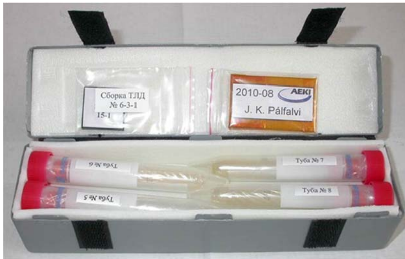
Bioekologiya case for the Biotrek space experiment. Image provided by Biokhimmash.
