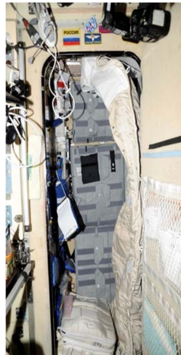
Protection screen on the wall of the ISS SM crew quarter, shown with the arrow (photo presented by RSC Energia)
