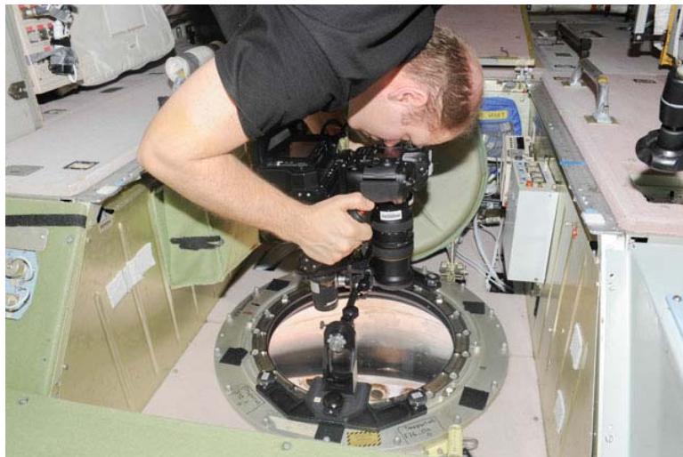
At a window in the International Space Station's Zvezda Service Module, ISS crewmember Oleg Kotov uses a digital camera photospectral system to perform a session for the Albedo Experiment (ISS038E005022).
