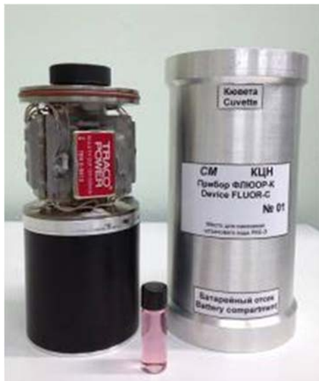
Fluor-C Device containing human lymphocyte cell suspension.
