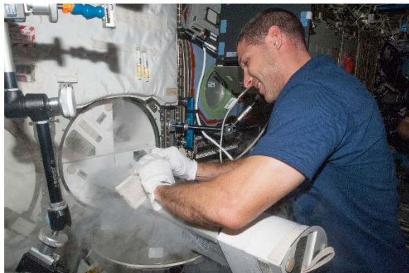
ISS crewmember Michael Hopkins, Expedition 37 flight engineer, prepares to insert samples into a Minus Eighty Laboratory Freezer for ISS (MELFI) dewar tray in the International Space Station's Destiny laboratory (ISS037E010720)
