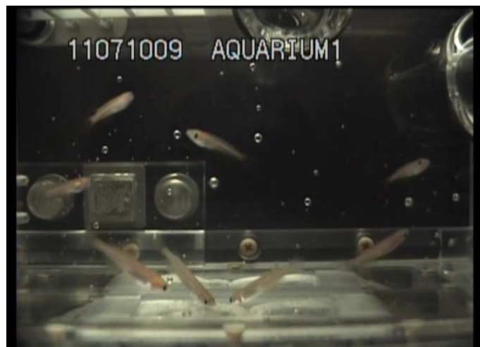
Video Screen Shot of Medaka in the Aquatic Habitat onboard the ISS. Image courtesy of JAXA.
