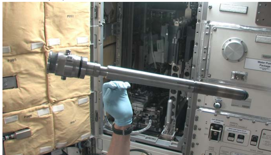
Video screen shot of a levitating sample cartridge removed from the Gradient Heating Furnace in the ISS.
