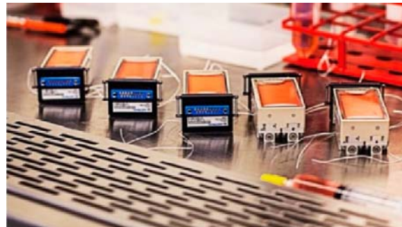
Cell suspensions prepared in six spaceflight experiment containers flown to the ISS. Image Daniela Grimm.
