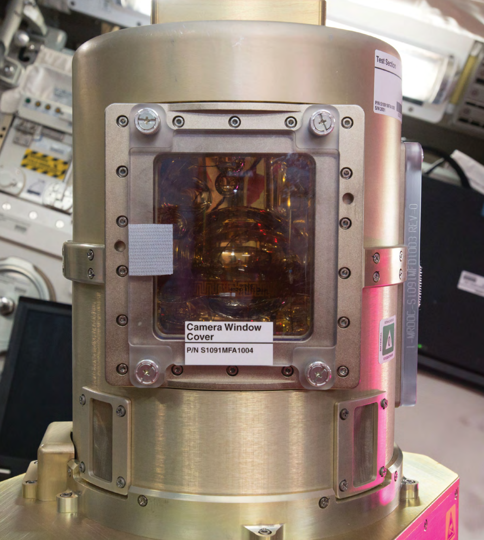
A view of the Zero Boil-Off Tank (ZBOT) experiment Vacuum Jacket Camera Window Cover hardware. ZBOT uses an experimental fluid to test active heat removal and forced jet mixing as an alternative means for controlling tank pressure for volatile fluids. Results from the investigation improve models used to design tanks for long-term cryogenic liquid storage, which are essential in biotechnology, medicine, industrial, and many other applications on Earth. (iss051e028301)
