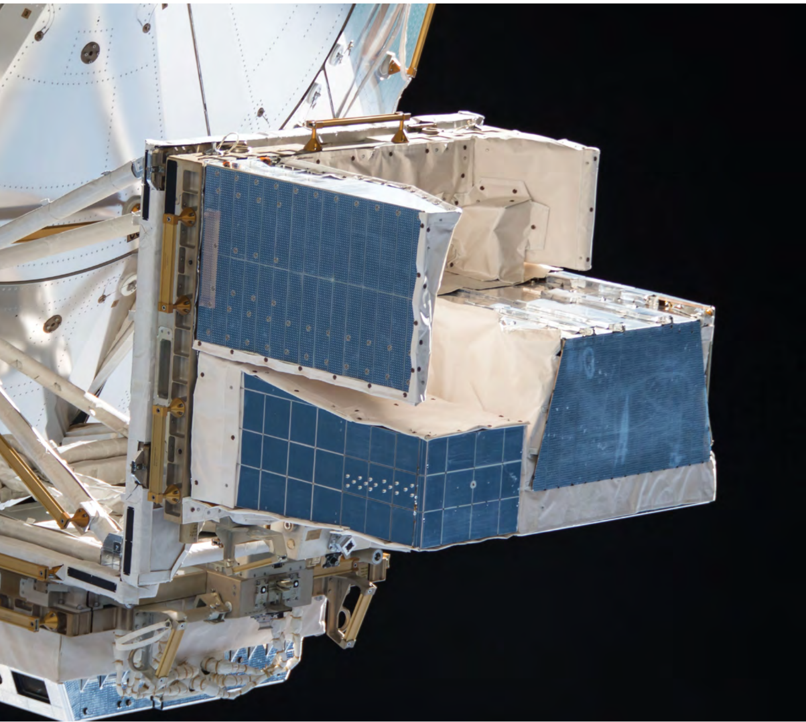
View of the External Payload Facility attached to the Columbus European Laboratory. The Atmosphere-Space Interactions Monitor and High Definition Earth Viewing payloads are in view. Photo was taken by the ground-controlled External High Definition Camera 3 (iss057e080463).
