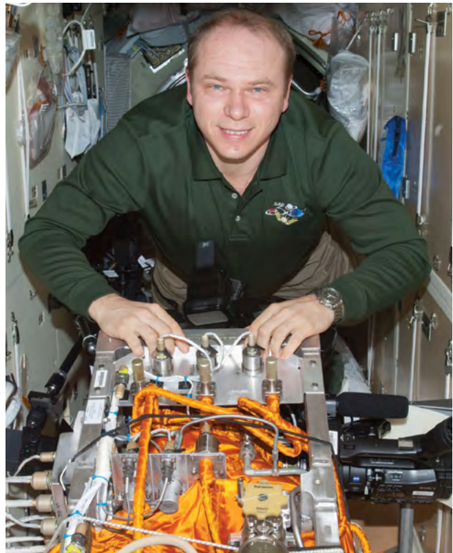
Figure 18. Russian cosmonaut Oleg Kotov, Expedition 38 commander, sets up the Particle Cooler/Generator Module for the Kaplya-2 experiment in the Rassvet Mini-Research Module 1 (MRM1) of the ISS (iss038e029764).
