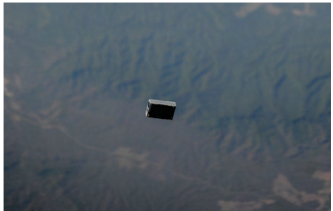
Figure 22. A view of the ASTERIA satellite moments after deployment from the ISS. ASTERIA is a six-unit CubeSat, deployed from the ISS, that tests new technologies for astronomical observation such as the detection of planets outside our solar system (iss053e470644).
