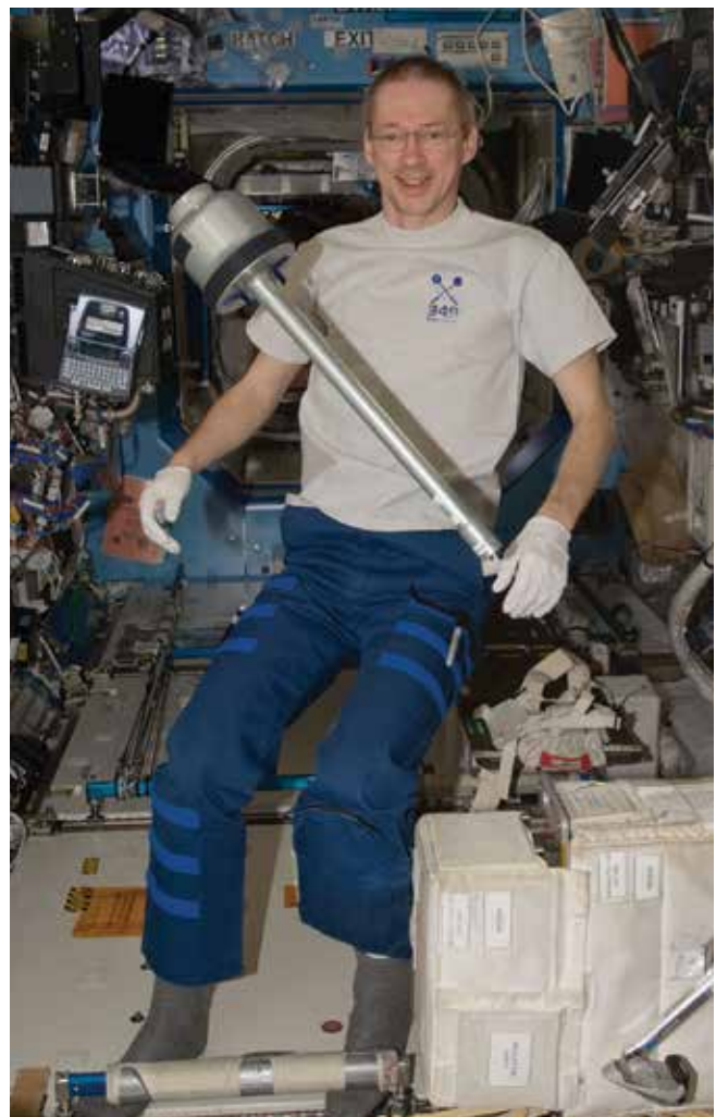
ISS crew member Frank De Winne removes a CETSOL sample cartridge assembly from its MSL mechanical protection container tube during MSL commissioning activities on board ISS (ISS021E023149).
