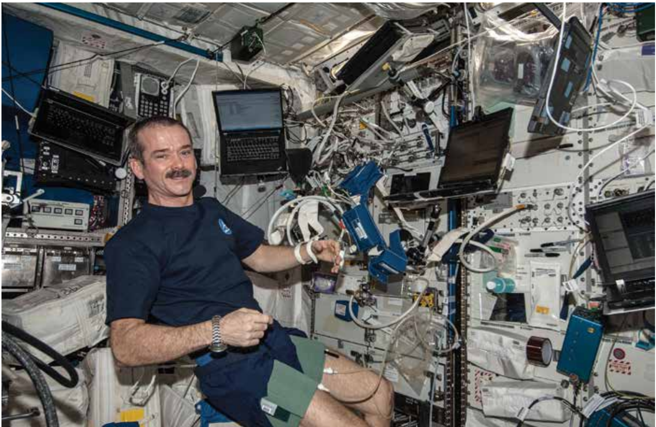
ISS crew member Chris Hadfield is photographed during BP Reg operations. He is wearing the Leg/Arm Cuff System on his thighs, and the Continuous Blood Pressure Device on his left hand. (ISS035E022360).
