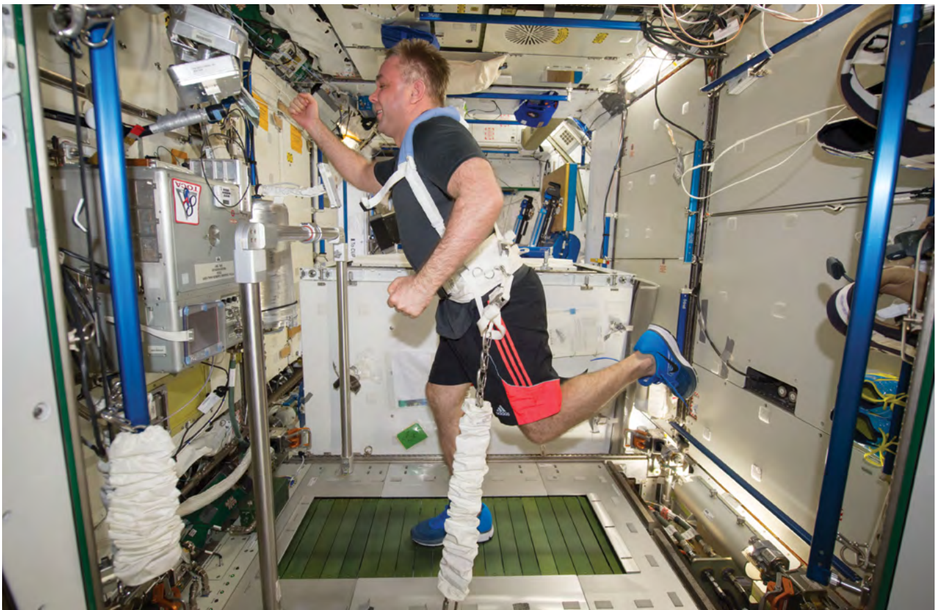
ISS crewmember Maxim Suraev, equipped with a bungee harness, exercises on the Combined Operational Load Bearing External Resistance Treadmill (ISS041E011475).
