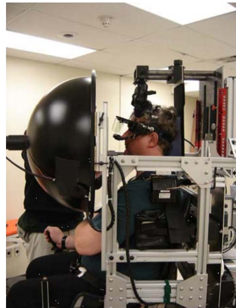
Rotating drum vestibular testing with multi-axis tilt device. ESA image.
