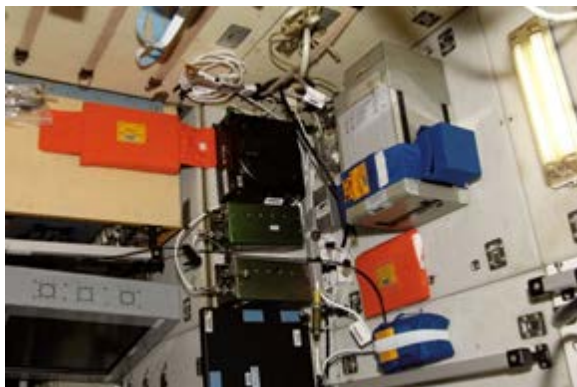
ISS015E11115 – View of a Time Log Table (upper right) and Materials Kits (blue and orange bags) for the Alteino Long Term Cosmic Ray Measurements on board the International Space Station Experiment in the Zvezda Service Module. Photo taken during Expedition 15
