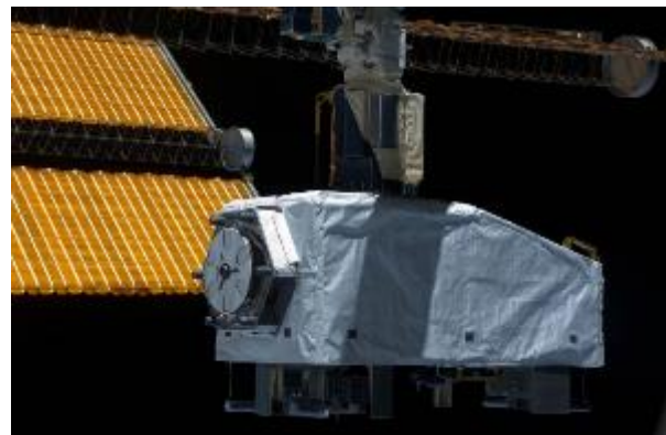
S127E008244 – Close-up view of Kibo arm moving Space Environment Data Acquisition Attached Payload. Solar arrays are visible in the background. JAXA image.
