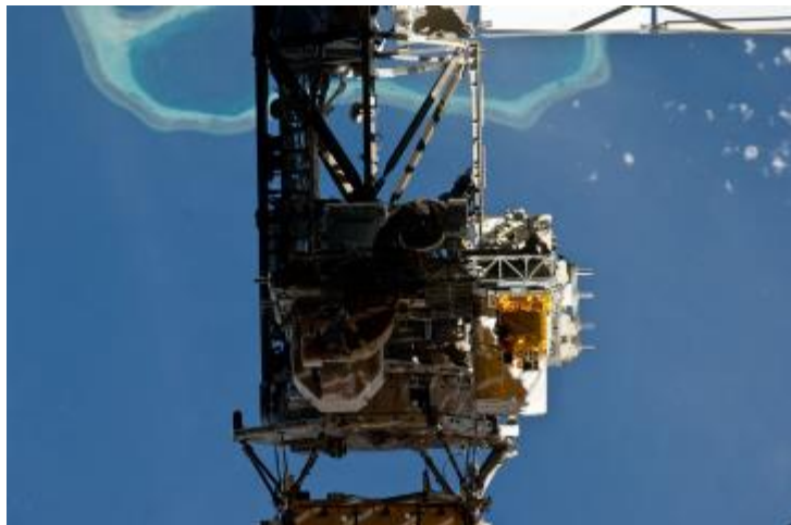
STS-135 fly-around view of the zenith side of the P3 Truss, with STP-H3 on ELC-3 in view.
