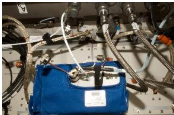
ISS020E022219 - Documentation of the installation of the Dose Distribution Inside ISS (DOSIS) in the Columbus module by the Expedition 20 crew. View is of the DOSIS Main box - with cables and connectors. NASA image.
