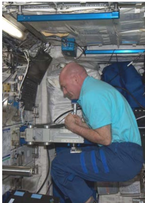
ESA astronaut André Kuipers undertaking Body Mass Measurement for the SODium LOading in Microgravity experiment. ESA/NASA image.
