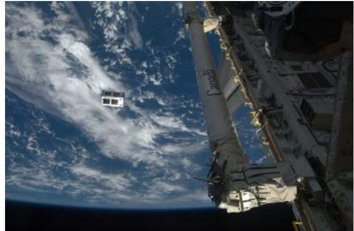
View of the Picosat for the Pico-Satellite Solar Cell Experiment experiment during its deployment from the starboard side of the payload bay of the orbiter Endeavour.
