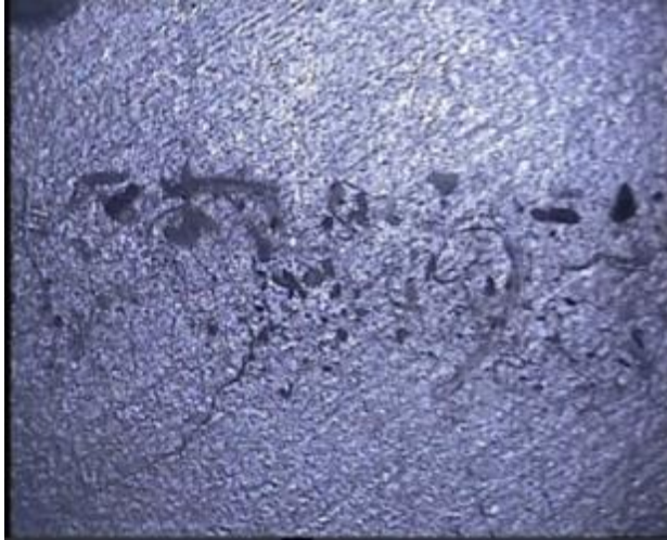
Area behind a panel, the temperature is 11°C with 2,0 \times 10^3 colony-forming unit (CFU) of Ulocladium botrytis and 2,0 \times 10^3 CFU of Aspergillus sydowii . Roscosmos image.
