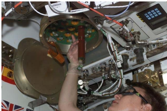
NASA Image: ISS005E19055 - View of Astronaut Peggy Whitson, Expedition Five Flight Engineer, as she places a cartridge into the Zeolite Crystal Growth (ZCG) experiment located in the U.S. Laboratory/Destiny on ISS.
