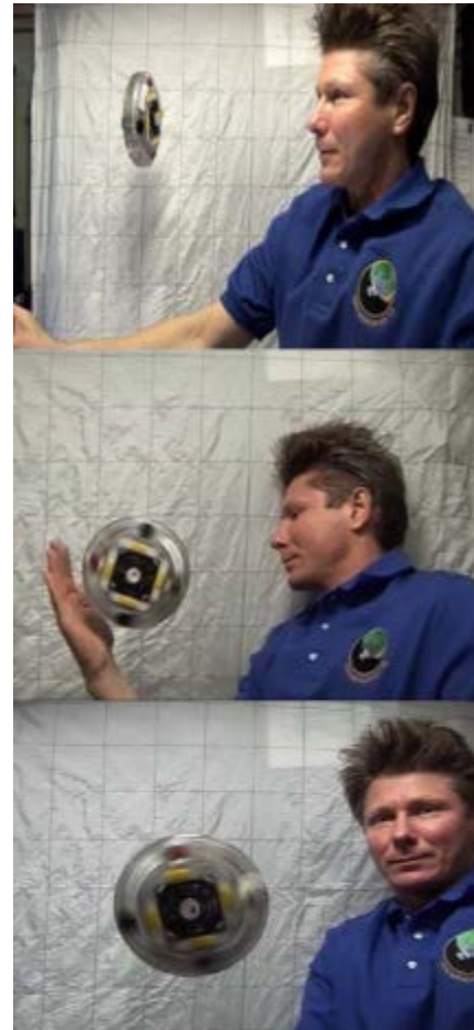
Forward motion of the flying saucer according to Bernoulli’s law, (top). Flying saucer while flying, unstable state (middle). Flying saucer while spinning, stable state (bottom). Roscosmos image.
