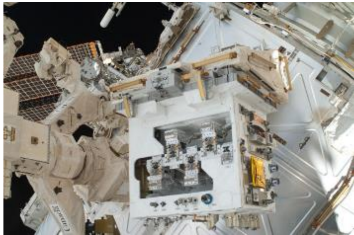
The Robotic Refueling Mission module on the International Space Station, temporarily installed on the Dextre robot's Enhanced Orbital Replacement Unit Temporary Platform.
