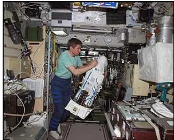
ISS011E13009 – Cosmonaut Sergei K. Krikalev, Expedition 11 commander representing Russia's State Space Corporation, works with the European Space Agency (ESA) Matroshka radiation experiment in the Zvezda Service Module of the International Space Station. Matroshka, a human-torso-like device, was retrieved from the exterior of the station during an August spacewalk for return to Earth. The experiment is designed to better understand the exposure of astronauts, including those making spacewalks, to radiation.
