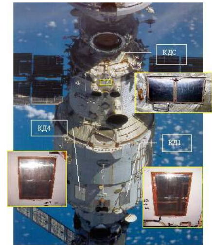
General view of the Station and the placement of sensors on the planes of the Service Module. Roscosmos image.
