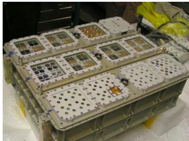
Expose allows long exposures to space conditions and solar UV-radiation on the International Space Station. Several trays filled with organisms were installed on the outside of the European Columbus laboratory as one of the nine payloads of the European Technology Exposure Facility (EuTEF). ESA image.
