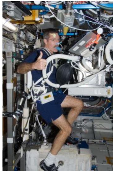
ISS030E007540 – View of astronaut Dan Burbank, Expedition 30 commander, using the Portable Pulmonary Function System (PPFS) hardware while exercising on the Cycle Ergometer with Vibration Isolation and Stabilization (CEVIS) in the U.S. Laboratory.
