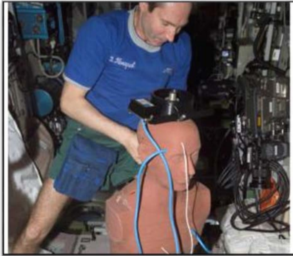
ISS012E22711 – Cosmonaut Valery I. Tokarev, Expedition 12 flight engineer works with the European Matroshka-R Phantom experiment in the Zvezda Service Module of the International Space Station.
