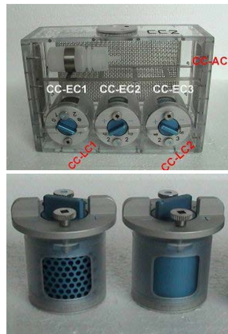
Top: 1 of the 2 Cricket Containers (CC), showing the adult compartment (CC-AC), the egg collectors (CC-EC), and hatching larvae compartments (CC-LC). Bottom: Egg collectors in open and closed configuration. ESA image.
