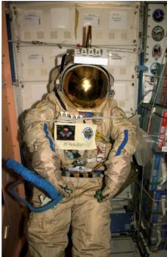
RadioSkaf created using a decommissioned Russian Orlan spacesuit that is outfitted with transmission hardware was released during an extravehicular activity. Roscosmos image.
