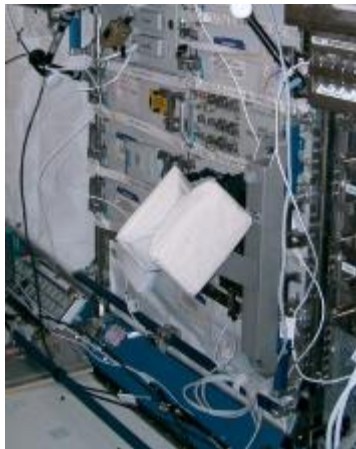
Left: Crew Restraint attached to the front of an International Space Station rack. Right: ESA astronaut Pedro Duque works on the Microgravity Science Glovebox while testing the new Crew Restraint device. ESA image.
