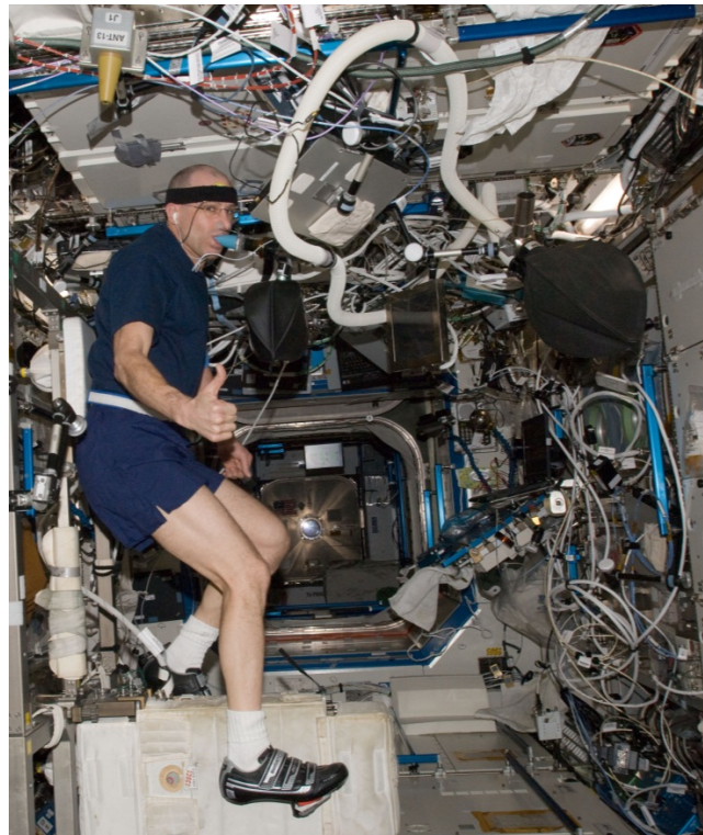
NASA astronaut Don Pettit, Expedition 30 flight engineer, performs a joint session of the European Space Agency's (ESA) Thermolab and Assessment of Endurance Capacity by Gas Exchange and Heart Rate Kinetics During Physical Training experiments in conjunction with NASA's VO 2 max experiment while using the Cycle Ergometer with Vibration Isolation System in the Destiny laboratory of the International Space Station. ESA/NASA image.
