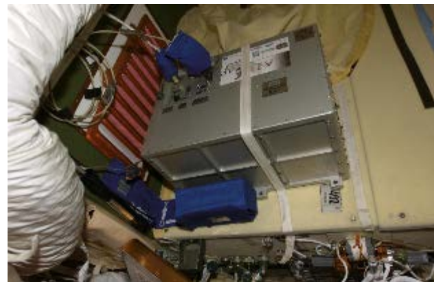
ISS010E24814 – Low Altitude Ionizing Observatory (LAZIO) in the Service Module 402/Zvezda during International Space Station (ISS) Expedition 10. LAZIO measures cosmic rays in space and their relation to anomalous phosphine (light flash) as perceived by crew members. Also studies the effect of different shielding materials to reducing the radiation environment and characterizes the magnetic environment inside the ISS. Hardware consists of a Main Electronics Box and Voice Recorder.
