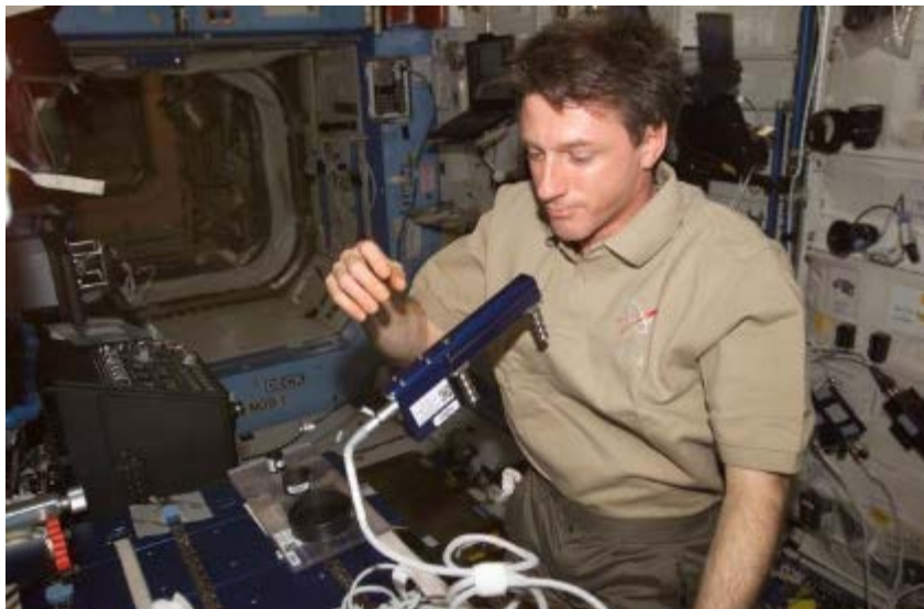
ISS008E21614 – International Space Station Science Officer Mike Foale performs the Hand Posture Analyzer investigation during Expedition 8, using the hand grip dynamometer to test the muscle fatigue of the forearm.
