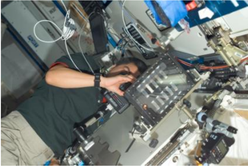
ISS016E027863 – Astronaut Dan Tani photographing the Binary Colloidal Alloy Test - 3 Sample Module using his own design for a ceiling mount in Node 2 of the International Space Station. Great high contrast pictures of difficult-to-capture images resulted from using this setup.
