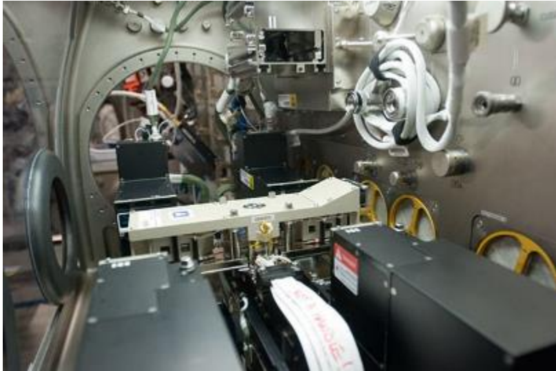
View of the Selectable Optical Diagnostics Instrument - Influence of Vibrations on Diffusion of Liquids investigation in the Microgravity Science Glovebox in the Columbus module of the International Space Station. NASA image.
