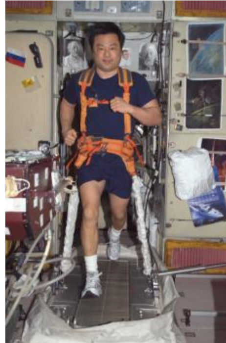
ISS010E24001 – Astronaut Leroy Chiao, Expedition 10 commander and NASA International Space Station (ISS) science officer, equipped with a bungee harness, exercises on the Treadmill Vibration Isolation System (TVIS) in the Zvezda Service Module of the ISS. Crew members completing standard exercise protocols on ISS are the experimental controls for the Mobility experiment.
