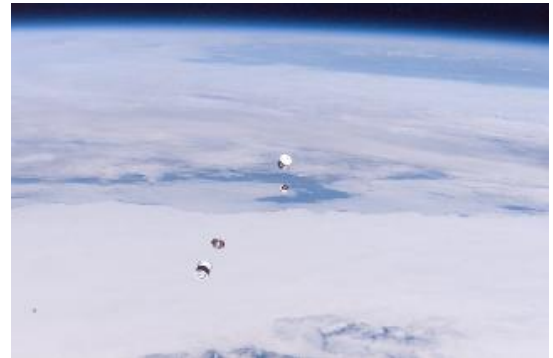
S116E07836 - Shown is one of the ANDE satellites floating free from Internal Cargo Unit (ICU) after deployment. The second satellite did not leave its half of the ICU until 4 hours after launch from the shuttle cargo bay.
