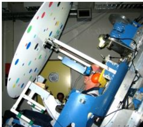
The Netherlands Organization for Applied Scientific Research (TNO) rotation chair combines vestibular stimuli (tilt and/or rotation) with visual stimuli (optic flow in roll). Used for addressing motion and attitude perception. ESA image.
