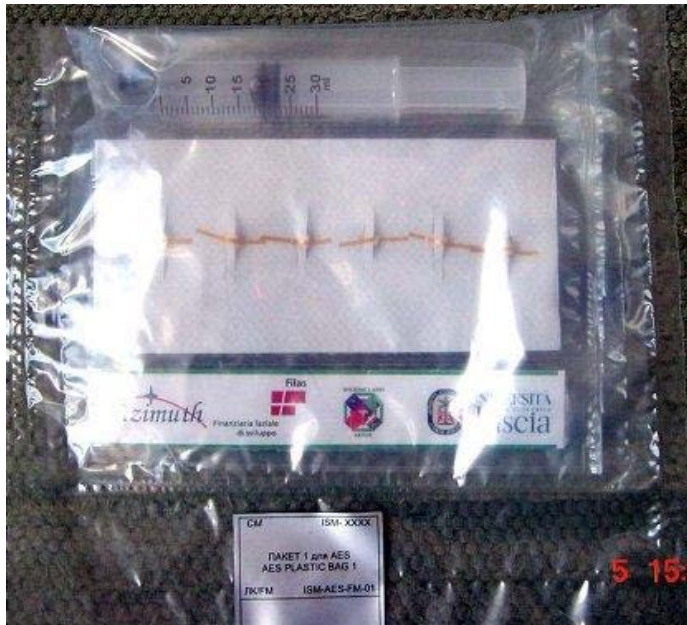
Space Beans for Students experiment. Plastic bag contains paper towel, seeds, and the water container. ESA image.
