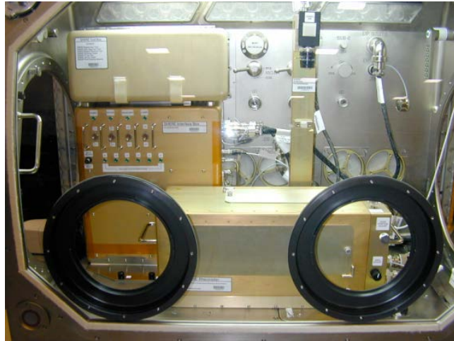
SHERE experimental hardware assembled in the Microgravity Science Glovebox (MSG) on the International Space Station (ISS). NASA's Glenn Research Center, Cleveland, Ohio image.
