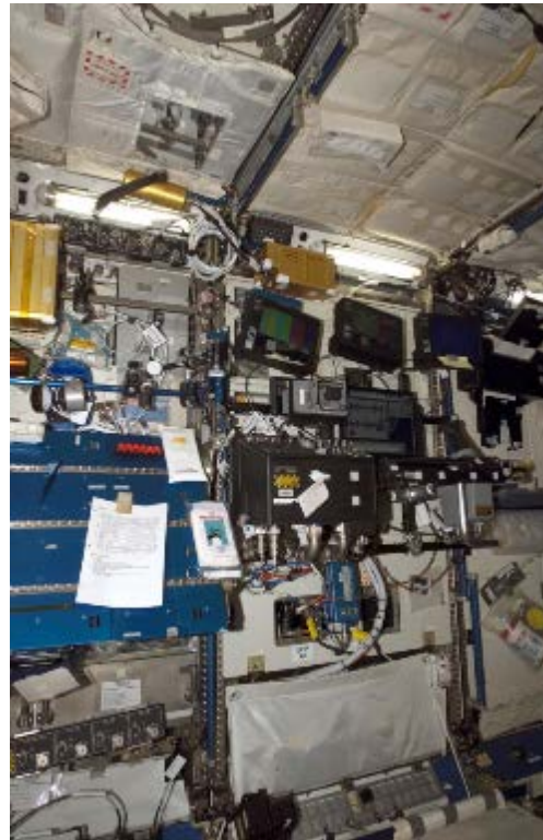
ISS015E12111 (June 15, 2007) – View of the Tissue Equivalent Proportional Counter (TEPC) Radiation Detector (gold cylinder) and the TEPC Spectrometer (gold box) in the US Laboratory/Destiny during Expedition 15. The TEPC monitors radiation doses at the cellular level.
