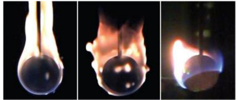
Zero-g facility test burning a 2 cm diameter PMMA sphere in 30 cm/s airflow. Left: 1 g; Middle: 0 g (1 s after drop); right: 0 g (4 s after application of nitrogen extinguishing agent). NASA image.
