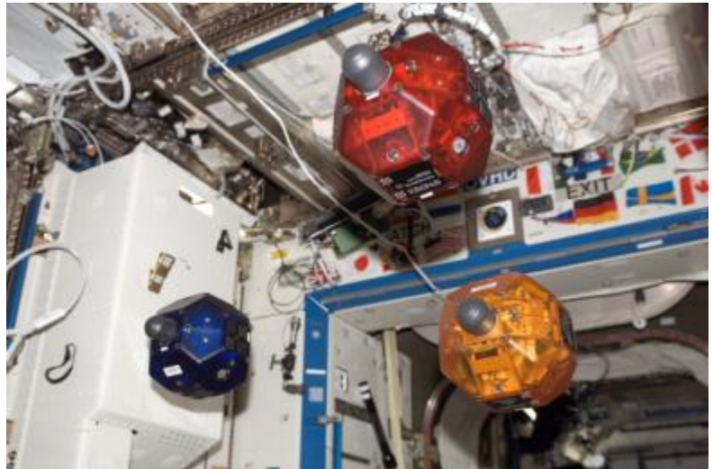
Three satellites fly in formation as part of the Synchronized Position Hold, Engage, Reorient, Experimental Satellites investigation.
