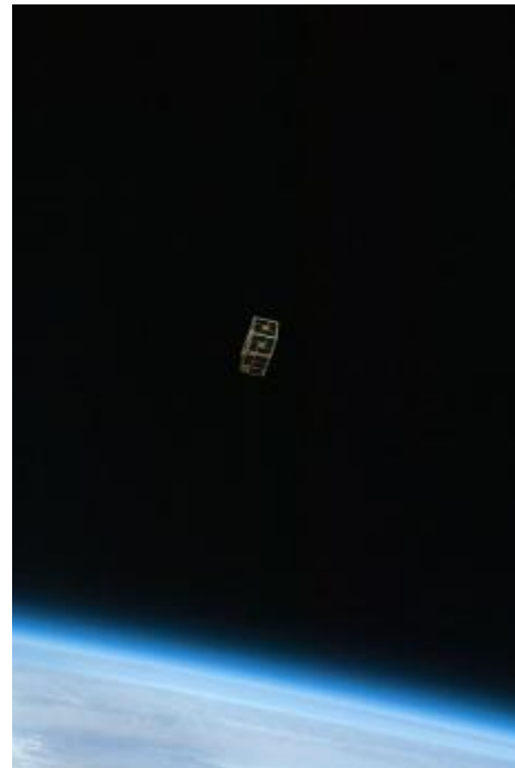
DRAGONSat looks at independent rendezvous of spacecraft in orbit using Global Positioning Satellite data.
