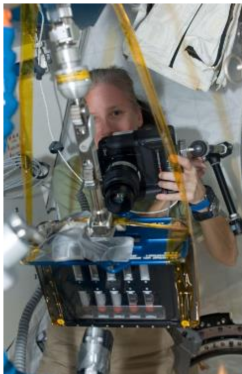
ISS025E008239 – NASA astronaut Shannon Walker, Expedition 25 flight engineer, uses a digital still camera to photograph Binary Colloidal Alloy Test-5 experiment samples in the Kibo laboratory of the International Space Station.
