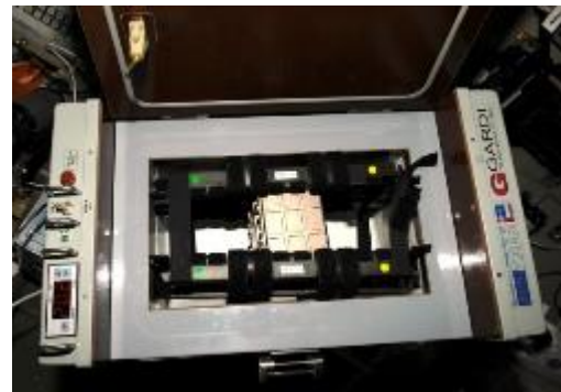
ISS014E20129 – A close-up view of the JAXA-Granada Crystallization Facilities (GCF) in the Thermo Biological Universal (TBU) during Expedition 14. JAXA image.
