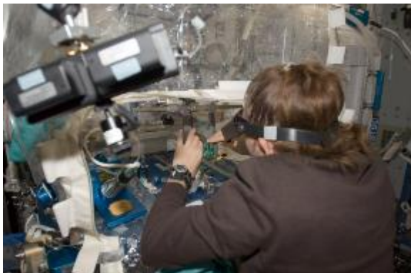
ISS018E035796 – Astronaut Sandra Magnus removing conformal coating during the CRE-1 experiment. NASA image.
