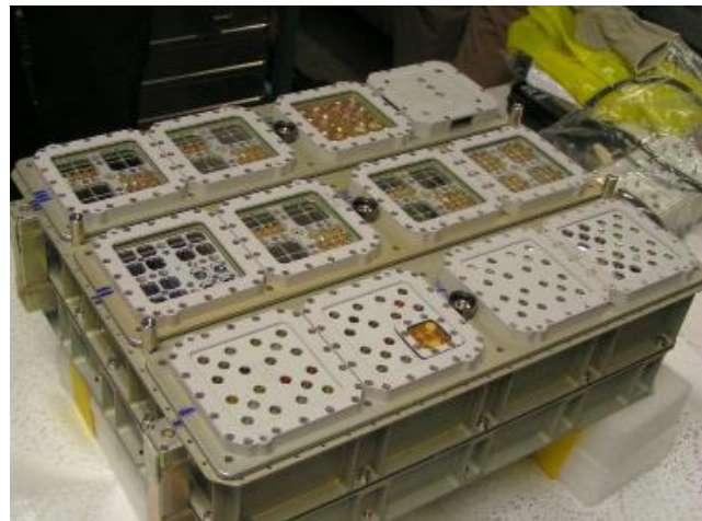
Expose allows long exposures to space conditions and solar UV-radiation on the International Space Station. Several trays filled with organisms were installed on the outside of the European Columbus laboratory as one of the 9 payloads of the European Technology Exposure Facility (EuTEF). ESA image.
