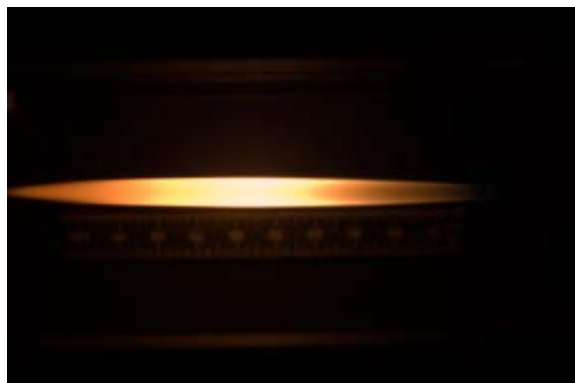
ISS018E030371 – View of the flame ignited in the SPICE (Smoke Point In Co-flow Experiment) payload performed in the MSG and controlled by its A31p with SPICE microdrives. Photo was taken by Expedition 18 crew.
