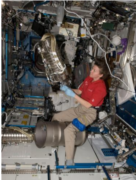
ISS026E014918 – NASA astronaut Catherine (Cady) Coleman, Expedition 26 flight engineer, removes the Low Gradient Furnace and installs the Solidification and Quench Furnace in the Material Science Laboratory in the Destiny laboratory of the International Space Station.
