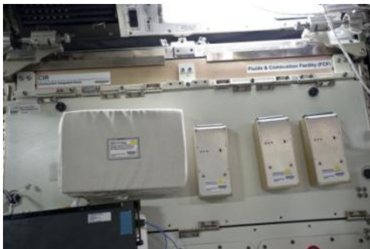
View of an I-ENOS bag and 3 I-ENOS sensors mounted to the Combustion Integrated Rack (CIR) in the US Laboratory/Destiny.
