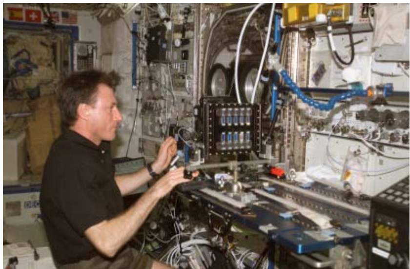
ISS008-E-20613 (April 5, 2004) – Astronaut C. Michael Foale, Expedition 8 commander and NASA International Space Station science officer, works with a Slow Growth Sample Module for the Binary Colloidal Alloy Test-3 experiment.
