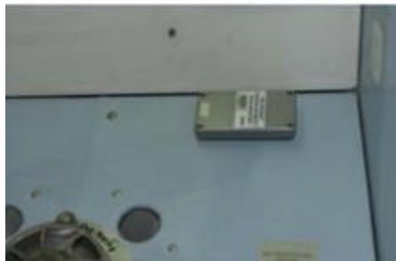
Placement of several Bradoz sets within the ISS RS compartments. Roscosmos image.
