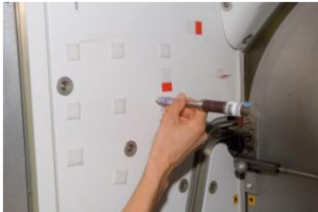
Expedition 14 Flight Engineer Suni Williams uses the swabbing unit to collect samples that will be placed into the cartridges to be analyzed by the Lab-on-a-Chip Application Development reader.
