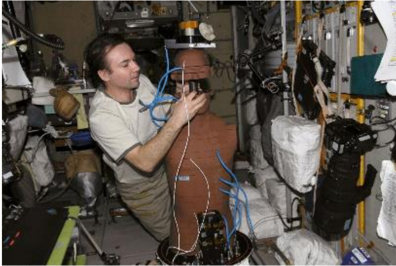
Cosmonaut Yury Lonchakov works with the European Matroshka Phantom experiment in the Zvezda Service Module of the International Space Station. Matroshka, the name for the traditional Russian set of nesting dolls, is an anthropomorphic model of a human torso designed for radiation studies. NASA image
