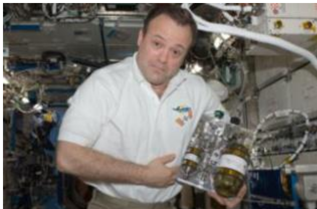
NASA astronaut Ron Garan prepares to install a Gas Supply Orbital Replacement Unit into the VCAM.
