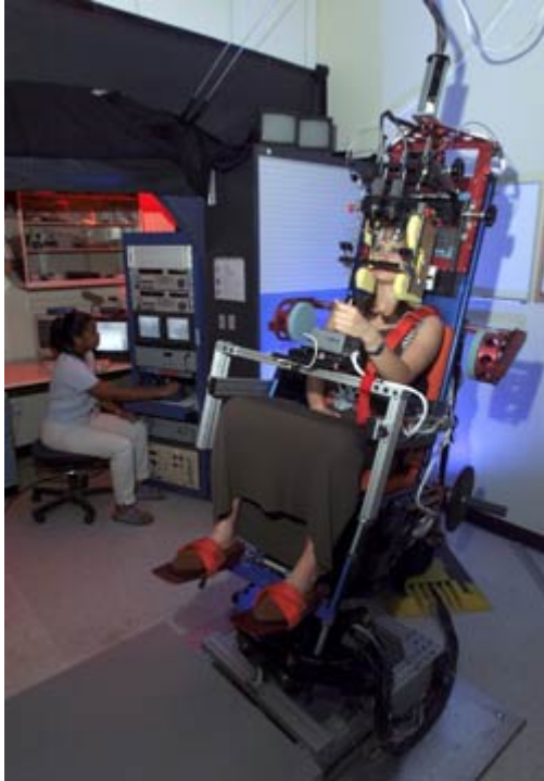
Off Vertical Rotation - Measurement of Perception and Video Recording of Eye Movements. ESA image.
