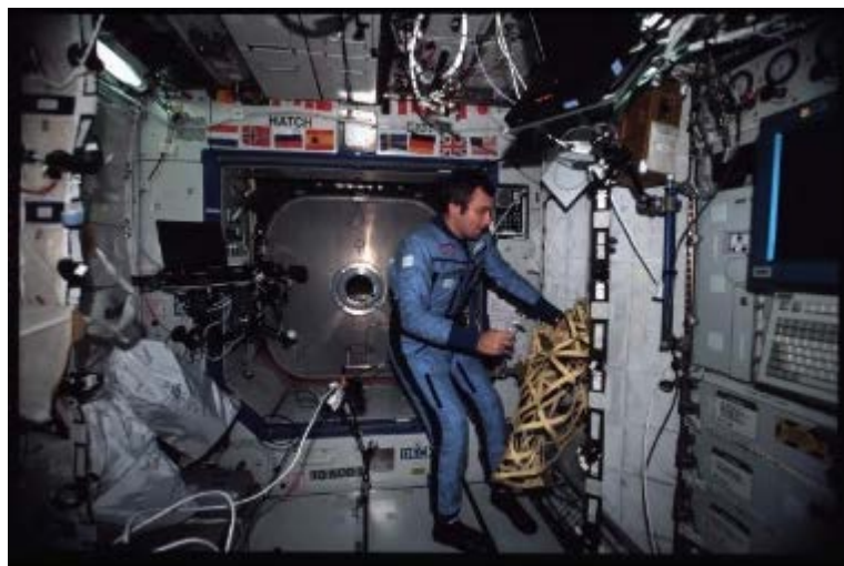
Cosmonaut Vladimir Dezhurov performs ARIS-ICE hammer tests in the US Destiny laboratory during Expedition 3.
