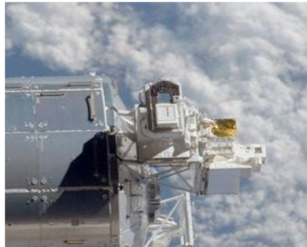
Sun monitoring on the External Payload Facility of Columbus – SOLAR Auto-Calibrating EUV/UV Spectrophotometers external facility mounted outside the Columbus module. ESA/NASA image.
