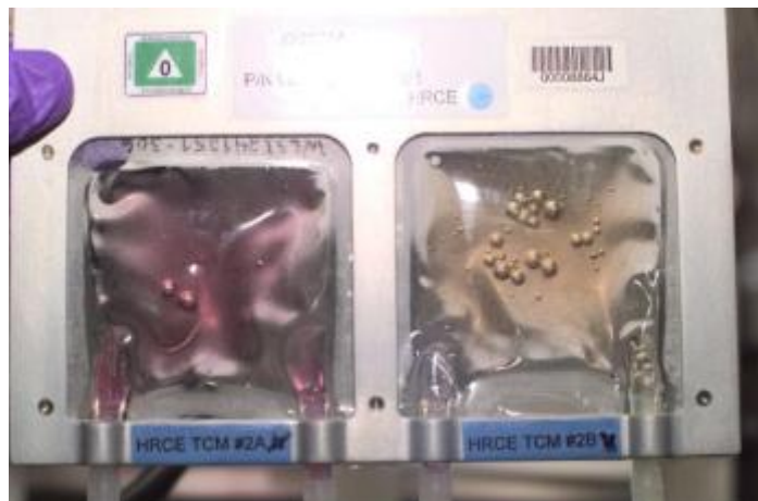
ISS0003E5276 – Image of a Quad Tissue Culture Module Assembly (QTCMA) 7 on International Space Station (ISS) Expedition 3 after activation of the cells. A syringe was used to inject cells into the pink nutrient growth media. The Biotechnology Specimen Temperature Controller (BSTC) can hold 8 of these QTCMAs, which are used to grow human cells on ISS. When the samples completed their growth cycle, the crew transferred the QTCMAs from the BSTC to the Biotechnology Refrigerator (BTR) where they were stored until they are examined at a ground-based laboratory.
