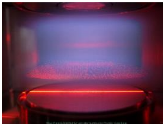
Side view of a plasma crystal in the laboratory. Dust particles are suspended in an argon plasma above a high-frequency electrode (bottom). The horizontal field of view is 2 cm. Max Planck Institute for Extraterrestrial Physics image.
