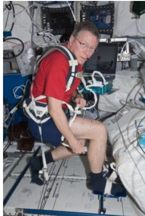
ISS029E036754 – NASA astronaut Mike Fossum, Expedition 29 commander, performs a SPRINT leg muscle self scan in the Columbus Laboratory of the International Space Station (ISS). Fossum powered on the Ultrasound 2 (USND-2) unit and Video Power Converter (VPC) hardware, and connected the VPC to Human Research Facility 1 (HRF-1) in order to perform this activity.
