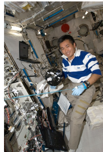
ISS018E044461 – Koichi Wakata installs a FACET cell in the Solution Crystallization Observation Facility (SCOF) during Expedition 18 aboard the International Space Station. JAXA image.
