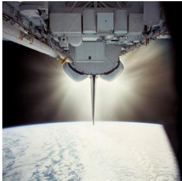
This image shows the Glow experiment documentation of Orbital Maneuvering System (OMS)/Reaction Control System (RCS) pods and vertical stabilizer from STS-007.
