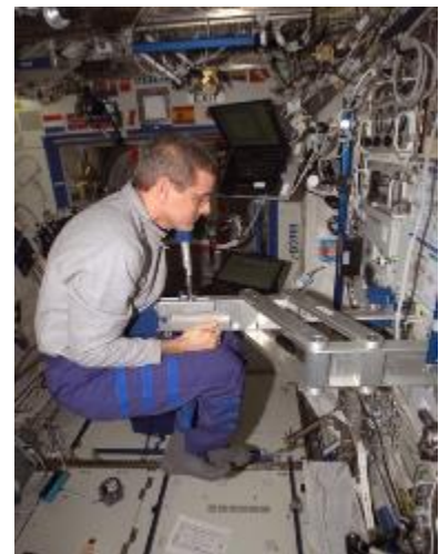
ISS012E12635 – International Space Station Science Officer Bill McArthur during expedition 12, during check-out of the SLAMMD hardware of HRF-2. Measuring the mass of a crew member in space is difficult because mass does not equal weight in the absence of gravity. NASA image.
