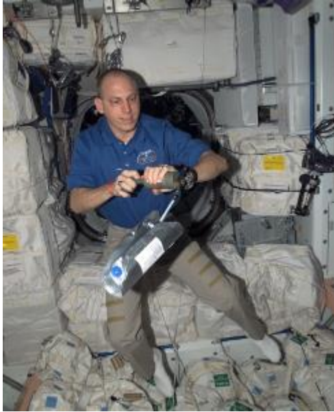
ISS015E32200 - Clay Anderson using the sampling pump and 2.5 liter gas sample bag for the ANITA experiment in the Node 1/Unitv.
