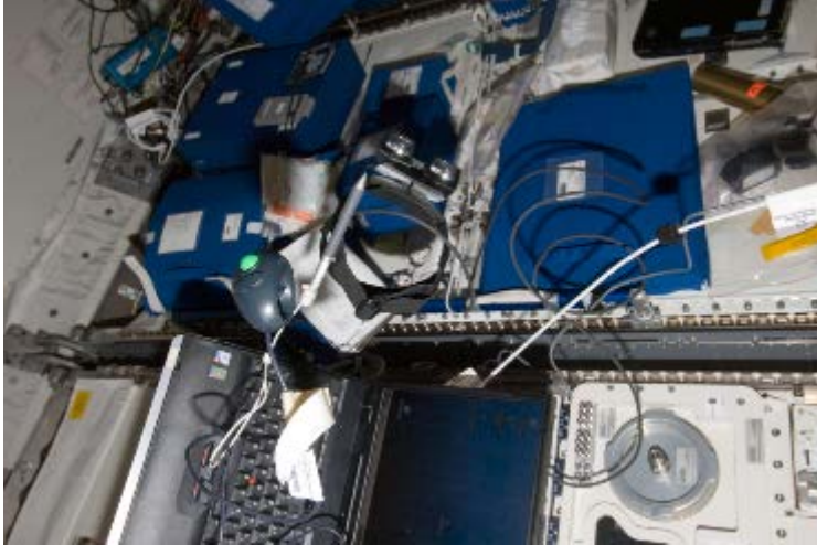
The European Space Agency Multipurpose Laptop with a prepared Hard Disk Drive, data storage on a PCMCIA memory card, and an electronic pen table connected to it to be used by the Expedition 20 crew during the French/CNES neuroscientific research experiment Mental Representation of Spatial Cues During Space Flight. NASA image.
