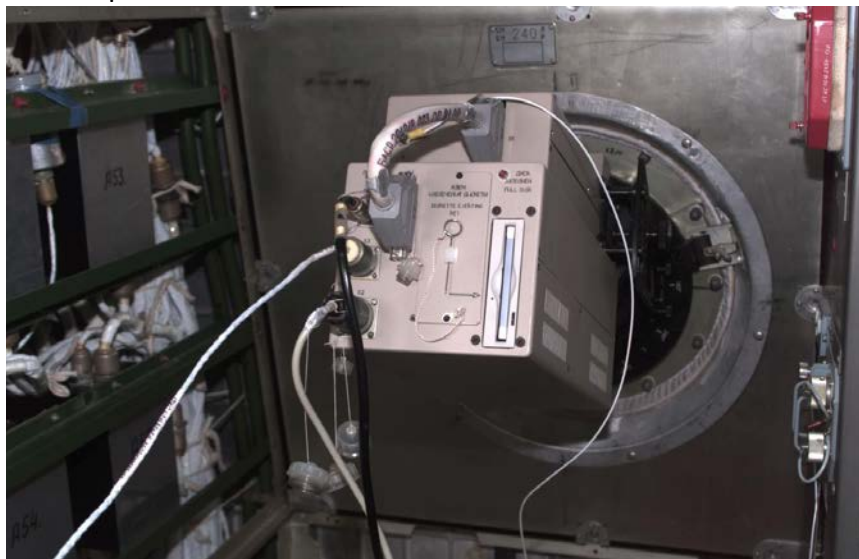
BΦC-3M Videophotometric Camera installed on a window in the ISS RS Service Module. Roscosmos image.
