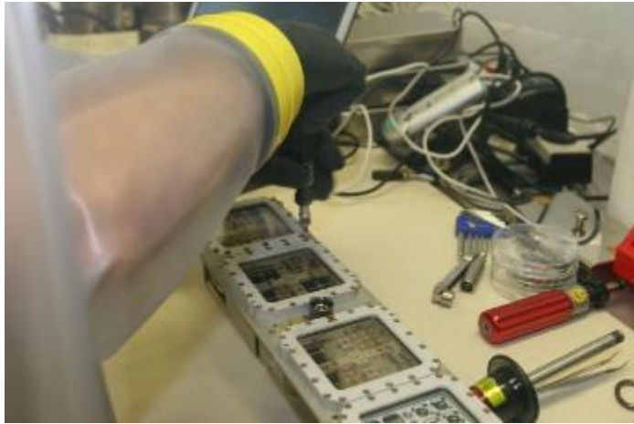
Sample containers are opened after they are returned to Earth for analysis. ESA image.
