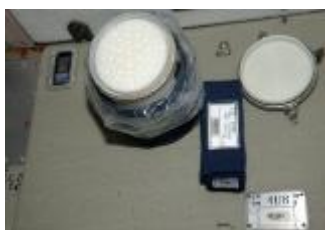
Ulitka container with the cover removed and the automatic temperature recorder on Panel #406 in the ISS RS SM. Roscosmos image
