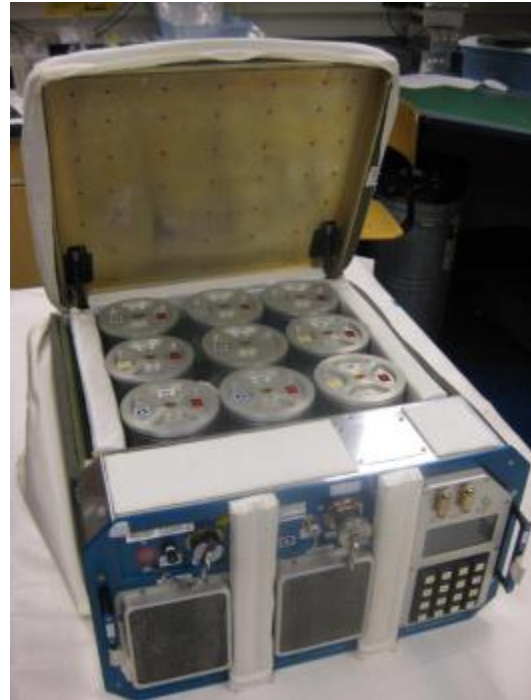
In this image shows the Group Activation Packs placed into the Commercial Generic Bioprocessing Apparatus that provides environmental controls from cold storage to incubation temperatures. BioServe Space Technologies image, University of Colorado, Boulder, Colorado.
