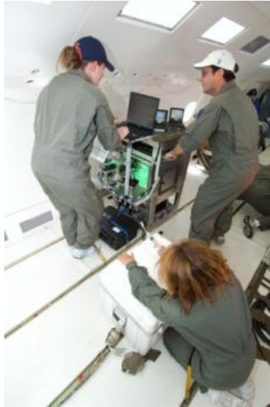
Glenn researchers test the effectiveness of an IV fluid mixing method on NASA's zero-gravity aircraft. NASA's Glenn Research Center image.
