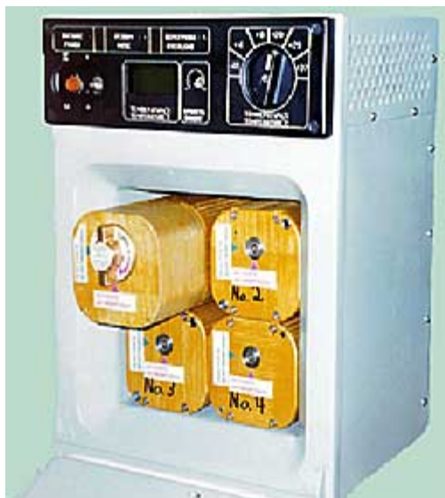
Freezer Kriogem-03 for storage of blood samples. ESA image.
