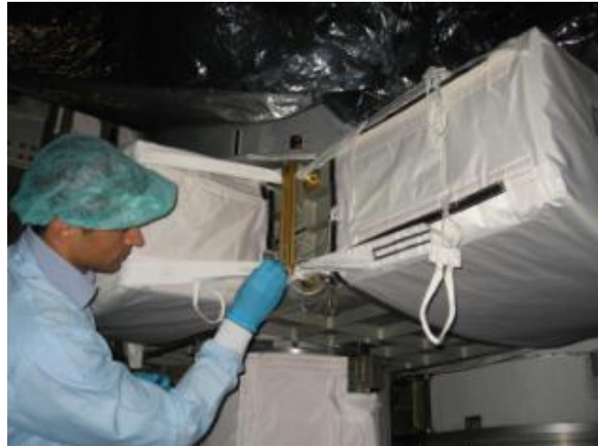
Lab-on-a-Chip Application Development-Portable Test System-Exploration principal investigator Jake Maule swabs a handrail of the S6 Truss.
