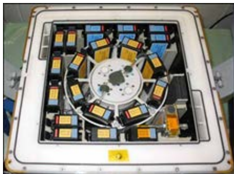
Example of Kubik incubator with centrifuge configuration loaded with experiment containers. ESA image.
