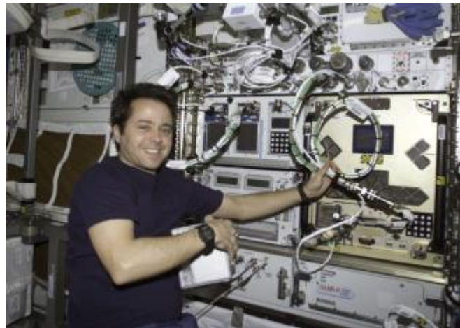
ISS004E11048 – The Commercial Generic Bioprocessing Apparatus isothermal containment module v.3, installed in Expedite the Processing of Experiments for Space Station rack just above astronaut Dan Bursch's extended left arm; photograph taken during Expedition 4.
