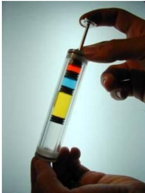
The Group Activation Pack - Fluid Processing Apparatus is essentially a microgravity test tube that allows controlled, sequential mixing of 2 or 3 fluids in a weightless environment. BioServe Space Technologies, University of Colorado - Boulder, Colorado image.
