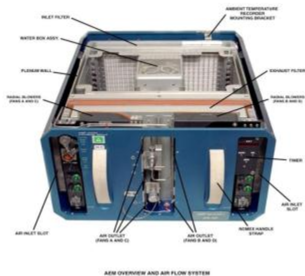
Image of the Animal Enclosure Module that houses the rodents used in the Mouse Immunology investigation. NASA's Ames Research Center image, Moffett Field, California.
