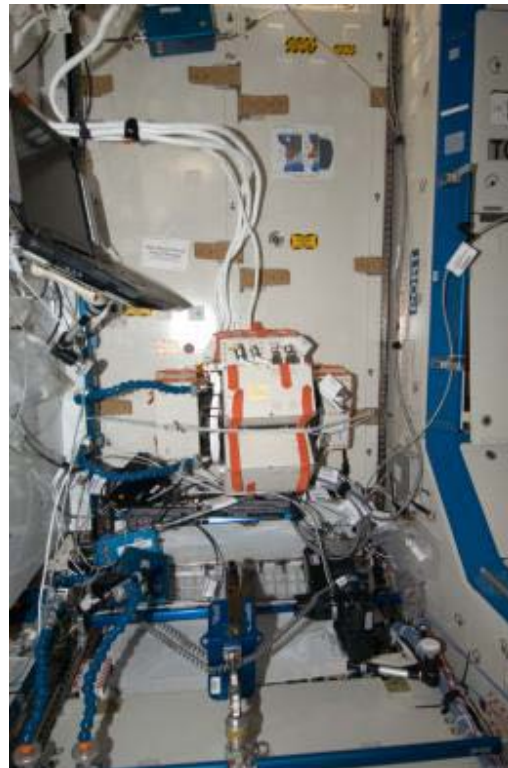
ISS019E005340 – View of the Anomalous Long Term Effects in Astronauts Central Nervous System (ALTEA) experiment and Silicon Detector Units designed to measure cosmic radiation passing through the brain. Photo taken in the U.S. Laboratory/Destiny during Expedition 19.
