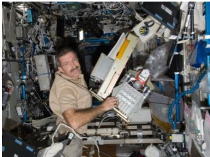
Expedition 30 Commander Dan Burbank assembles the Amine Swingbed Hardware Assembly in the US Laboratory/Destiny.
