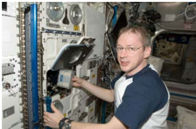
ISS020E044456 – Astronaut Frank De Winne, Expedition 20 flight engineer, works with the Yeast-B Part 2 experiment container in the Biolab incubator located in the Columbus module.
