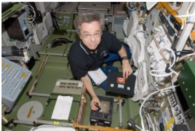
ISS020E050738 – Canadian Space Agency astronaut Robert Thirsk, Expedition 20/21 flight engineer, works with a Bubble dosimeter detector kit for the Matryoshka-R experiment in Service Module.
