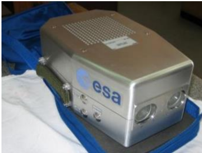
Erasmus Recording Binocular (ERB) 3-D video camera for use in the ERB experiment during Astrolab. The camera will be used to accurately map the interior of the International Space Station in its current configuration. These images will be used to improve the models available on the ground. ESA image.
