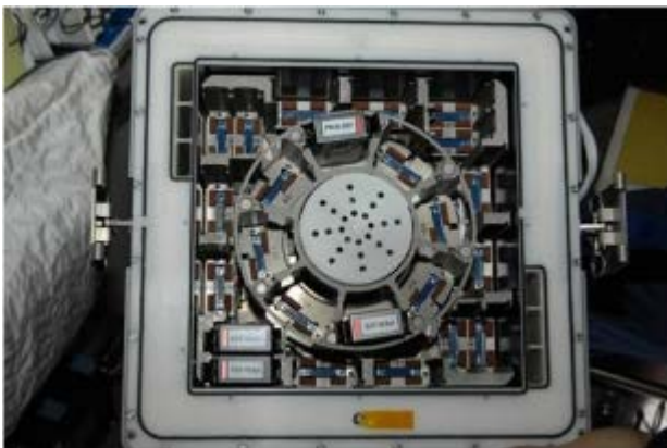
PKinase inside the transportable Kubik incubator. ESA image.
