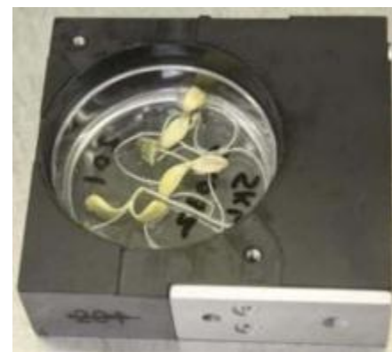
Medicago truncatula (barrel medic) seedlings grown inside a Biological Research In Canisters Petri Dish Fixation Unit. NASA image.
