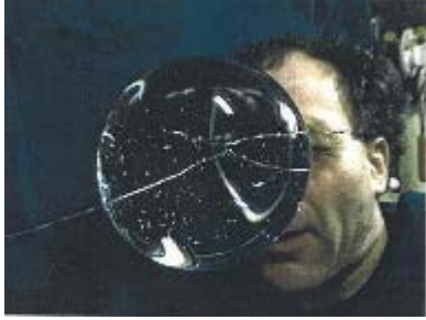
Video screen shot of a 13 cm free sphere of water stabilized by a wire loop aboard the International Space Station during Expedition 6. NASA image.
