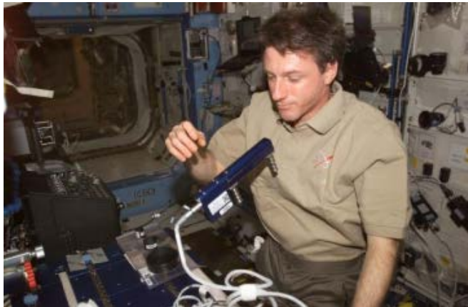
ISS008E21614 – ISS science officer Mike Foale is performing the HPA investigation during Expedition 8, using the hand grip dynamometer to test the muscle fatigue of the forearm.
