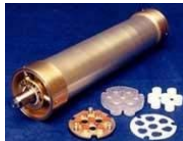
Protein Crystallization Apparatus for Microgravity (PCAM). NASA's Marshall Flight Space Center image.
