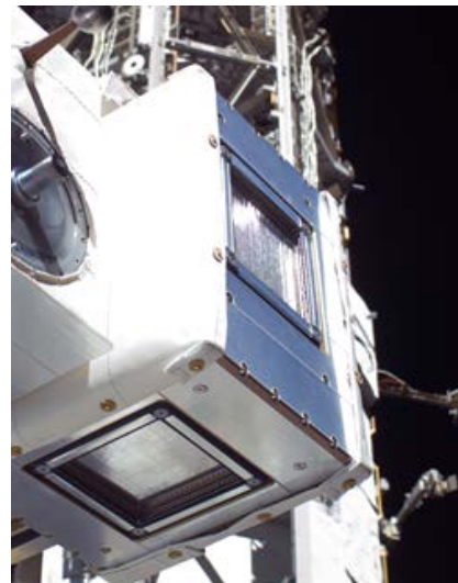
DEBris In Orbit Evaluator-2 instrument on the external surface of the Columbus laboratory as part of the European Technology Exposure Facility. ESA image.
