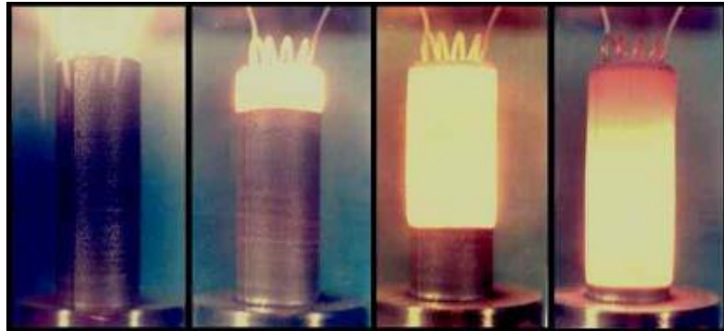
Snapshots of a combustion synthesis process, including the ignition stage and the movement of the combustion wave through the formed pellet. Institute of Structural Macrokinetics, Russian Academy of Sciences image.
