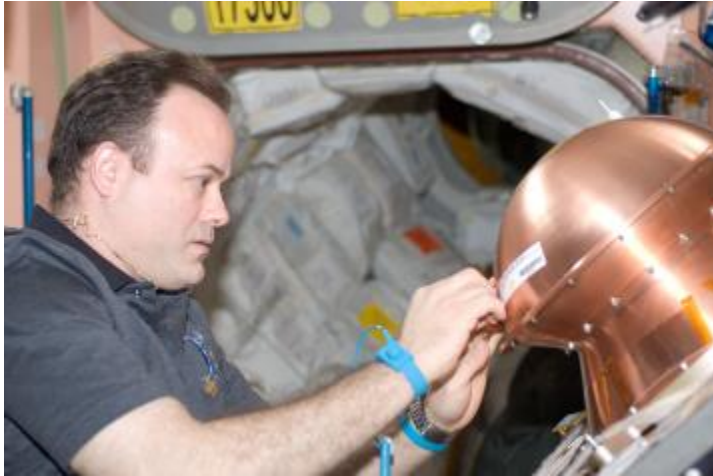
Expedition 28 Flight Engineer Ron Garan applies copper tape to exposed wires on the ReEntry Breakup Recorder prior to installation in the ATV-2.
