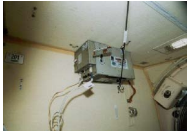
The Alteino apparatus is mounted inside the Pirs module aboard the International Space Station. ESA image
