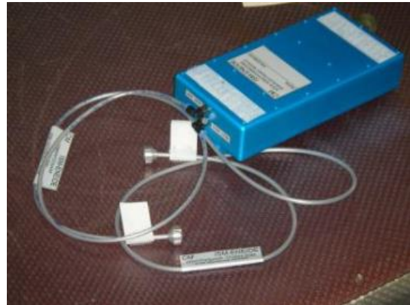
Electronic Nose Monitoring electronic module and probes. ESA image.
