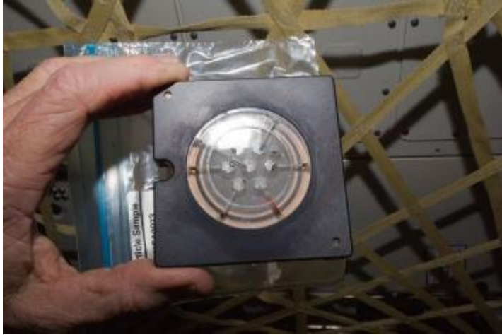
View of a Preliminary Advanced Colloids Experiment particle sample to be installed in the FIR/FCF.
