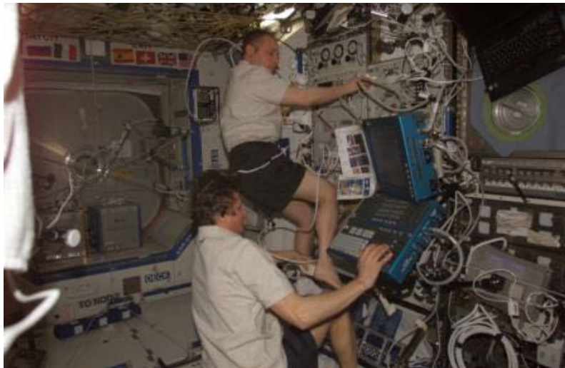
ISS009E17466 – Expedition 9 Commander Gennady Padalka performs an ultrasound bone scan on Flight Engineer and Science Officer Edward (Mike) Fincke's heel using the Advanced Diagnostic Ultrasound in Micro-G (ADUM) setup in the Destiny U.S. Laboratory Module. The ADUM keyboard, flat screen display, and front control panel are visible in the right field of view.
