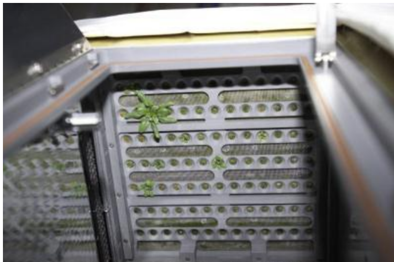
ISS004E8727 - Interior view of the Advanced Astroculture (ADVASC) experiment plant growth chamber showing the emergence of mustard seedlings. The ADVASC experiment is located in Expedite the Processing of Experiments to the Space Station rack 4 in the Destiny U.S. Laboratory during Expedition 4.
