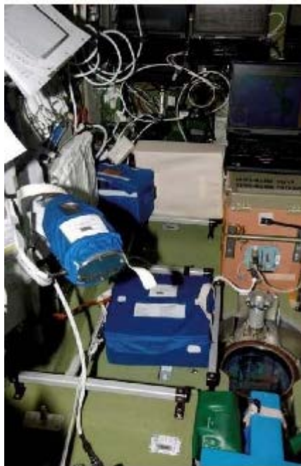
ISS012E24271 – The Planton Unit and Medical kits in the Zvezda Service Module. The Planton unit, Nitric Oxide Analyzer, used in the European Space Agency Nitric Oxide 1 experiment, is in the mid-left of the image. This image was taken during Expeditions 12/13 Joint Operations.
