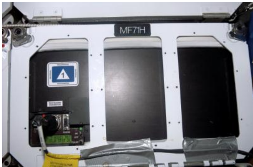
S118E10350 – Seen in this image is the hardware that houses the Cell Culture Module - Immune Response of Human Monocytes in Microgravity (CCM-Immune Response) and the Cell Culture Module - Effect of Microgravity on Wound Repair: In Vitro Model of New Blood Vessel Development (CCM-Wound Repair) experiments. The experiments were flown on STS118/13A August 1, 2007.
