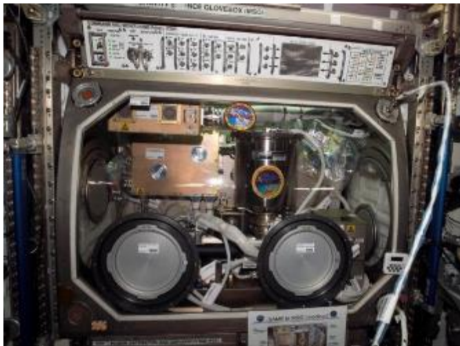
ISS015E26265 – View of Smoke and Aerosol Measurement Experiment (SAME) hardware in the Microgravity Science Glovebox (MSG) in the US Laboratory/Destiny. SAME aims to test the performance of ionization smoke detectors and evaluate the performance of the photoelectric smoke detectors.
