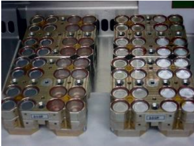
Flight sample carrier of experiments ADAPT and PROTECT after de-integration. DLR image.
