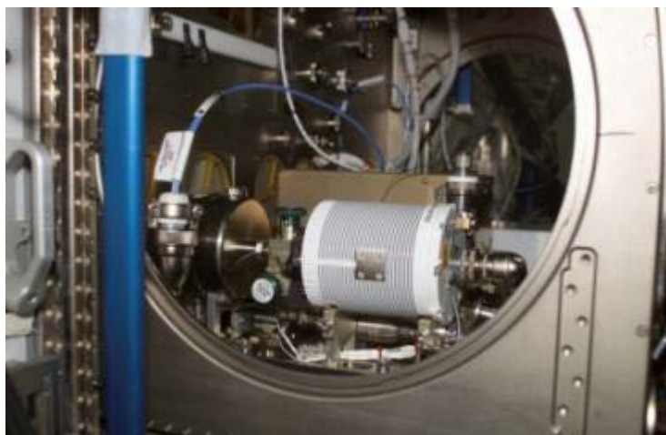
ISS007E10467 – Side view of the sample chamber portion of the Coarsening in Solid/Liquid Mixtures-2 experiment installed in the Microgravity Science Glovebox (MSG) of the Destiny Laboratory module. Also visible are cables attaching the hardware to the MSG and a vacuum valve knob.
