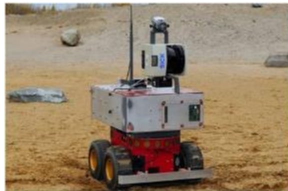
Red uses a laser to scan the terrain and provide 3-D images. Canadian Space Agency image.
