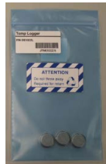
Transport Environment Monitor is composed of 3 commercial, small temperature loggers. JAXA image.
