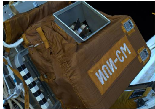
General View of the Pulsed Plasma Injector with Electro-physical Parameter Monitoring System Sensors on the ISS. Roscosmos image.
