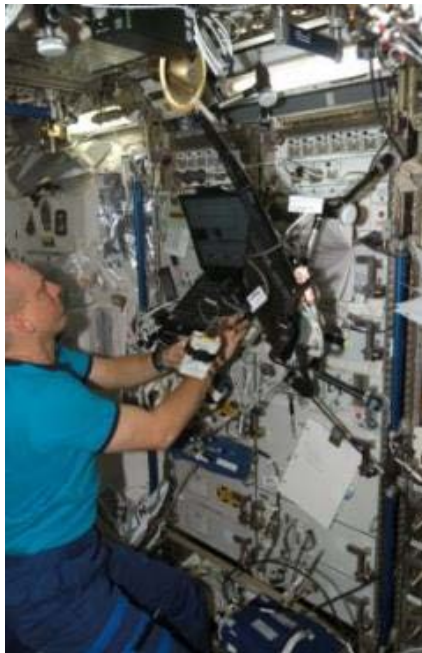
ISS015E14753 – View of Expedition 15 astronaut and flight engineer Clayton Anderson working with a Continuous Blood Pressure Device (CBPD) and computer during hardware set-up for the Cardiovascular and Cerebrovascular Control on Return from the International Space Station (CCISS) experiment in the U.S. Laboratory/Destiny.
