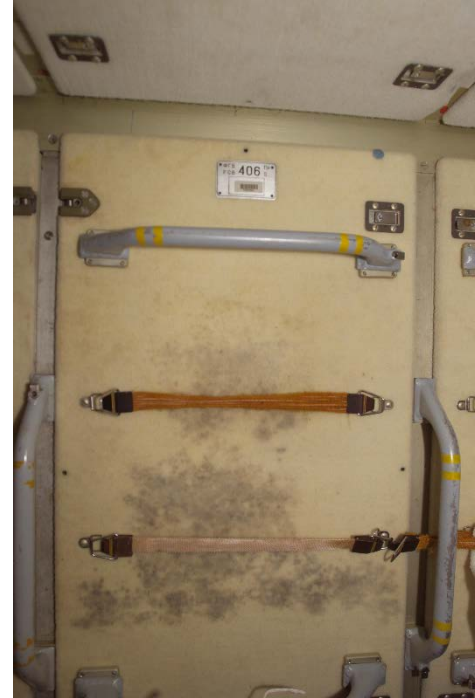
ISS010E11563 - An example of contamination that has developed on one of the interior panels aboard ISS. This image shows how contamination can form on interior ISS surfaces. Crews have weekly sessions to clean ISS surfaces. SWAB will help us understand the microbes involved in contamination and how to deal with them.
