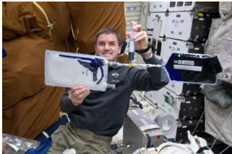
Mission specialist Rex Walheim uses the Forward Osmosis Pump Syringe to inject the Challenge Liquid into the FOB during STS-135/ULF7.
