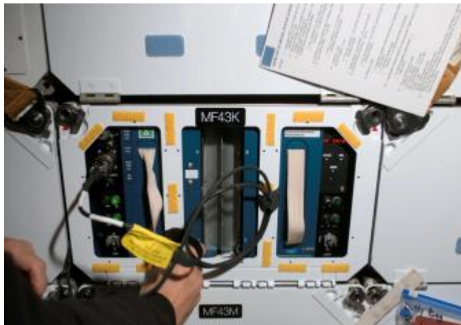
S118E09308 – The Commercial Biomedical Test Module - 2 (CBTM-2) hardware seen in this image flew onboard STS-118/13A.1 in August 2007. CBTM-2 tests the effectiveness of an experimental therapeutic as a possible countermeasure for muscle atrophy.
