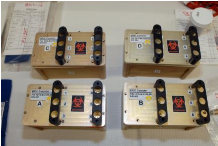
Image of Biological Research in Canisters (BRIC) - 16 middeck payload hardware and final packing of locker MR28K. BRIC Canister A-D, only A is fully assembled. NASA image.
