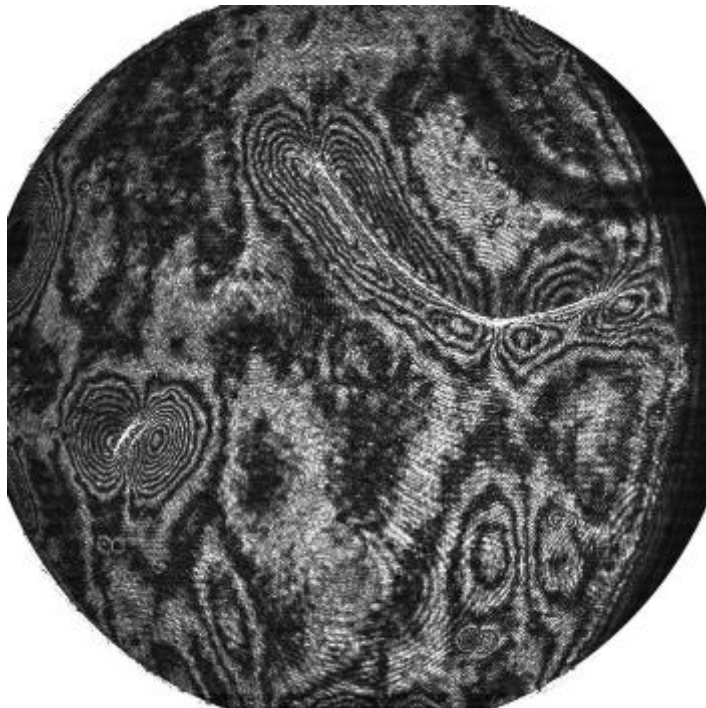
Geoflow-II image showing plume-like thermal upwellings. ESA image.
