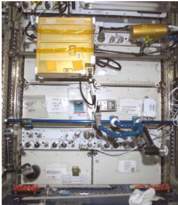
ISS009E06471 – EXPRESS Rack 5 with the Intravehicular Charged Particle Directional Spectrometer (IV-CPDS) (gold box in left field of view) and the Tissue Equivalent Proportional Counter Radiation Detector (gold cylinder) and upper storage compartments visible. EXPRESS Rack 5 is in the Destiny module/U. laboratory. NASA image.
