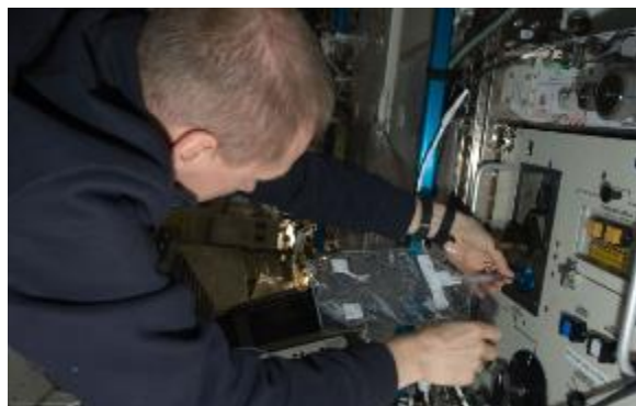
ISS021E010366 – Expedition 21 Commander Frank De Winne fills a bag with water from the Potable Water Dispenser in the US Laboratory/Destiny for analysis. NASA image.
