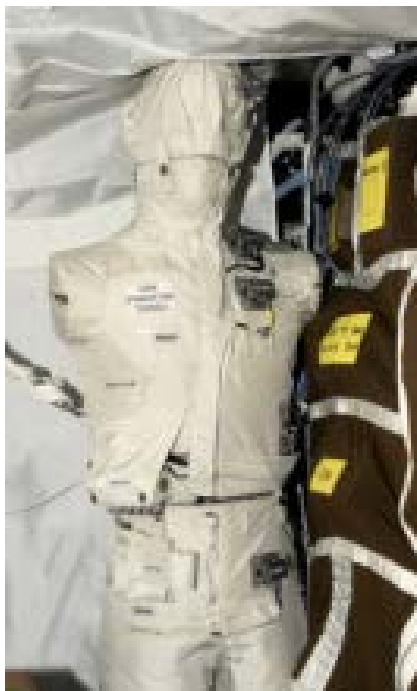
ISS002E6080 – The Phantom Torso, seen here in the Human Research Facility (HRF) section of the Destiny/U.S. Laboratory on the International Space Station (ISS), is designed to measure the effects of radiation on organs inside the body by using a torso that is similar to those used to train radiologists on Earth. The torso is equivalent in height and weight to an average adult male.
