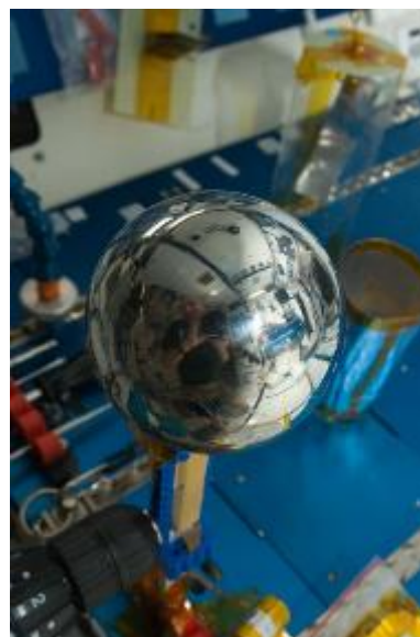
ISS031E035391 – Close-up view of a 4 inch polished metal sphere used to construct a Van de Graaff generator, along with Lego bricks, a rubber band, aluminum foil, and a drill. The image of Expedition 31 flight engineer Don Pettit is reflected in the sphere. Image was taken in the Harmony Node 2 during Expedition 31. NASA image.
