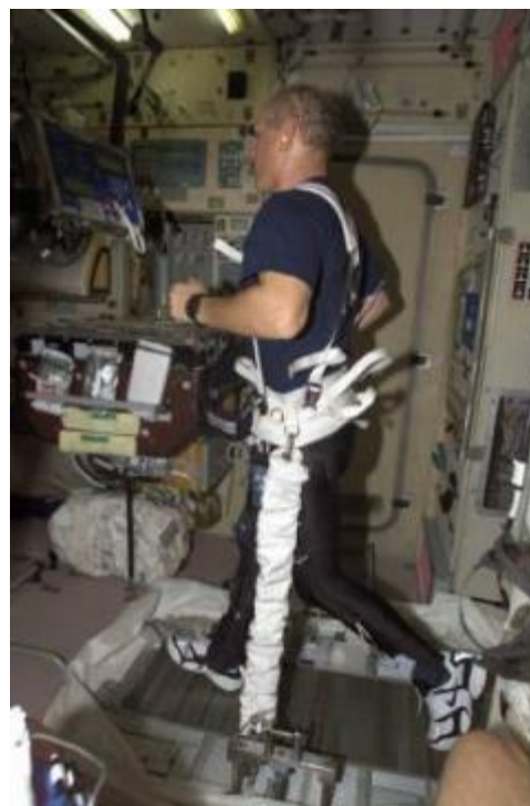
ISS006E11018 – Expedition 6 Mission Commander Kenneth Bowersox, wearing a body harness, runs on the Treadmill Vibration Isolation System (TVIS) while conducting the Foot/Ground Reaction Forces During Spaceflight (Foot) experiment in the Zvezda/Service Module.
