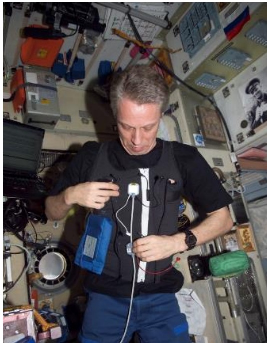
ESA astronaut Thomas Reiter wears the Cardiac Adapted Sleep Parameters Electrocardiogram Recorder vest right before going to sleep. ESA image.
