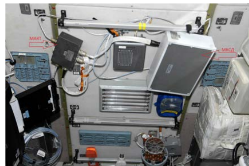
Gamma sensor monitoring module and control and data acquisition module from the Foton-Gamma payload set up on one of the panels in the ISS RS Service module. Roscosmos image.
