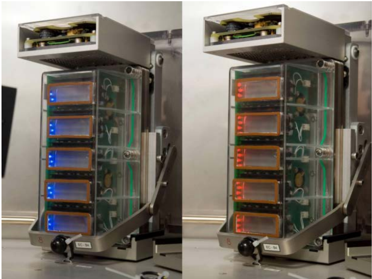
European Modular Cultivation System (EMCS) Tropi experiment unique equipment (EUE) shown stimulating Arabidopsis seedlings with blue light (left). EMCS Tropi EUE shown stimulating Arabidopsis seedlings with red light (right). Ames Research Center, Moffett Field, California image.
