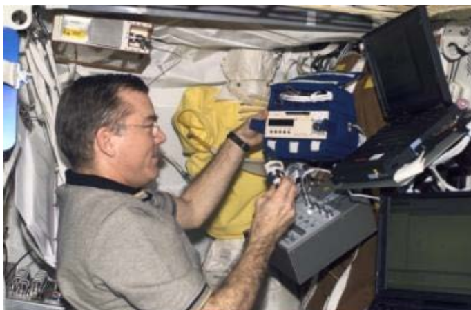
ISS002E7814 (June 26, 2001) - James S. Voss, Expedition Two flight engineer, sets up the Human Research Facility's (HRF) Dosimetric Mapping (DOSMAP) Power Distribution Unit (PDU) in Destiny.
