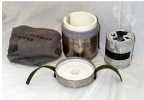
Container KB-03 for returning urine and blood samples. Roscosmos image.
