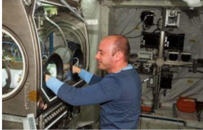
ISS016E036416 – Expedition 17 Flight Engineer Garrett Reisman works with the Coarsening in Solid Liquid Mixtures-2 (CSLM-2) experiment in the Microgravity Sciences Glovebox. Image was taken in the European Laboratory/Columbus Module during Expedition 16 / Expedition 17 joint operations.
