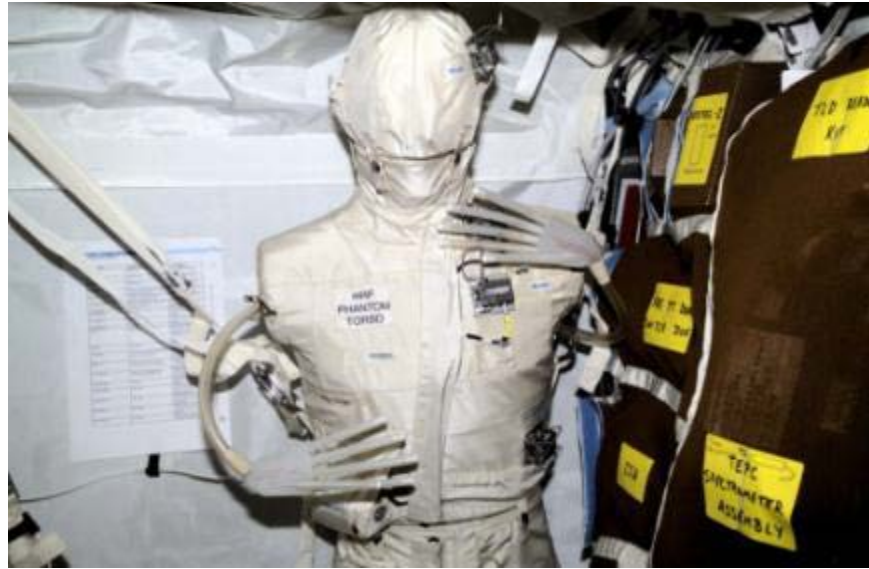
ISS002E5952 – The Phantom Torso, seen here in the Destiny laboratory on the International Space Station (ISS), is designed to measure the effects of radiation on organs inside the body by using a torso that is similar to those used to train radiologists on Earth. The torso is equivalent in height and weight to an average adult male. It contains radiation detectors that will measure, in real-time, how much radiation the brain, thyroid, stomach, colon, and heart and lung area receive on a daily basis.
