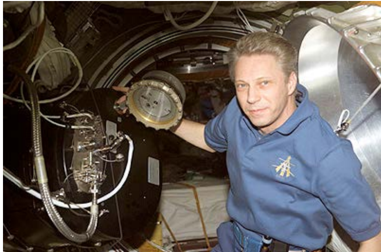
German ESA astronaut Thomas Reiter aboard the International Space Station with the PK-3 Plus laboratory. The Experiment Container is mounted in the Service Module. NASA image.
