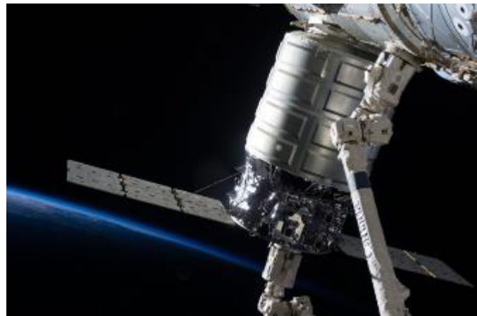
ISS037E006296 – The first Cygnus commercial cargo spacecraft built by Orbital Sciences Corp., seen here attached to the International Space Station's Harmony node. NASA image.
