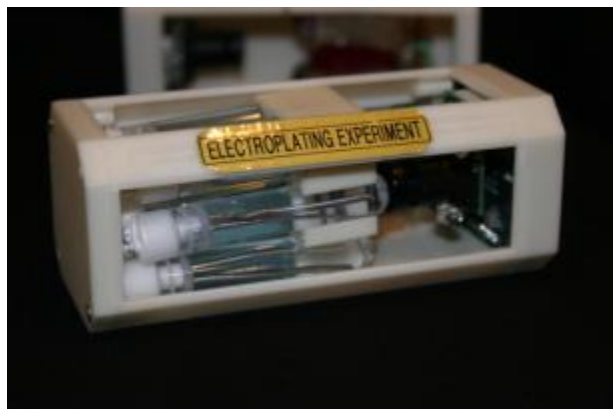
NanoRacks-Valley Christian High School-Electroplating Experiment Ground Test Unit. Valley Christian High School image.
