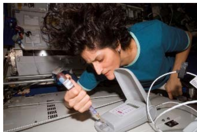
ISS014E18822 – Astronaut Suni Williams, Expedition 14 flight engineer, works with the Lab-on-a-Chip Application Development-Portable Test System (LOCAD-PTS). Williams is placing the sample mixed with water from the swabbing unit into the LOCAD-PTS cartridge. NASA image.
