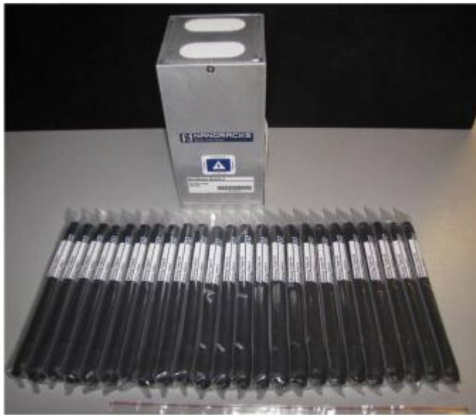
NanoRacks-Terpene Extraction in Microgravity MixStix contain a dry wood sample and a 50/50 mixture of water and ethanol. Image courtesy of NanoRacks, LLC.
