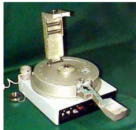
Centrifuge Plasma-03 to separate blood into plasma and serum. ESA image.
