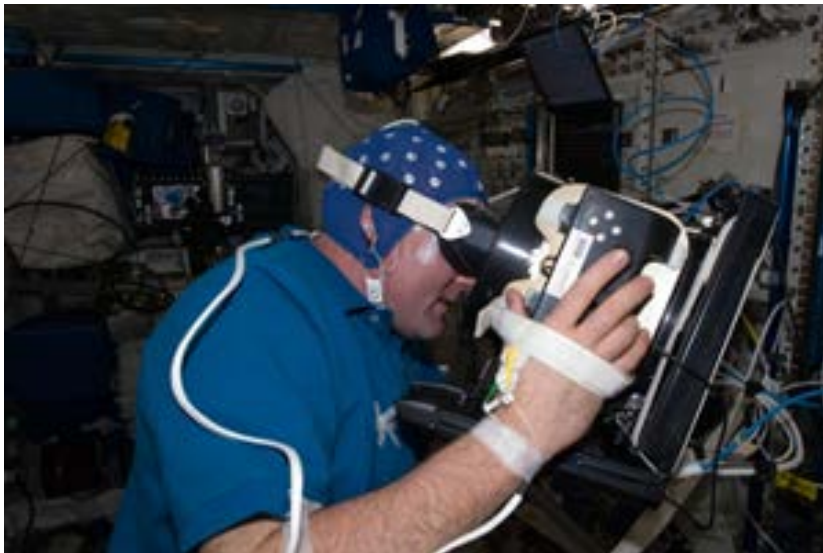
ESA's Andre Kuipers performs his first orbital the Effect of Gravitational Context on EEG Dynamics: A Study of Spatial Cognition, Novelty Processing and Sensorimotor Integration session. Andre is wearing an Electroencephalogram electrode cap and optimizing channel impedance of the electrodes before starting measurements. NASA image.
