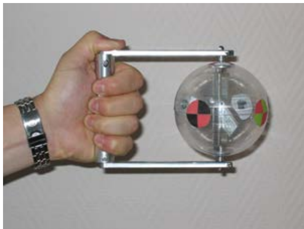
Analysis of Inertial Solid Properties experimental configuration. ESA image.
