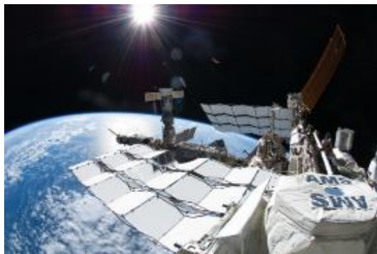
S134E007193, ISS028E016135 - Alpha Magnetic Spectrometer mounted on the S3 truss.
