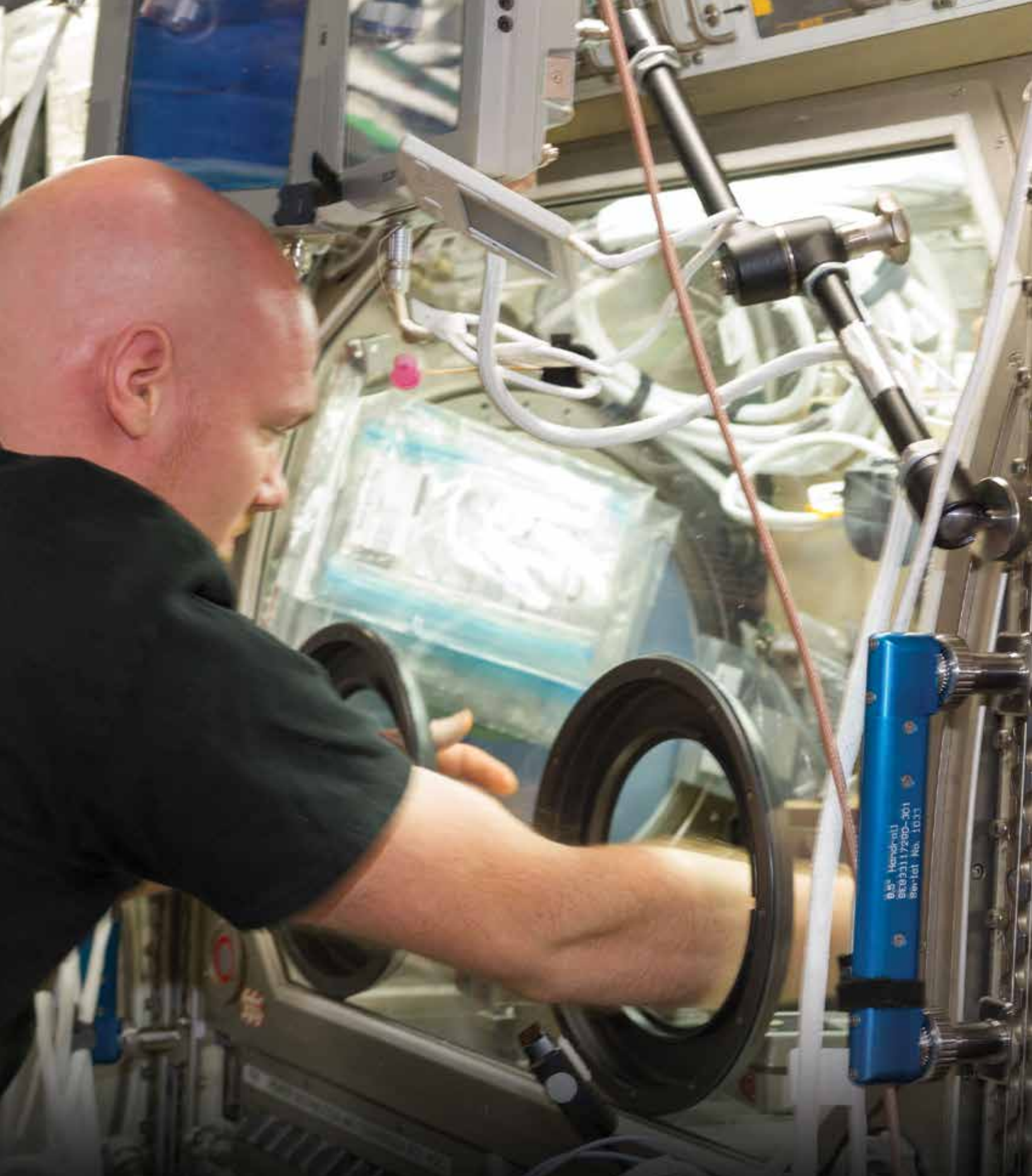
European Space Agency astronaut Alexander Gerst, Expedition 40 flight engineer, performs two tests with a combustion experiment known as the Burning and Suppression of Solids (BASS-II) in the Microgravity Science Glovebox (MSG) in the Destiny laboratory of the International Space Station (ISS040E083576).
