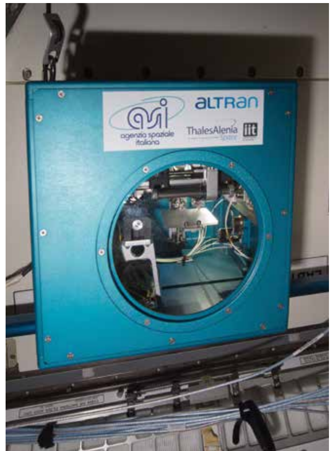
Fabrication of the test object in the Portable on-Orbit 3D Printer (ISS046E031502).
