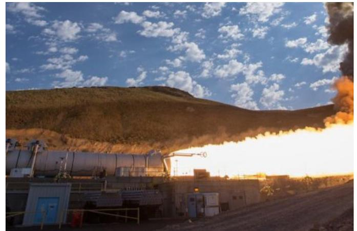
NASA and Northrop Grumman have successfully completed three full-scale development and two full-scale qualification test firings of the five-segment solid rocket motor, as well as the important booster critical design review.
