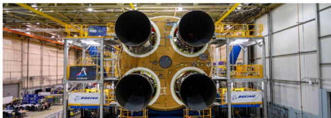
Four RS-25 engines attached to the core stage for Artemis I
