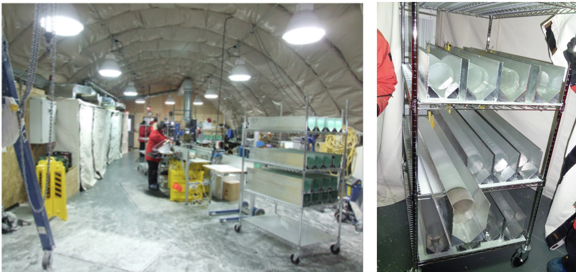
Figure II-8. West Antarctic Ice Sheet (WAIS) Divide drill site. Left: On site freezer units that keep ice at -26C. Right: Core sections in core trays, where the core diameter is 122 mm (4.8 inches).
