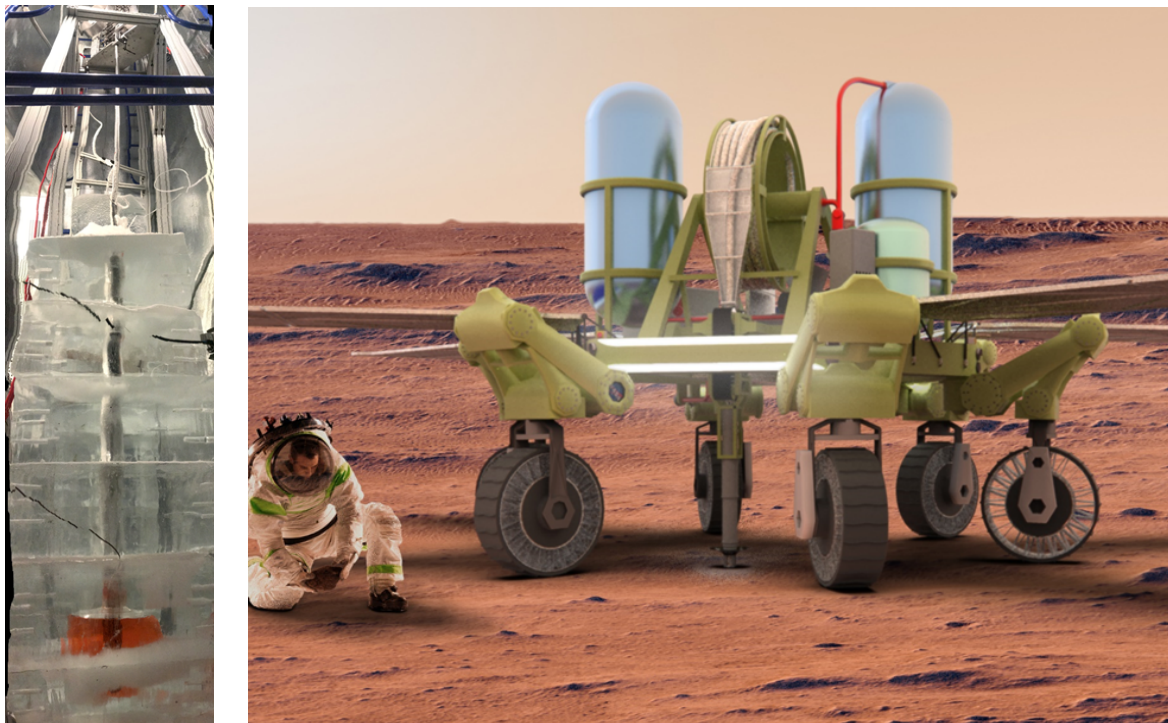
Figure IV-8. Left: Coiled Tubing drill, RedWater, being tested in a freezer. Right: RedWater implementation on NASA All-Terrain Hex-Limbed Extra-Terrestrial Explorer (ATHLETE) rover.
