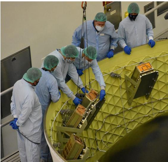
All 10 secondary payloads have been installed in the Space Launch System (SLS) rocket's Orion stage adapter. The Orion stage adapter connects the SLS rocket to Orion and had slots built into it for the payloads.
