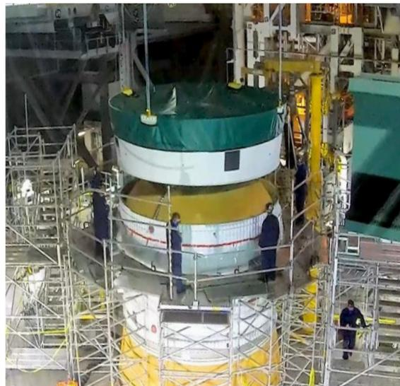
Teams from Exploration Ground Systems mate the Orion Stage Adapter (OSA) to the Interim Cryogenic Propulsion Stage (ICPS) on top of the Space Launch System.
