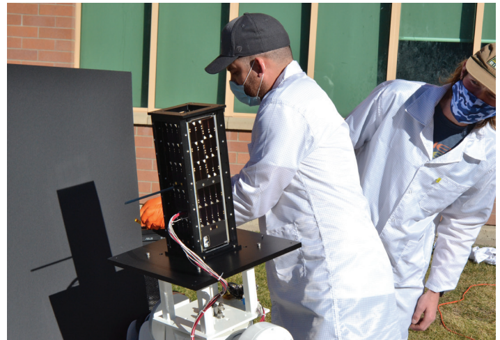
Solar array balance testing at MSU. Rubin Meuchel (L), Nevin Leh(R).
