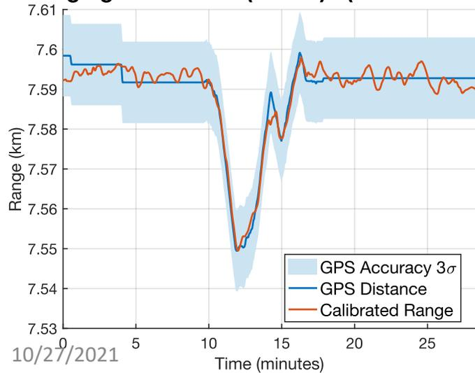
**Ranging Calibration (B to E) (RMS = 3.3418m)**
