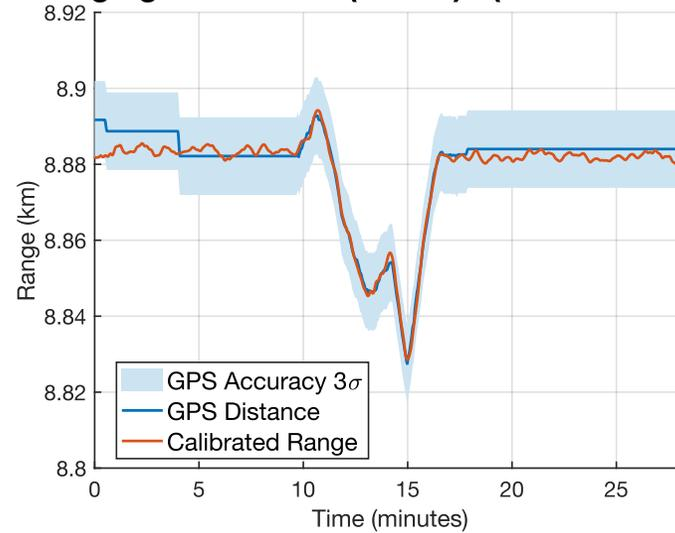
**Ranging Calibration (D to B) (RMS = 2.3012m)**
