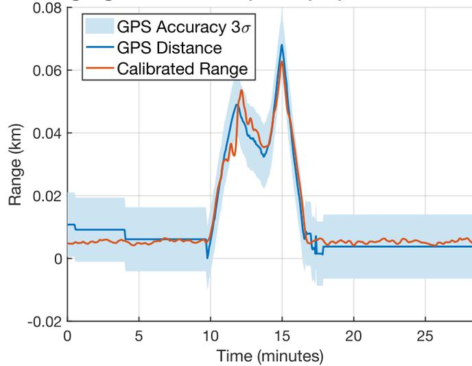
**Ranging Calibration (C to B) (RMS = 2.4388m)**
