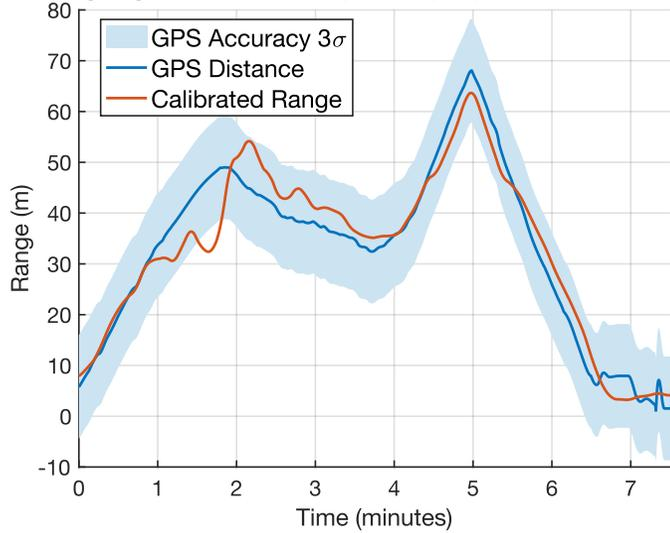
**Ranging Calibration (C to B) (RMS = 1.1204m)**
