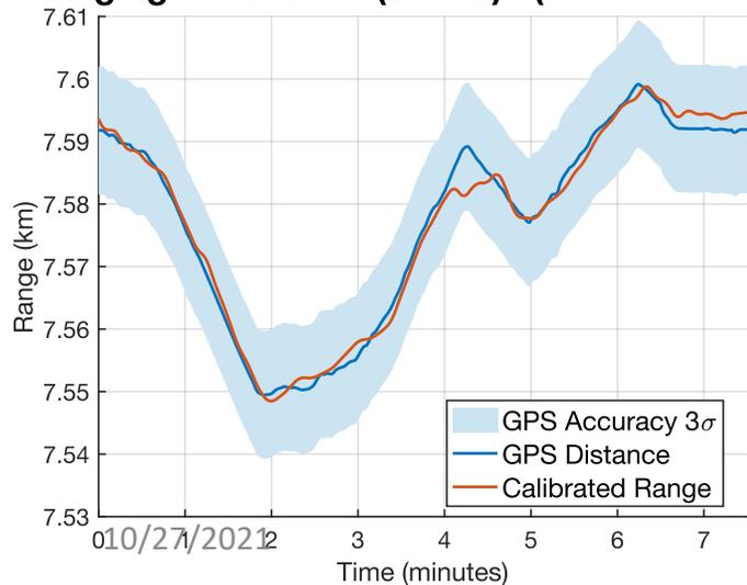
**Ranging Calibration (B to E) (RMS = 3.6266m)**
