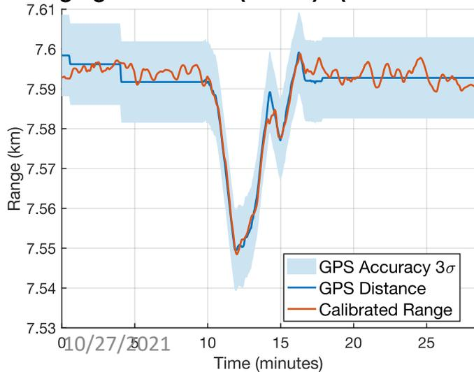
**Ranging Calibration (B to E) (RMS = 3.851m)**
