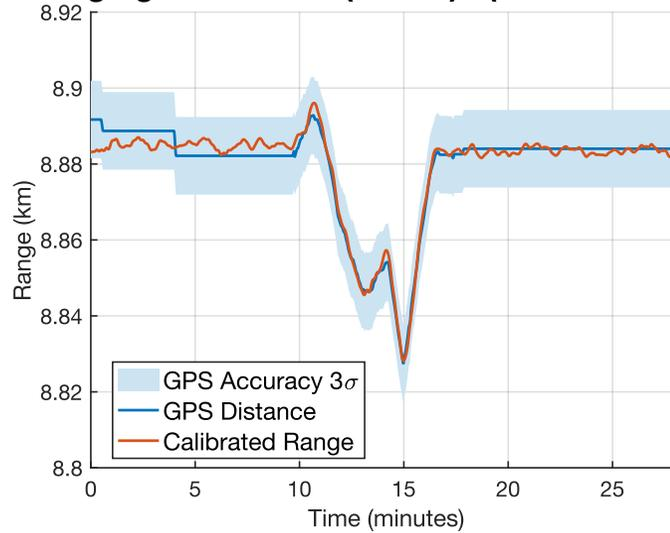
**Ranging Calibration (D to B) (RMS = 2.212m)**
