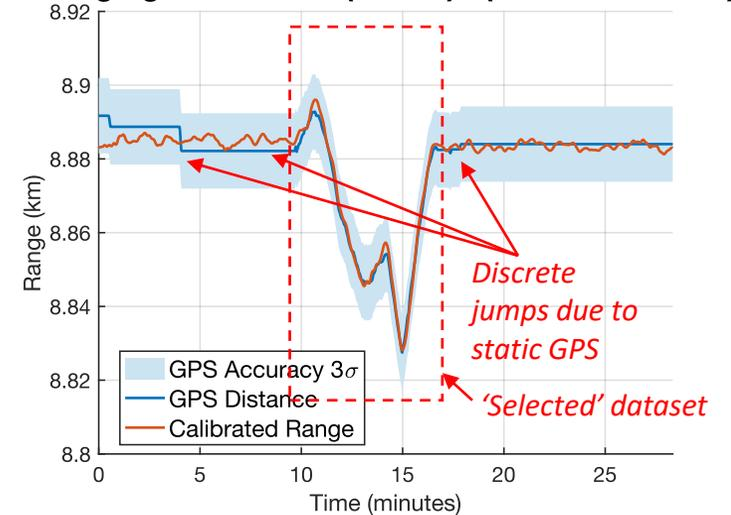
**Ranging Calibration (D to B) (RMS = 1.8458m)**
