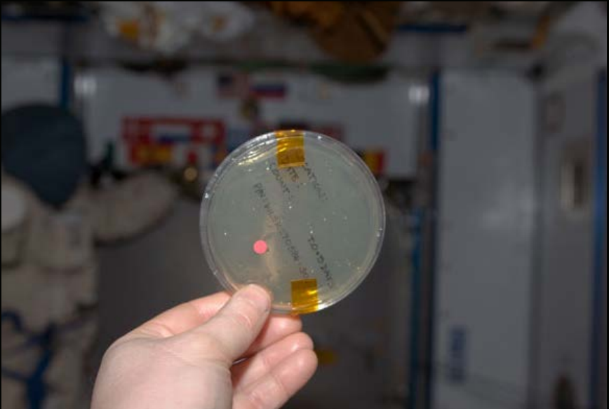
An astronaut holding a Microbial Air Sampler (MAS) Petri Dish on the ISS. The MAS is used for the collection of cabin air atmosphere for evaluation of the microbial load.
