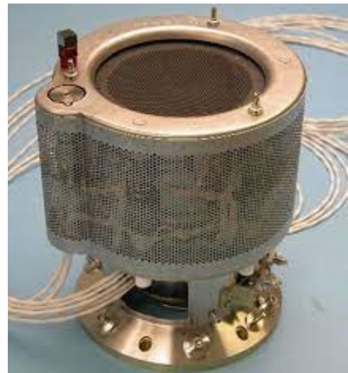
Figure 4.32: T5 gridded-ion thruster for GOCE mission. Credit: QinetiQ.
