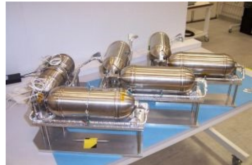
Figure 4.13: SSTL butane propulsion system. Credit: Surrey Satellite Technology, Ltd.
