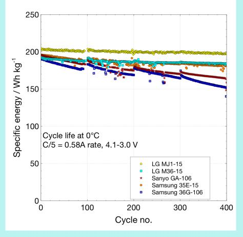
All the cells have shown high specific energy of 190 Wh/kg at 0°C, with LG Chem MJ1 cells offering the ~205 Wh/kg.
