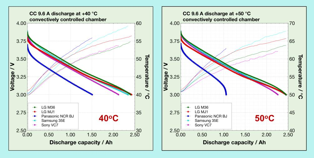
LG Chem cells provide high power densities at 20-50°C, while other chemistries provide only at warm temperatures.
