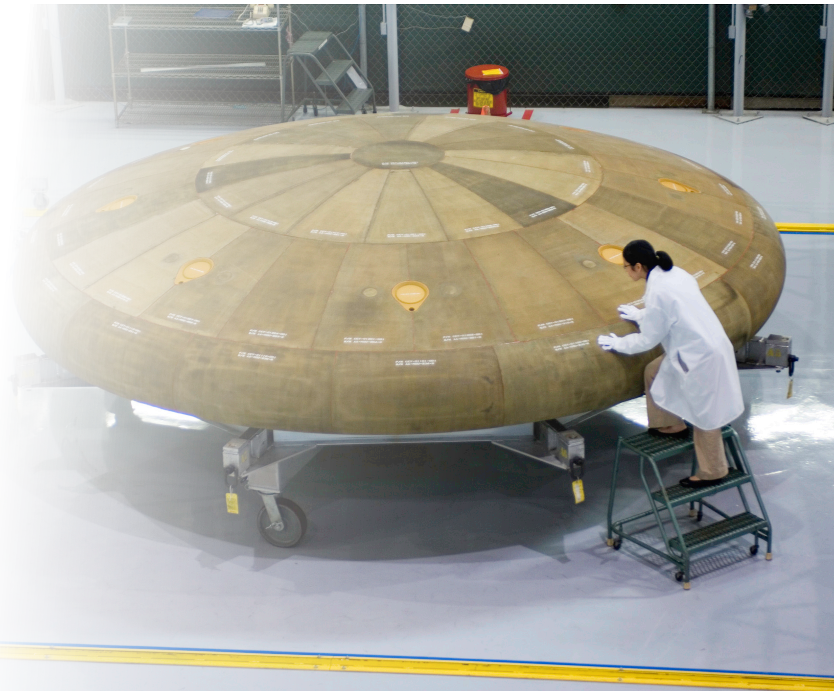
The heat shield of Orion undergoing inspection. (NASA)
