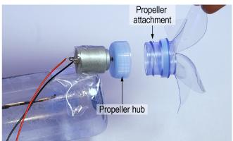
With the bottom of the bottle cap facing toward you, secure the bottle cap to the shaft of the motor.
