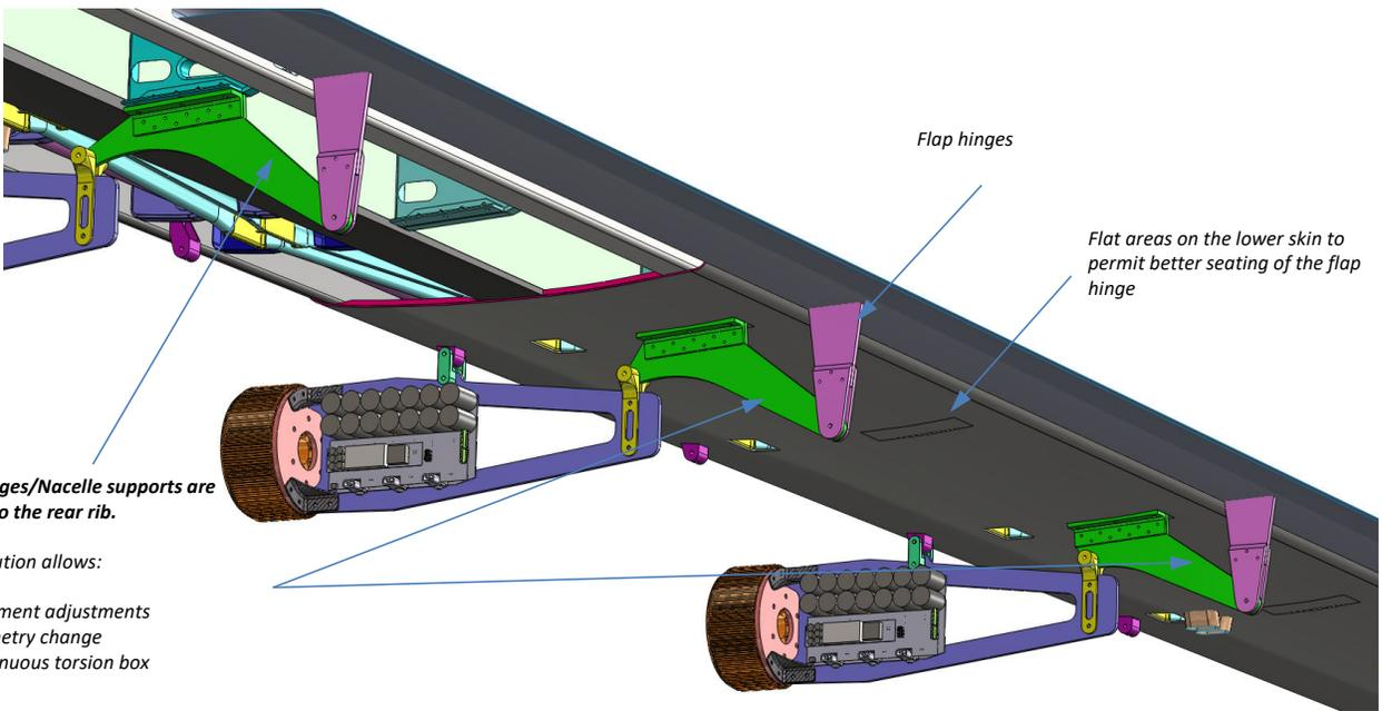
Flap hinges/Nacelle supports are bolted to the rear rib.
