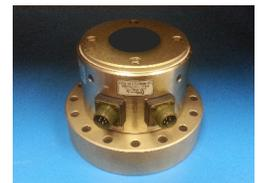
Torque/Thrust Load Cell
