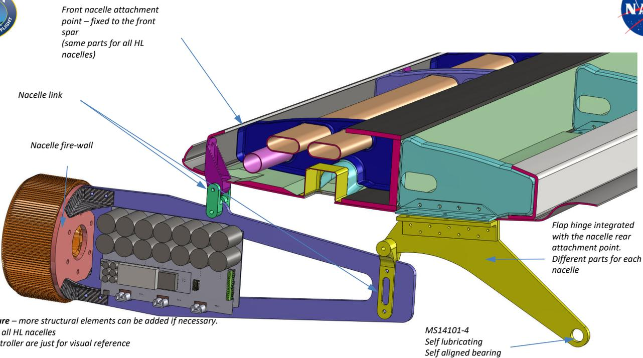
Front nacelle attachment point - fixed to the front spar (same parts for all HL nacelles)
