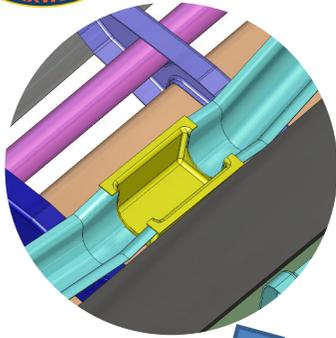
Notice the zig-zag path of the instrumentation duct in order to intercalate with the main bus duct curves that goes into the HL nacelles.
