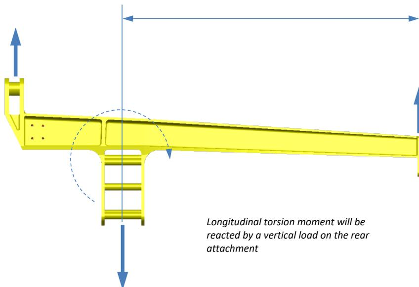
*Longitudinal torsion moment will be reacted by a vertical load on the rear attachment*
