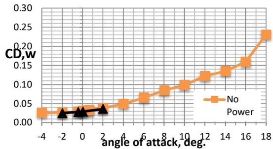
Cruise power at wing-tip results in 7.5% reduction in wing CD
