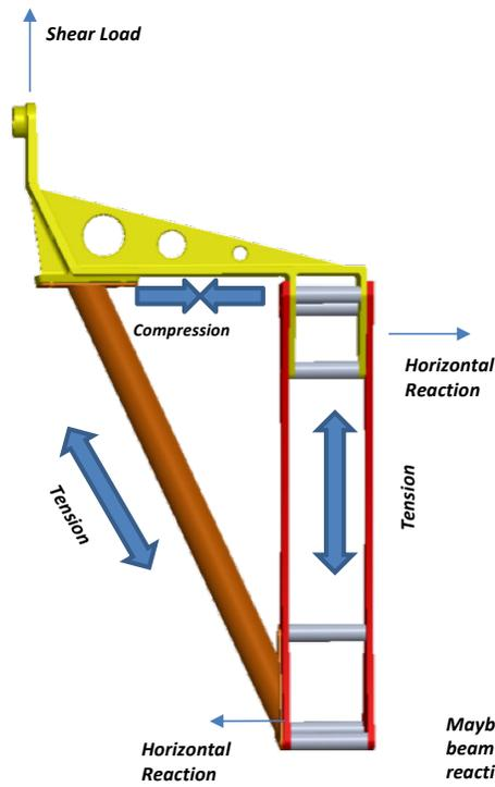
*Maybe it will be necessary to add one beam on the fuselage to carry this reaction. Further analysis will be necessary.*
