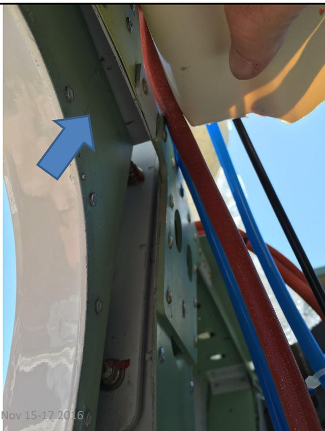
*Door frame will require too much modifications to install the tube structure proposed originally.*
