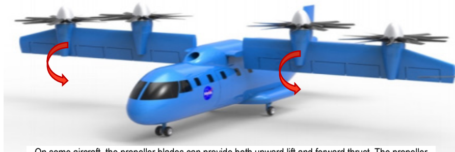
On some aircraft, the propeller blades can provide both upward lift and forward thrust. The propeller blades rotate parallel to the ground to provide upward lift for takeoff, but the propellers can then pivot 90° so the blades are rotating perpendicular to the ground to provide forward thrust.
