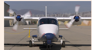
NASA's X-57 all-electric X-plane is shown here in its Mod II configuration. (NASA AFRC TV/ Steve Parcel)
