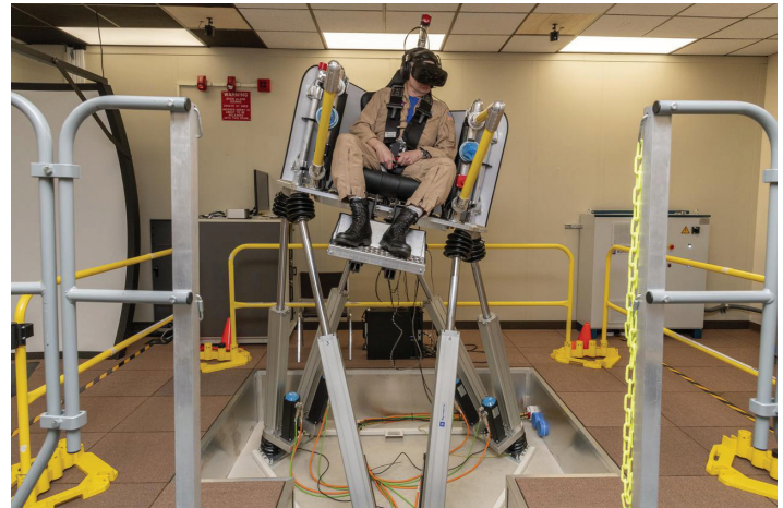
Several projects supporting NASA's Advanced Air Mobility mission are researching how to make routine flight of air taxis and drones a reality. NASA Armstrong also built a new simulator to study air taxi passenger comfort. NASA/Steve Freeman
