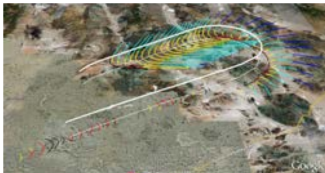
CISBoomDA software is used to integrate vehicle and environmental data with a real-time, local-area moving-map capable of displaying an aircraft's sonic boom footprint at all times and predicting effects of various maneuvers. This allows pilots to select a flight path or parameters to either avoid generating a sonic boom or to place the sonic boom in a specific location.
