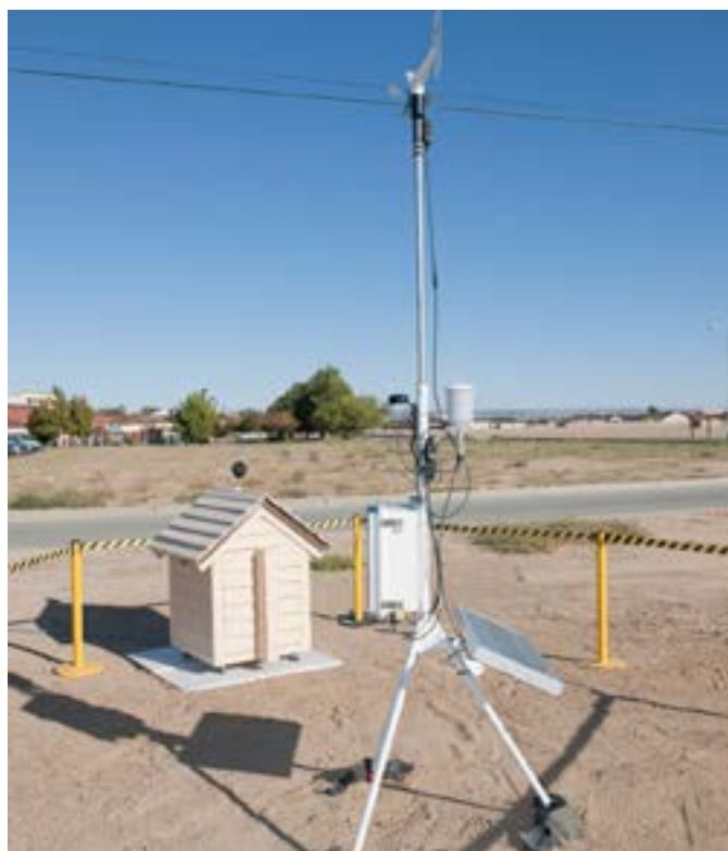
One of the instruments used for the WSPR project is the SNOOPI sonic boom recorder, short for Supersonic Notification of Overpressure Instrumentation, mounted inside a commercial doghouse. SNOOPI records local sonic booms by date, time and intensity, 24-hours a day, seven days a week.
