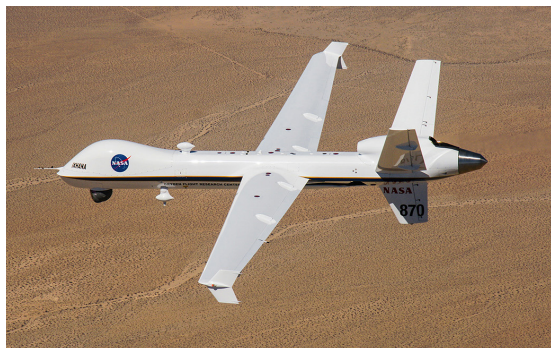
NASA's Ikhana Predator B received an avionics upgrade, wingtip winglets and a new paint scheme in 2013. GA-ASI Photo
