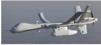
With a high-tech infrared imaging sensor in its underbelly pod, the Altair UAS flew repeated passes over the Esperanza wildfire to aid firefighting efforts in October 2006. (GA-ASI photo)
