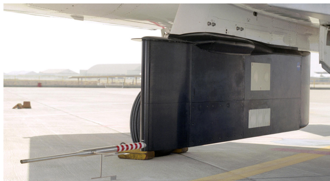
Two panels of Space Shuttle TPS insulation were mounted on the flight test fixture underneath NASA's F-15B during the Lifting Foam Trajectory flight test series in 2005. (NASA / Jim Ross)
