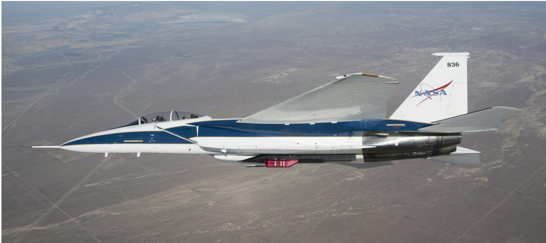
The Eagle Aero probes fly attached to the red device underneath NASA's F-15B research test bed aircraft during a test flight in early 2011. (NASA / Carla Thomas)
