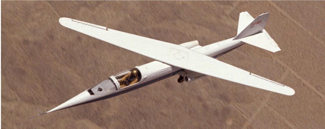
AD-1 in flight at 60 degree wing sweep (NASA photo ECN-15846)
