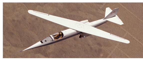
AD-1 in flight at 60 degree wing sweep (NASA photo ECN-15846)
