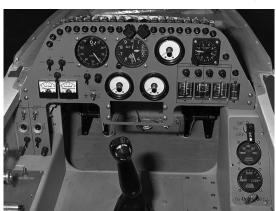
AD-1 cockpit and intrument panel (NASA photo E-36067)
