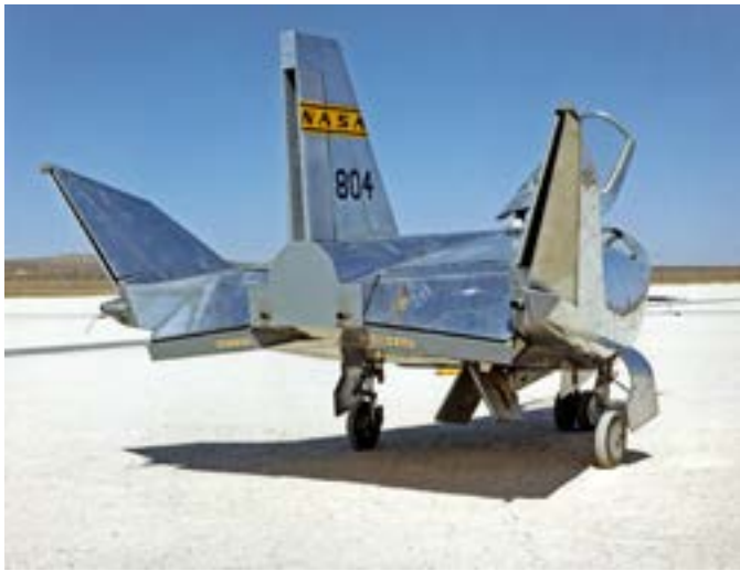
HL-10 is shown on Rogers Dry Lake in 1966 with its subsonic control surface configuration. (NASA Photo)
