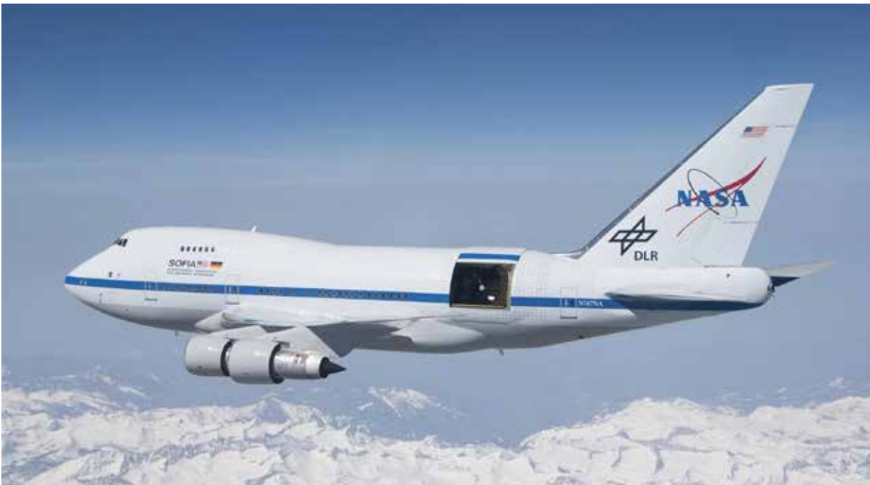
SOFIA soars over the snow-covered Sierra Nevada mountains with its telescope door open during a test flight. SOFIA is a modified Boeing 747SP aircraft. Credit: NASA/Jim Ross
