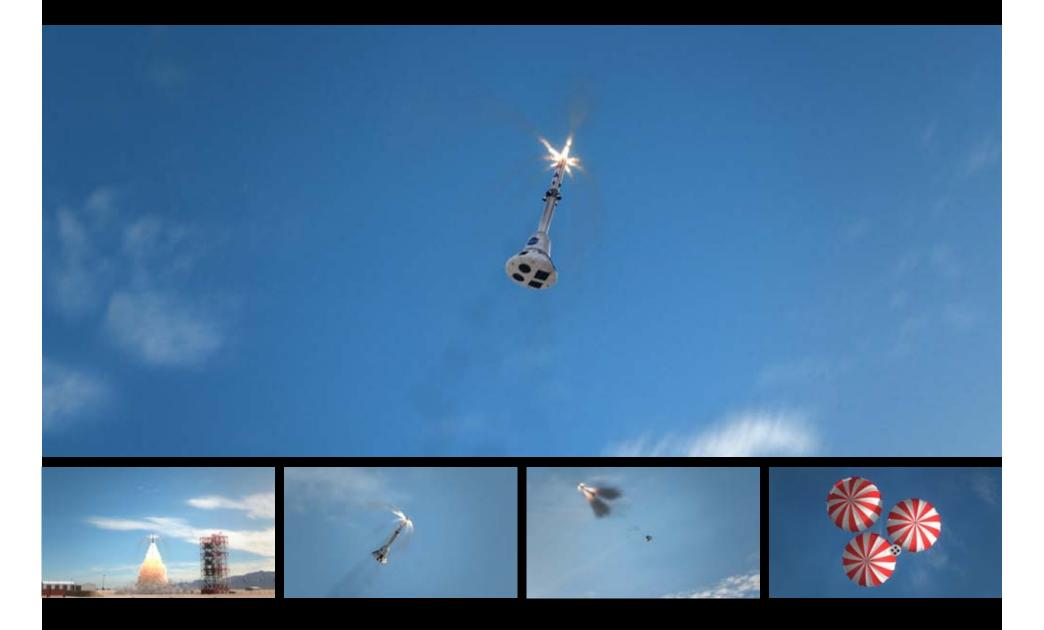
Pad Abort-1 is a NASA flight test of a system that could be used to rescue a crew and its spacecraft in case of emergencies at the launch pad.
